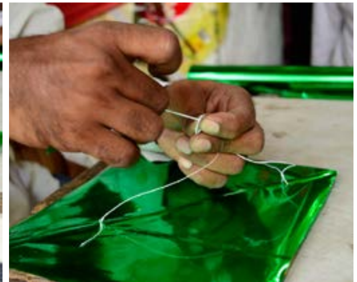
12. When the length of the loop is satisfactory a knot is made at that position.
