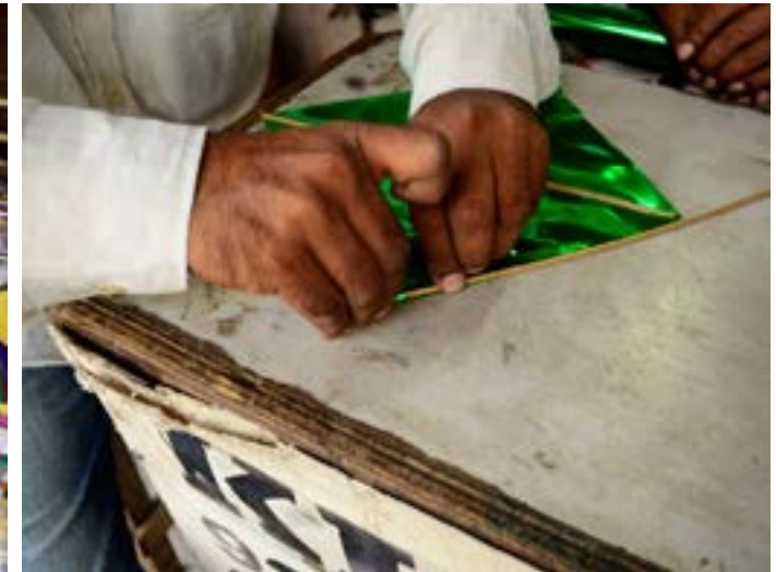
16a. The ends of this semi circular stick are stuck to the rhombus shaped paper as seen.
