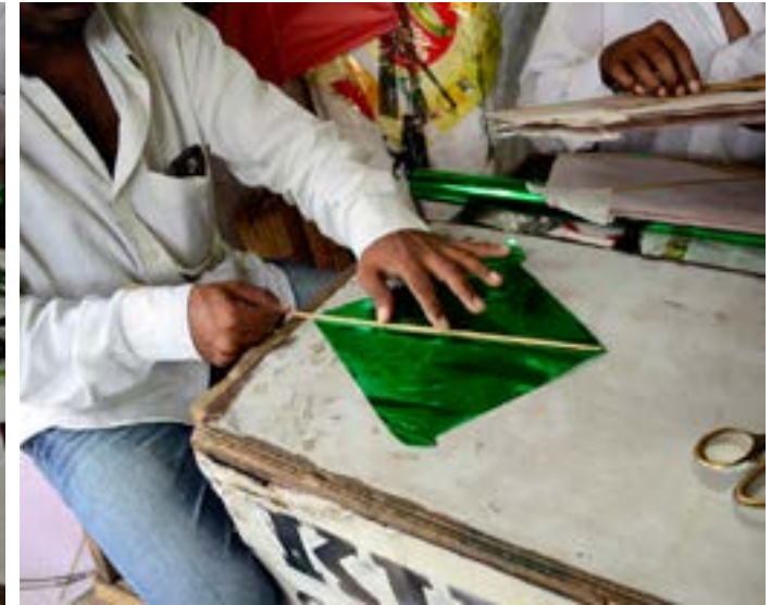
8. A bamboo stick is placed like a diagonal and the size is checked.
