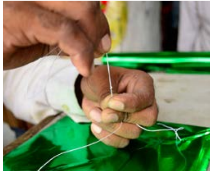
13. A double knot is made to ensure the length of the thread does not change.
