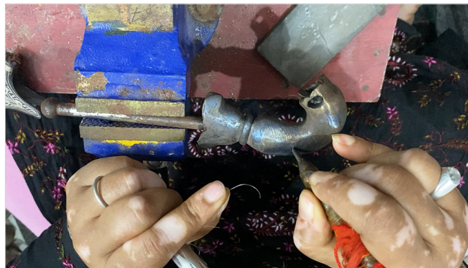
Iron pen and metal wire is used for inlay work.
