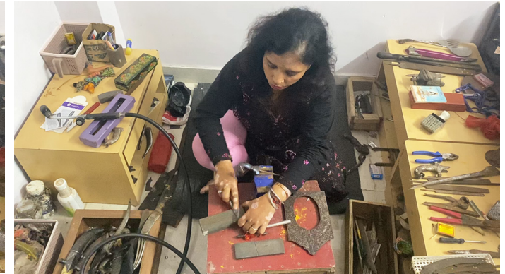
Iron Chirani is sharpened before carving.
