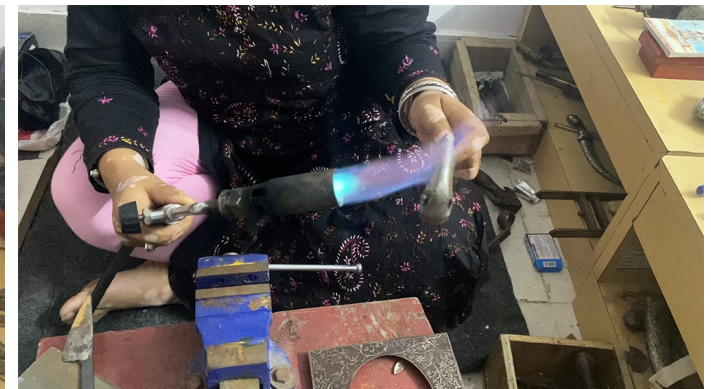
A handle is heated till its colour get changed.
