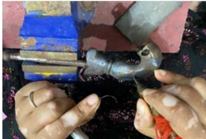
Iron pen and metal wire is used for inlay work.
