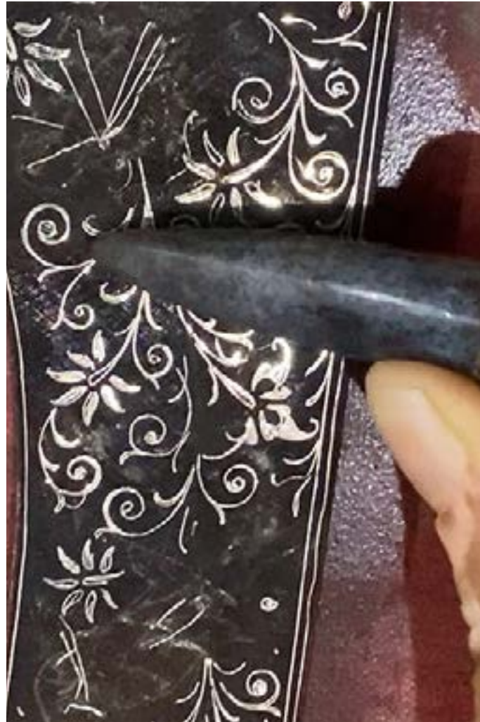
Upni is used to give the proper shape to the design using metal wire inlay work.
