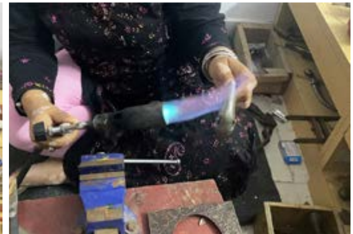
A handle is heated till its colour get changed.
