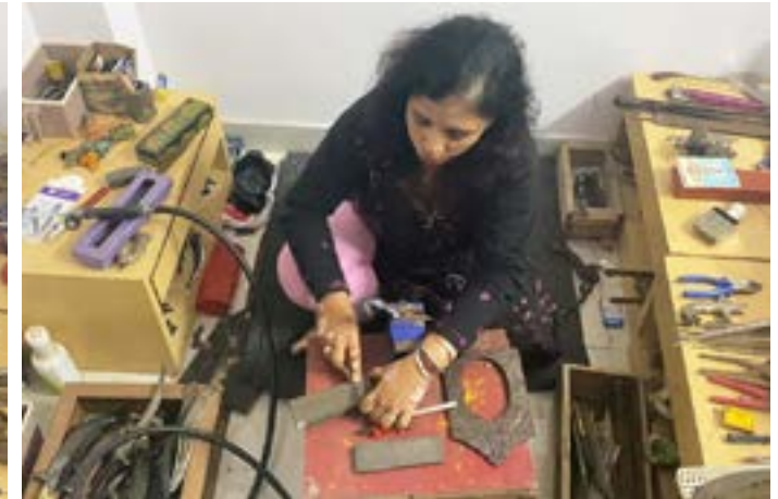
Iron Chirani is sharpened before carving.
