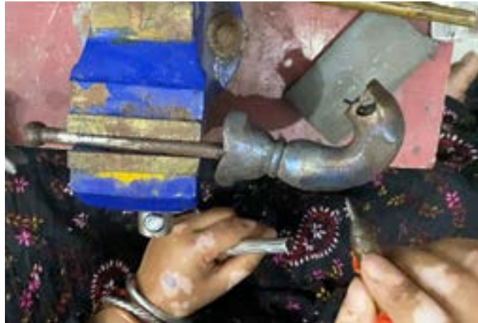
The colour of the handle is changed after heating.
