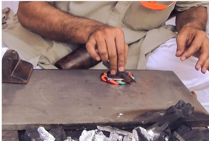
Artisan is placing heated aluminum bangle on the lac bangle.
