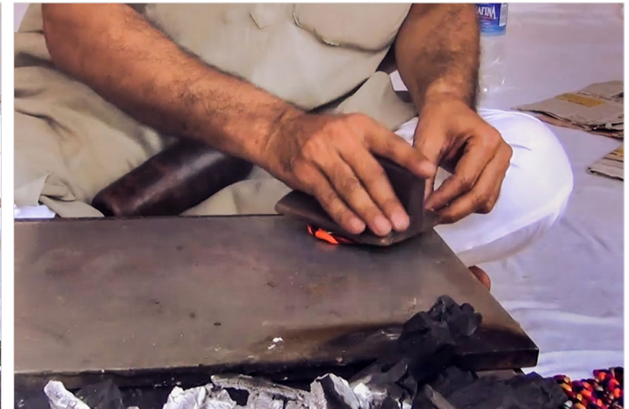
Artisan is pressing the lac bangle with a flat wooden tool to push the aluminum bangle inside.
