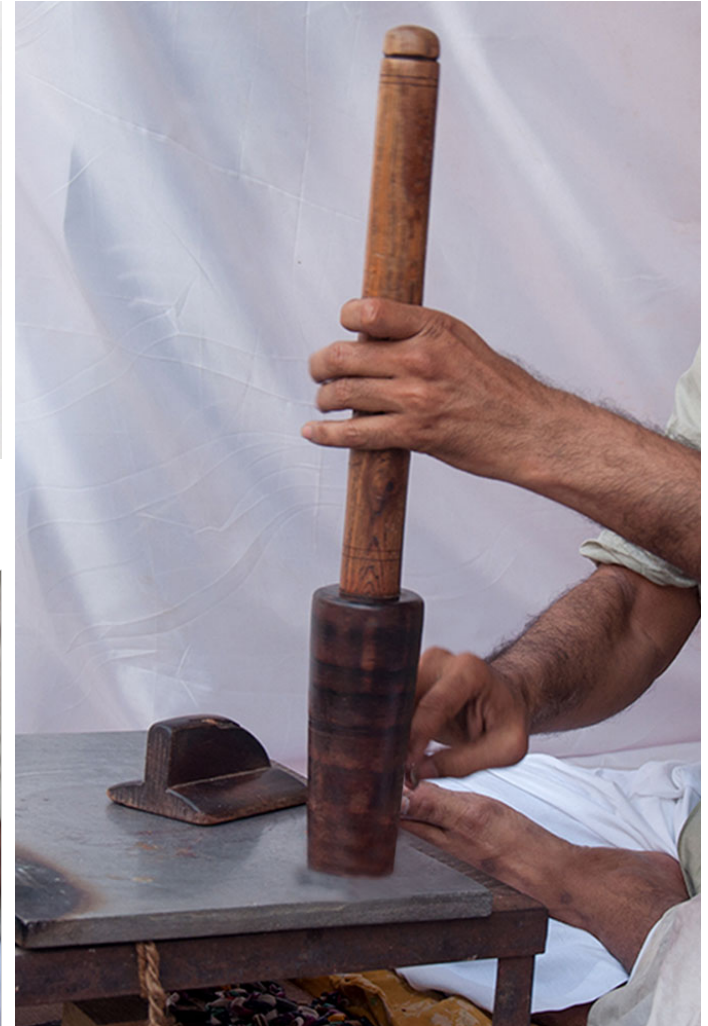
A flat wooden tool is used to press the lac bangle after heating, and a wooden round beam is used to mend the
