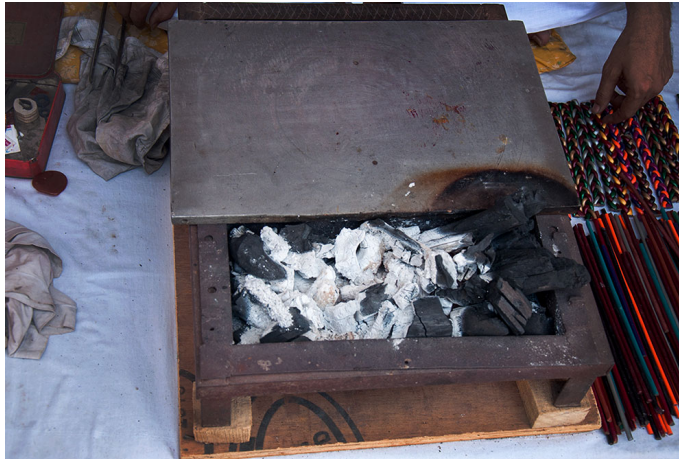
A coal burner is used to heat the lac to make it flexible for shaping.
