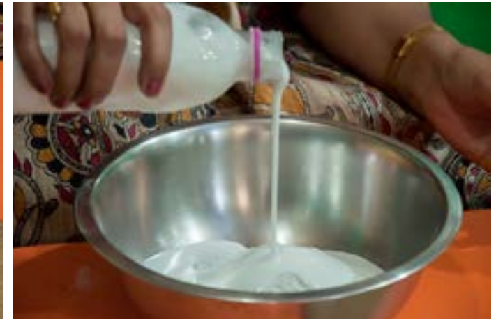
Synthetic Adhesive being mixed with ceramic powder.
