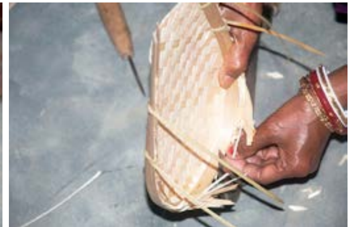
A chisel is used to tuck the extra strips.
