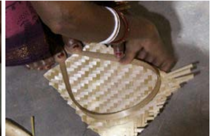
Artisan bends and arrange the bamboo strip in the required manner.
