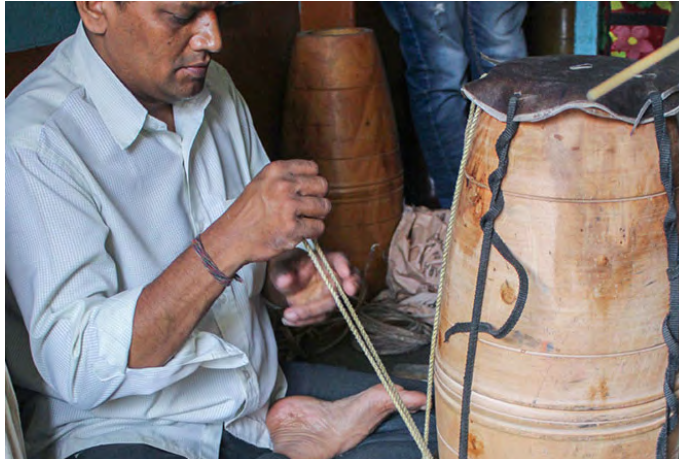
The rope is passed through the iron frame.
