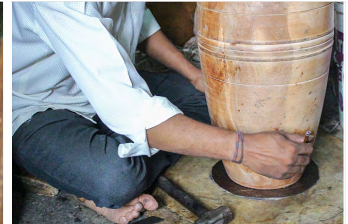
Resonator is placed on leather for marking the required size.
