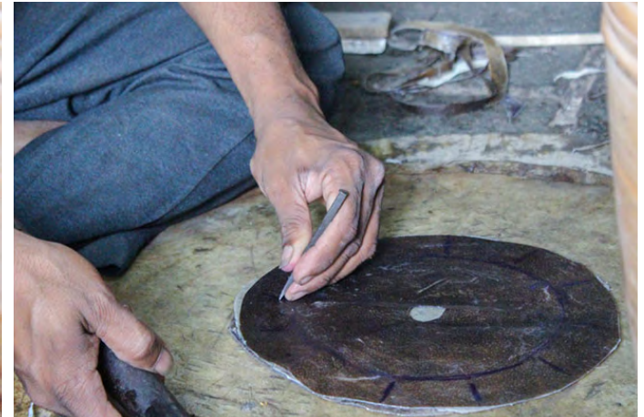
Holes are made on the leather to tie nylon strip.
