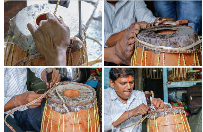
Leather straps is woven to make a circular grip.
