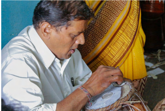
Slaked lime (chunna) is applied on the right side of mridangam.
