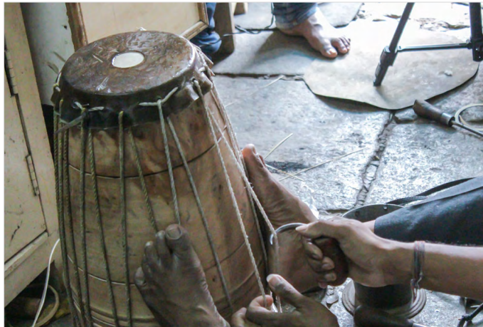
Rope is tighten using a hook.
