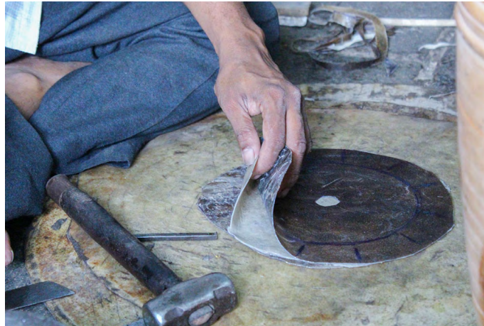
Three layers Buffalo, Goat and Buffalo calf leather is used to make the right side of the mridangam.
