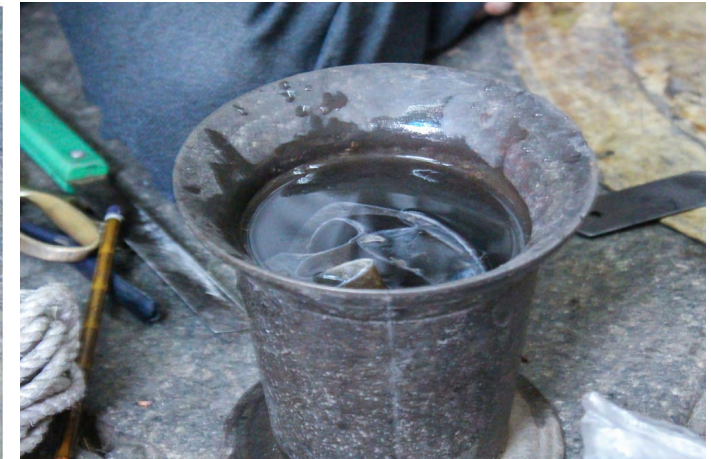
Leather is soaked into water to make it soft.
