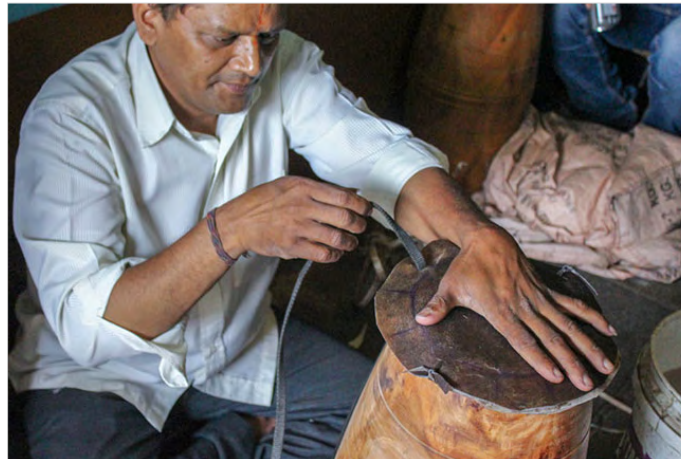
Nylon strip is used to hold the leather in place on both sides.
