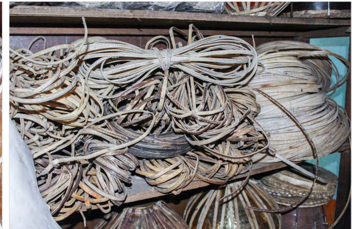
Strips of leather after treatment done using slaked lime (chunna).
