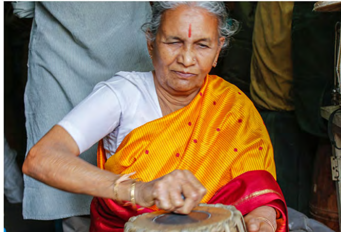
The karne (black patch) is leveled layer by layer using a stone.
