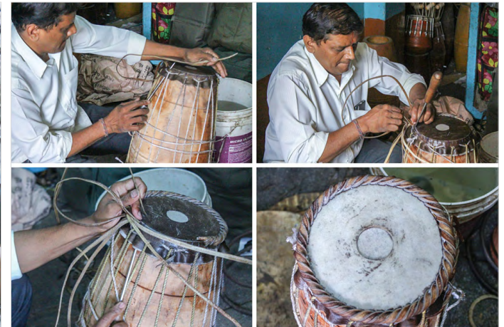
Using leather strips, circular grip is woven around leather.
