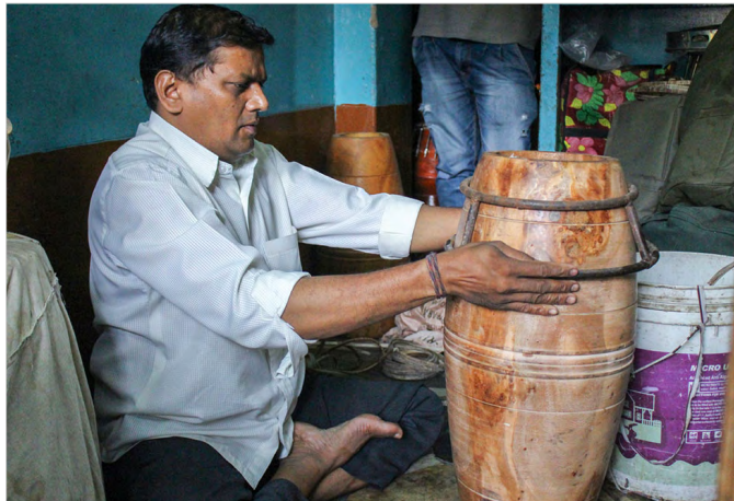
Iron frame of circular shape is placed on wood resonator to support the leather straps.
