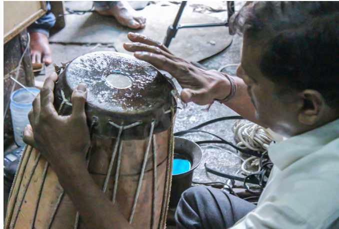
Water is applied frequently to soften the leather.
