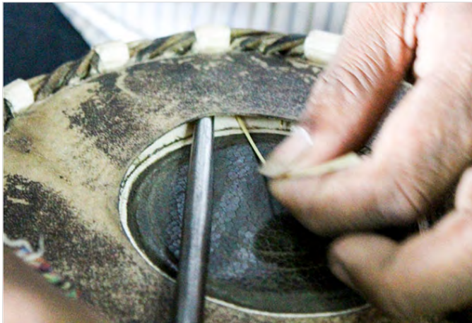
Small stick is placed inside a layer of leather to produce good sound.
