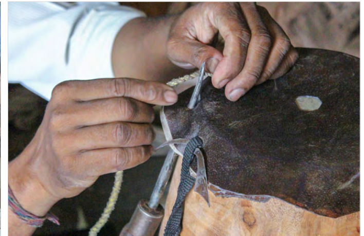
Small holes are made and rope is inserted to hold the leather in place.
