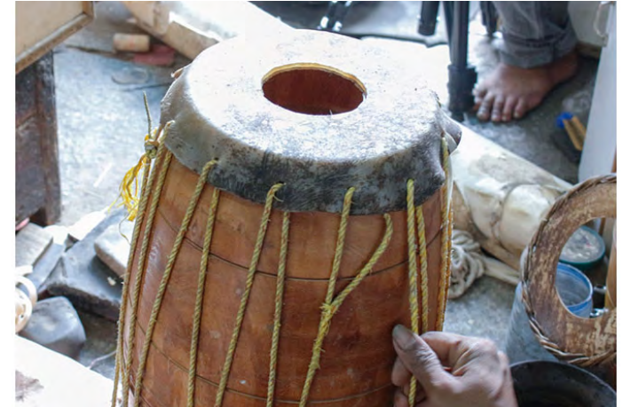
Two layers of buffalo Leather with a big hole is tied to the left side of resonator using rope.
