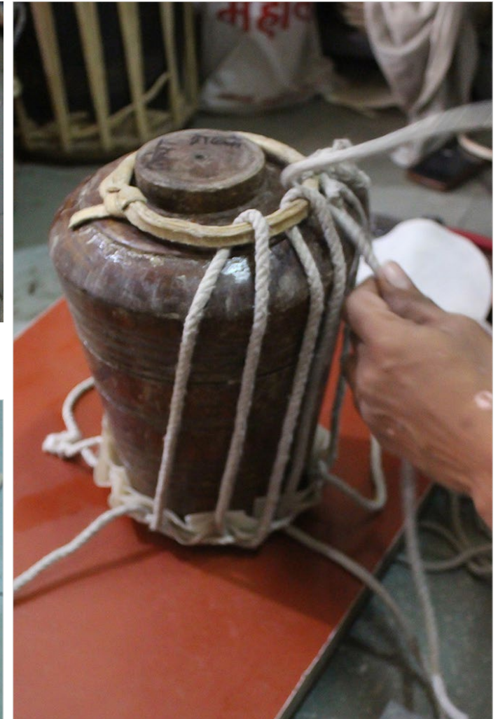
A rope is passed through the leather sheet and the leather belt.
