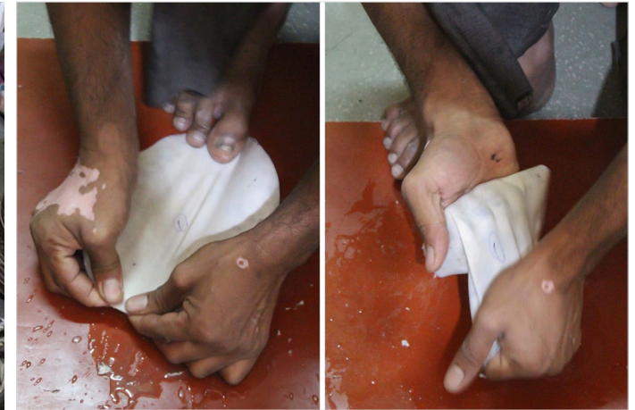
The hide/leather stretched from all the directions for uniform expansion.
