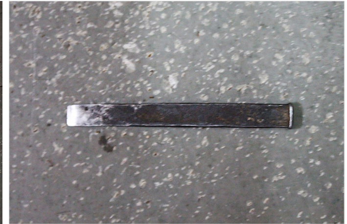
Chisel was used for making small slits for leather straps to pass.
