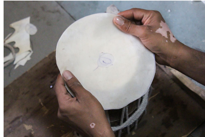
A small circular shape is cut in the center of the leather.
