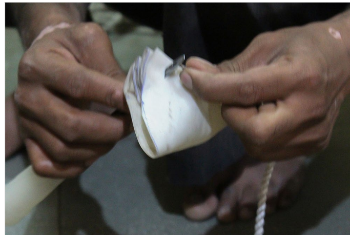
The rope is passed through each hole using a plug insertion needle.
