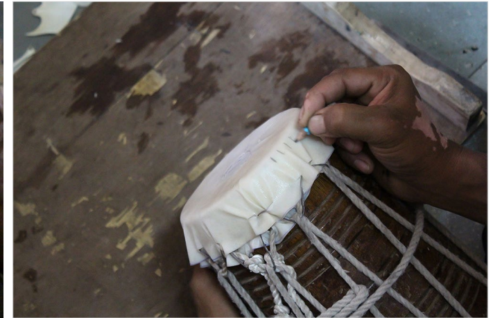
Markings being done on the rim of the drum with a pencil.
