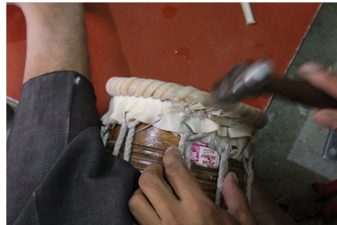
These strap ends are then hammered to avoid unknotting.
