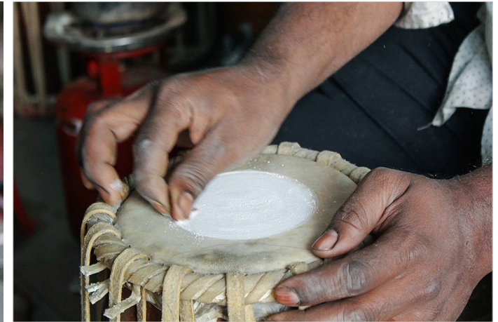
The surface of the leather is then scrubbed with a chalk piece.
