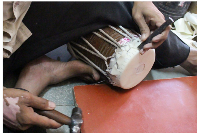
Small slits being made on the marked areas with a chisel and hammer.
