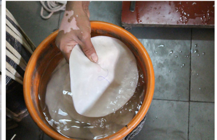
The leather soaked in water for flexibility purposes.
