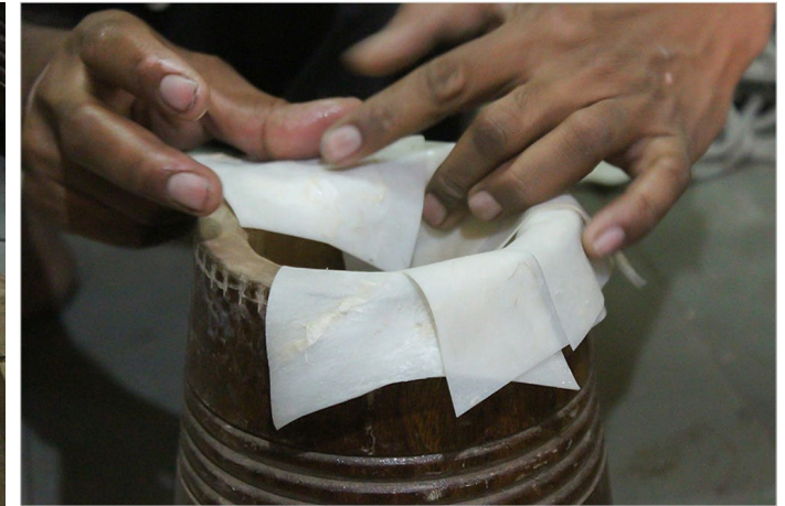
Previously made random leather shapes being folded and placed over the head of the drum.
