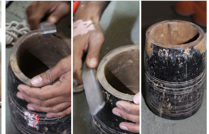
The wooden drum being leveled manually with a chisel.
