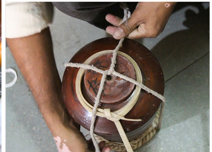
A strap of leather is tied under the drum as a belt.
