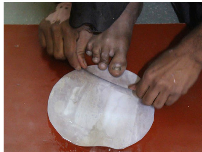
Soaked leather is placed on a board and scored with a metal ruler.
