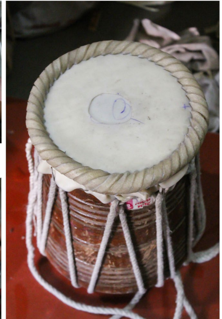
The semi-finished instrument is then left for drying and shrinking of leather.
