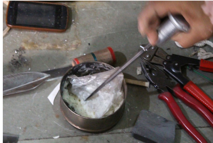
A plug insertion needle is greased with animal fats for smooth working.
