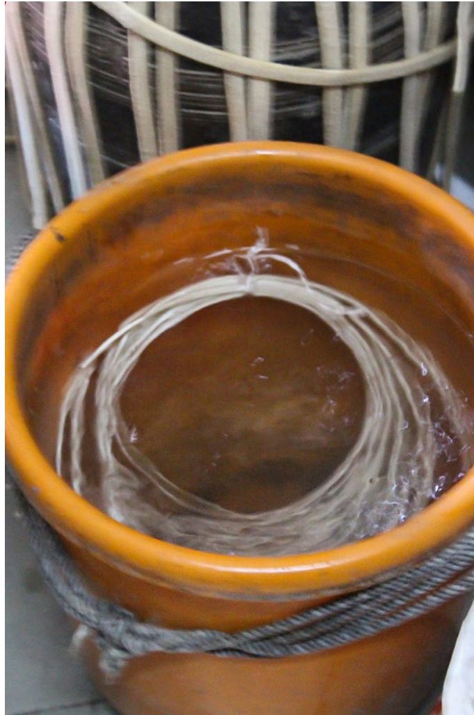
Straps being soaked in water.
