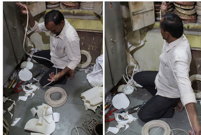
Leather straps being measured to suit the size of the drum.
