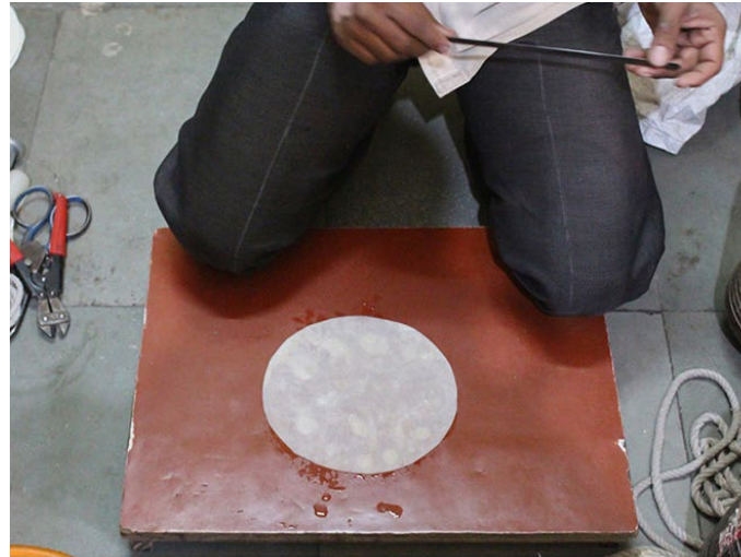
The hide/leather stretched from all the directions for uniform expansion.
