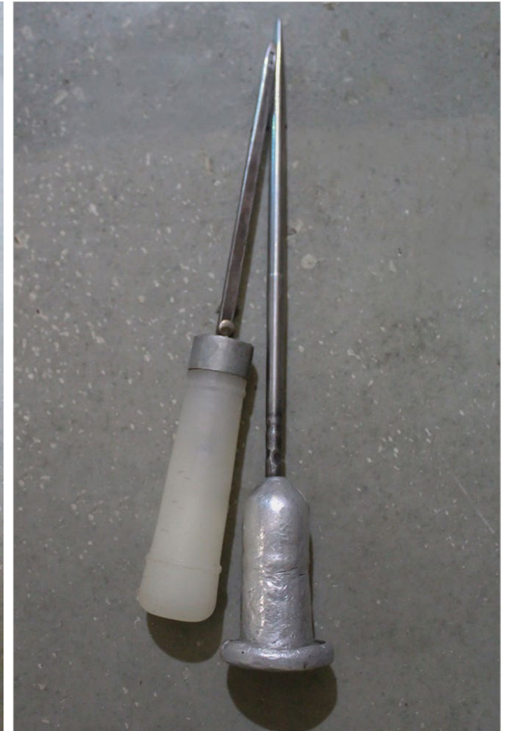
Plug insertion needles used for making rope and leather straps through the slits made.
