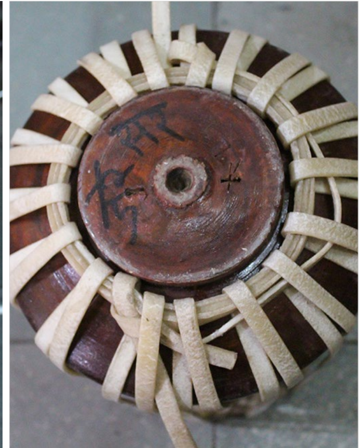
Leather straps are interwoven to attain tight tension.
