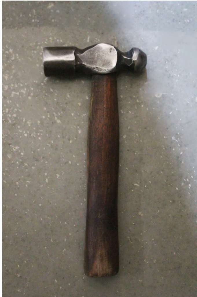
A ball-peen hammer is used for tapping and delivering blows for fine-tuning of the instrument.
