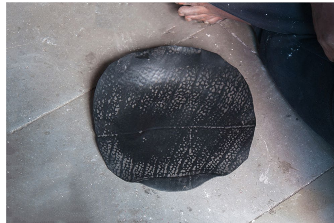
Flat rubber sheet, used for mixing wheat paste and the iron filings.
