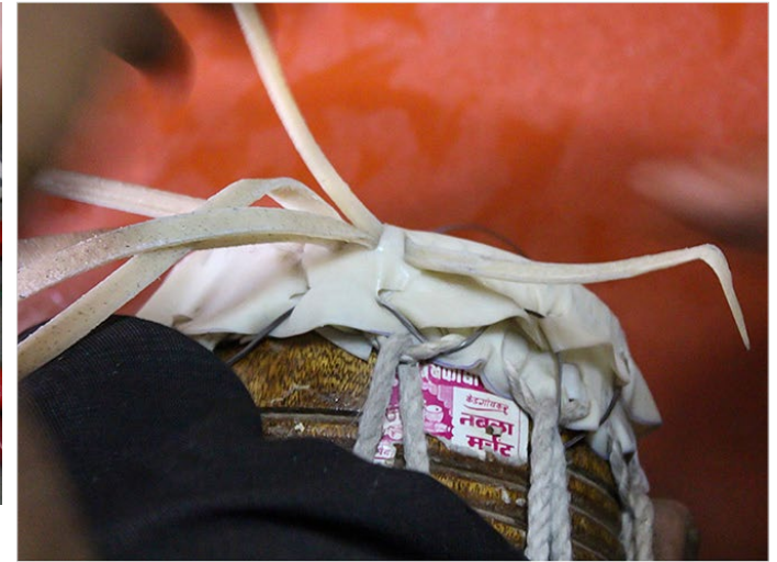
A plug insertion needle is greased with animal fats for smooth working.
