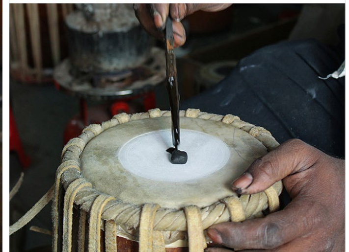
A pinch of wheat paste and glue is added to the top of the 'maidan' layer of the tabla.
