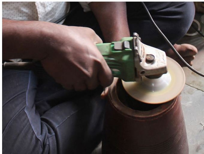
One side of the wooden drum being leveled using an angle grinder.
