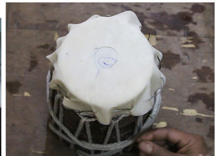
A string is passed through each hole manually with fingers and tied with rope.
