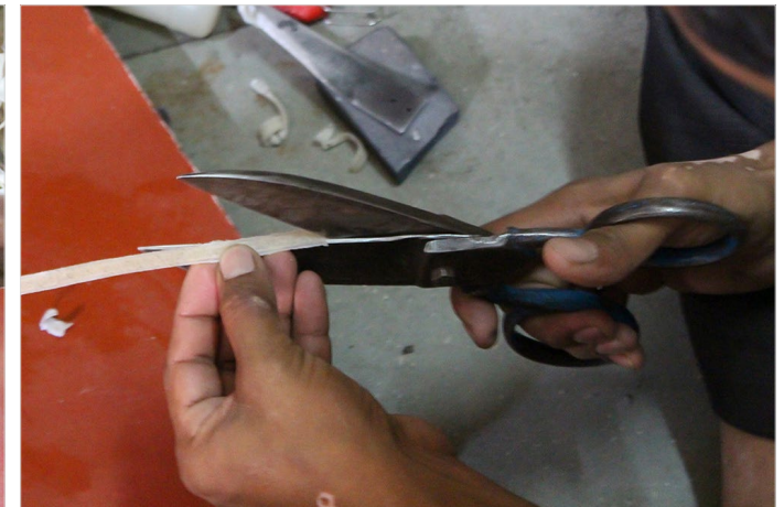
The leather strap is cut diagonally with a pair of scissors for easy insertion.
