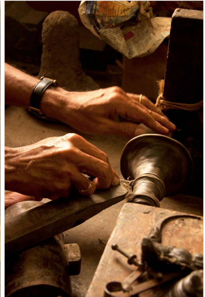
The artisan constantly keeps his leg in touch with the support system ( i.e. mallet and a wooden piece kept under his hand ) under the Lathe to get fine finishing on the wax model.
