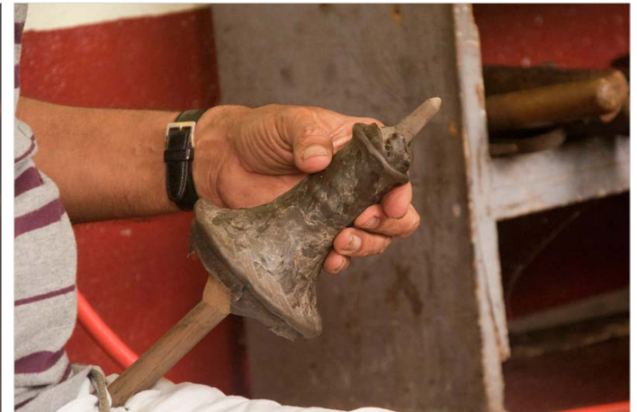
Roughly shaped wax model of a product.
