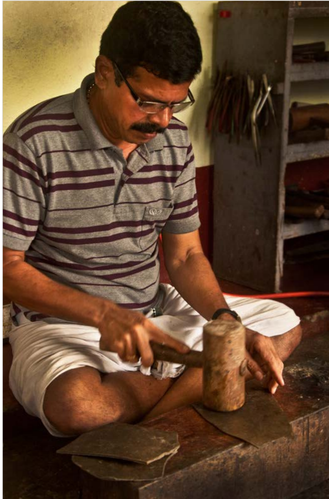
Beating with wooden mallet flattens wax sheet.
