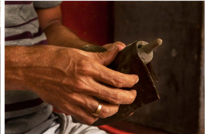
Warmed wax is coated around the finished clay model.
