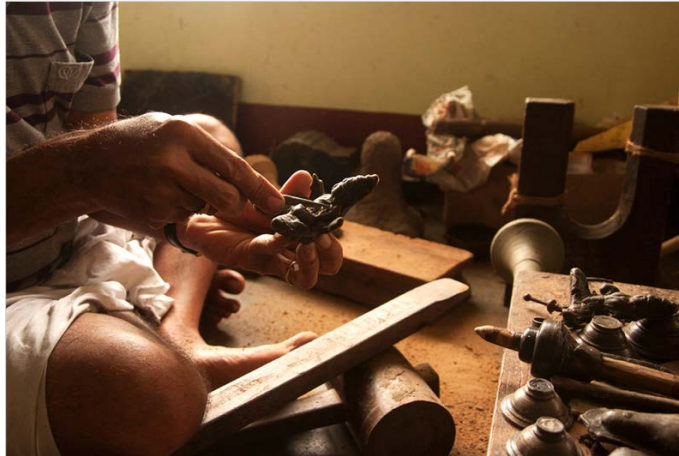
Artisan uses a flat edged tool to remove the excess wax.
