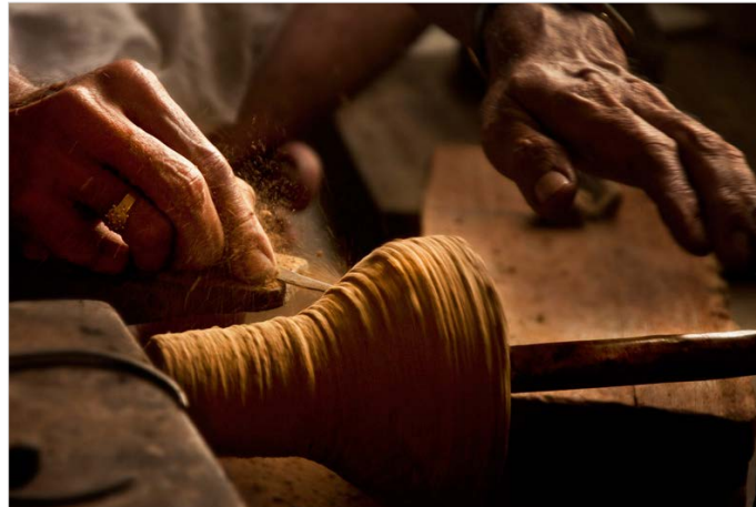
Rough base clay model is being turned for shaping.
