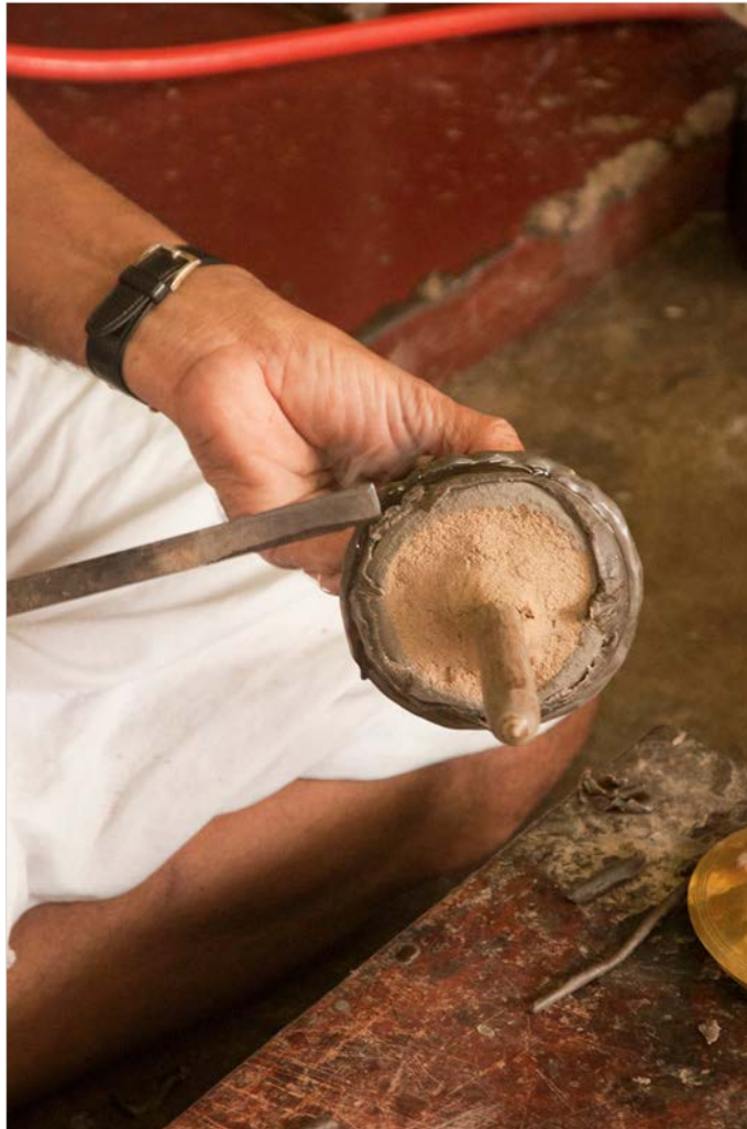
The Artisan melts wax to fill up small gaps or openings.
