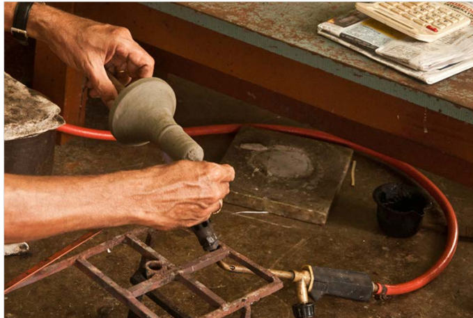
The clay mould is heated before applying the wax.
