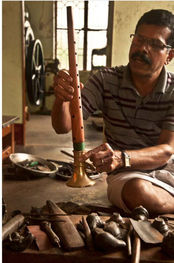
The upper part of Naadaswaram is wood and it is fixed with brass metal end piece.
