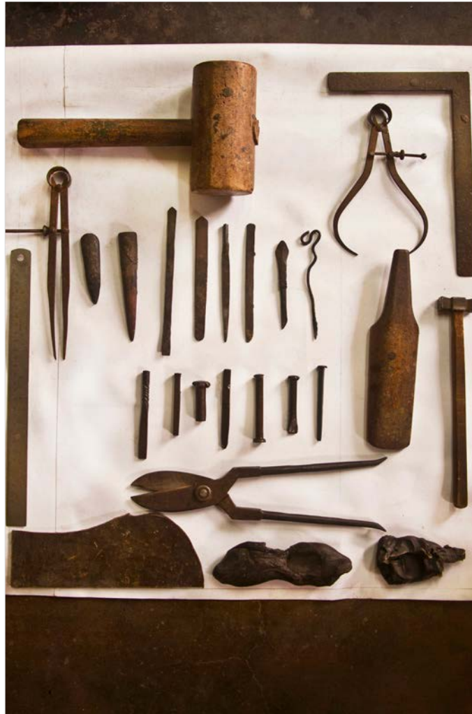
Compass, wooden mallet and other varieties of carving and casting tools.
