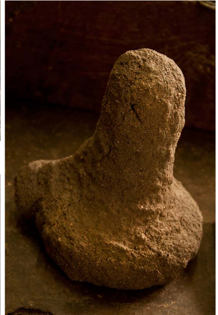
Clay coated wax model is melted and metal is poured inside to take shape of model.
