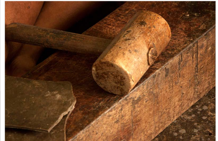
Wooden Mallets are used for flattening the wax pieces.
