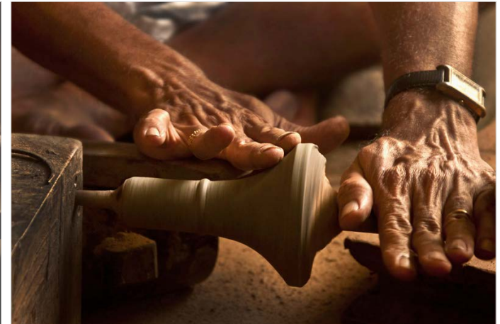
The surface of the clay model is being smoothened before coating wax.
