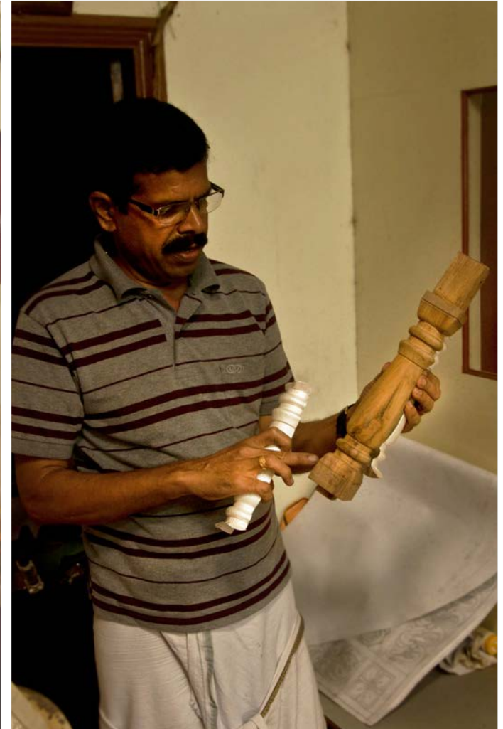
Carved wood model is used as a base for sheet metal embossing.
