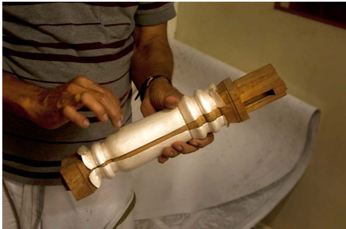
The sheet is placed in the wood model to emboss the designs.
