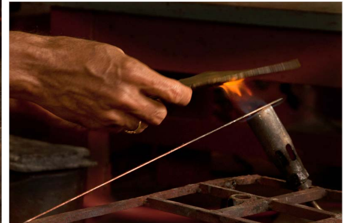
Wax is slightly warmed to make it soft for easy application.
