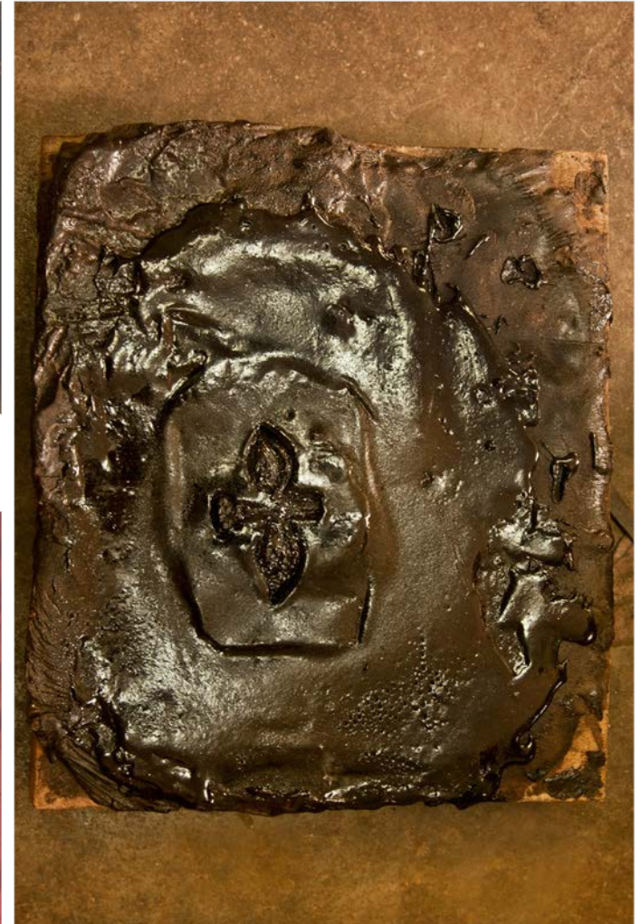
Lacquer / Wax board used while engraving the designs on the sheet metal products.
