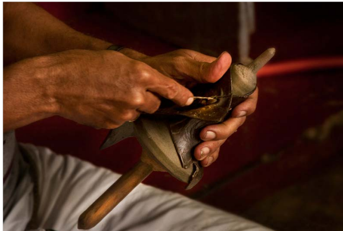
The excess wax is cut and removed.
