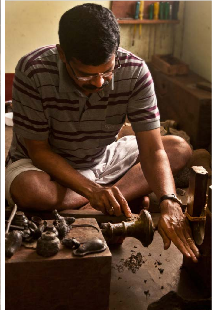
Turning process helps in creating accurate sharp and curved edges of Naadaswaram.
