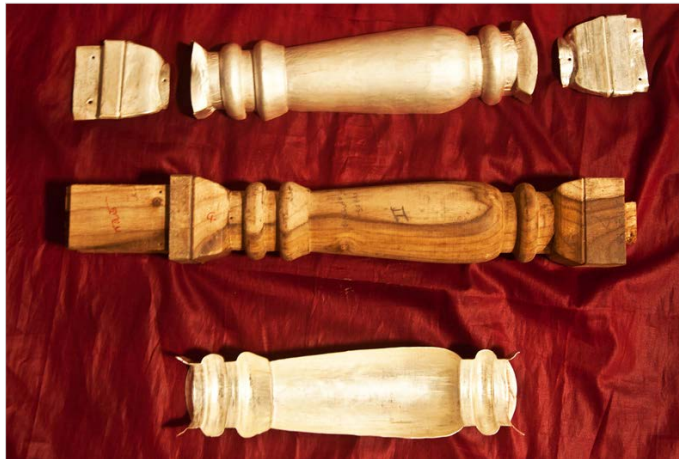
Wood model is used for making sheet metal products.
