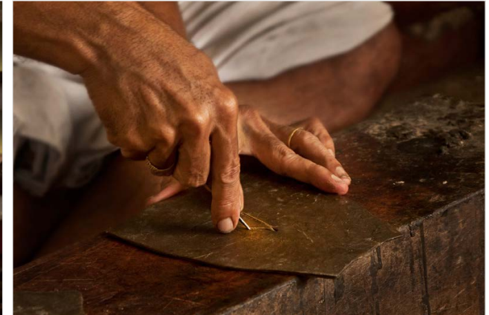
The sheet is cut according to the design to fit it on the mould.
