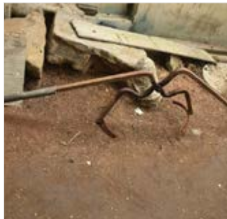
Prongs used to hold the mould.
