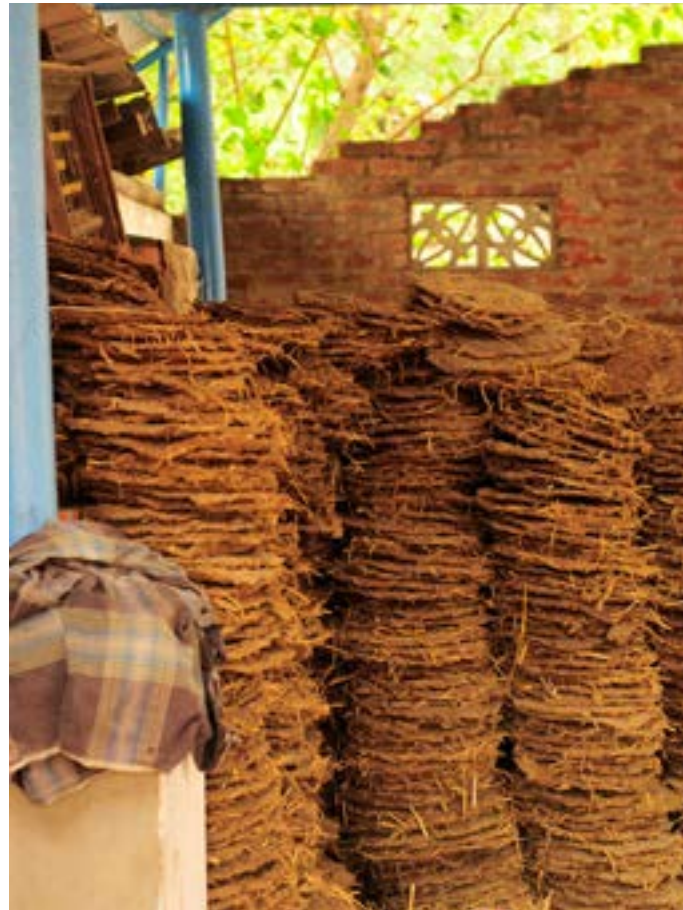
Fuel for heating the mould to remove wax.
