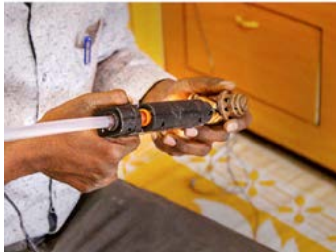
Using a lantern burner, the artisan making the head part of the bird.
