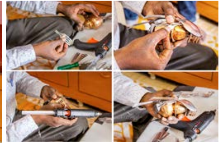
Artisan using fork heads to make the wings part of the bird.
