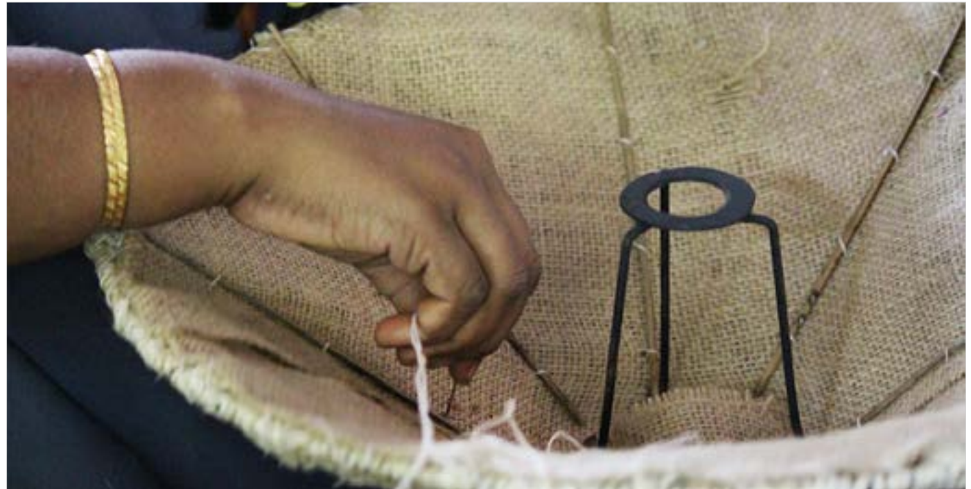
The gunny cloth and sticks are stitch at the back side of the lamp with the help of needle and thread.
