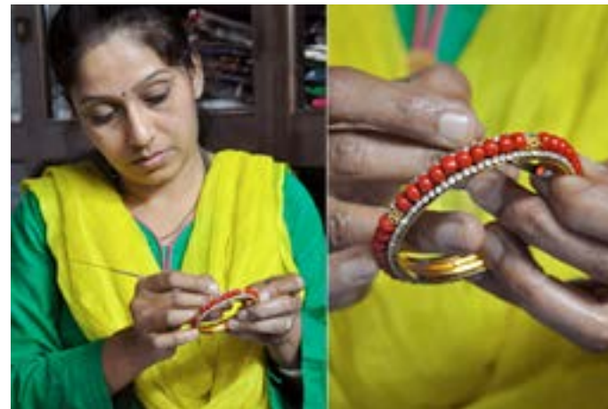
Artisan heats the edge of nylon thread using incense stick for making extra thread invisible.
