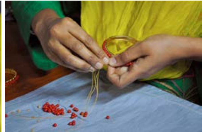
For fixing the beads to the bangle, the artisan puts several knots using nylon thread.
