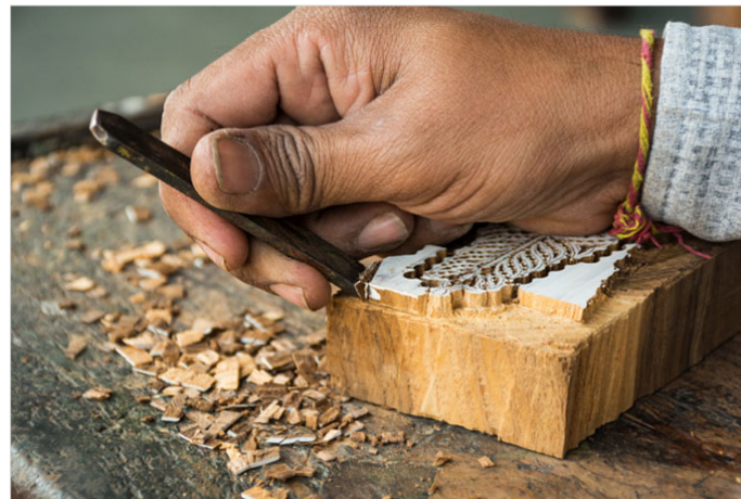
Gliding Motion: The artisan rests the Farsi on the angled face and hammers out the thin wafers of wood created from the chipping.
