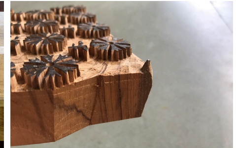
The projection on the corner is a repeat point made with a blunted nail with the wood around it carved in order to support it
