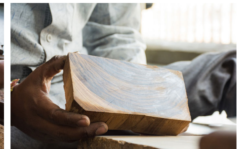
A leveled and polished block ready for the next step in the process, that is, etching.
