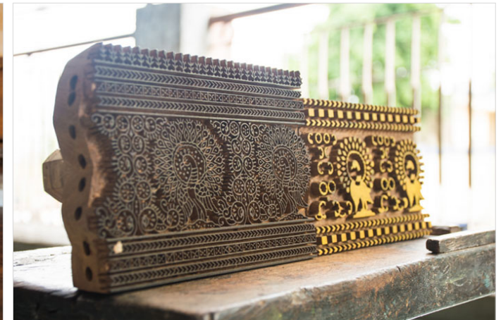
A Rekh (outline) and its corresponding Dattla (filler) block.
