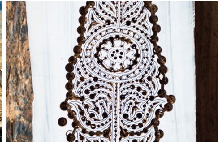
A block with the holes connected and the inner corners cleared with a sharp Nakhya.
