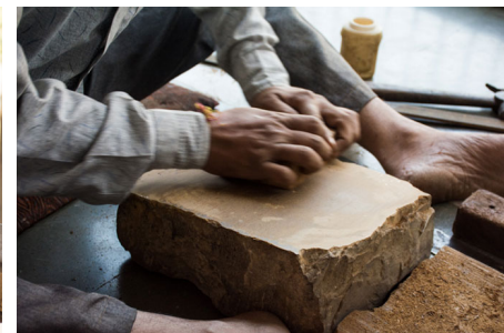
Polishing the leveled block on a river stone.
