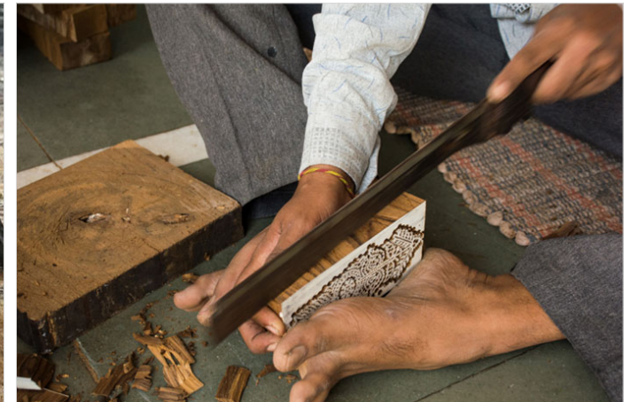
Marking the depth of the block with a saw, an important step.
