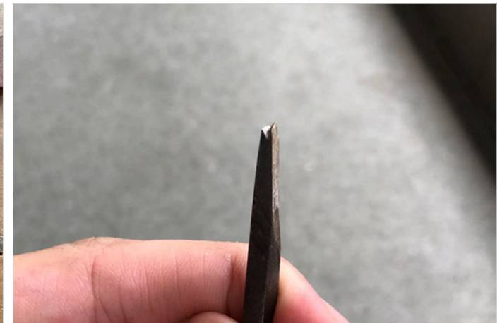
A Nakhya: The V-shaped end tapering into a sharp point allows the craftsmen to get into the corners and sharpen their appearance.
