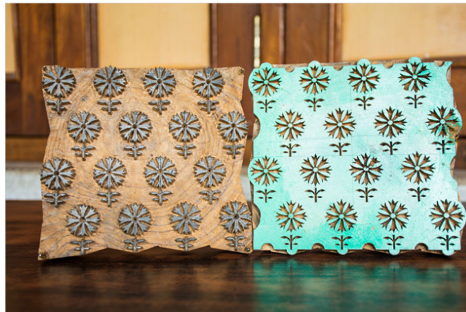
A Rekh (outline) and its corresponding Gad (background) block.
