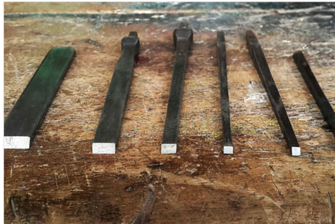
Farsis used for the chipping of excess wood.
