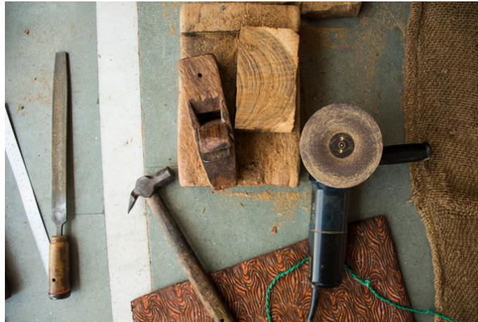
Leveling tools such as Randha, hand files, and sanding machine.
