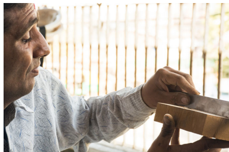
Artisans must check the uniformity of the surface after every round of filing and leveling, done usually with a thick steel scale.
