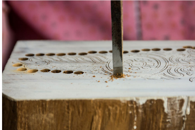
Holes being drilled along the edges of the design.
