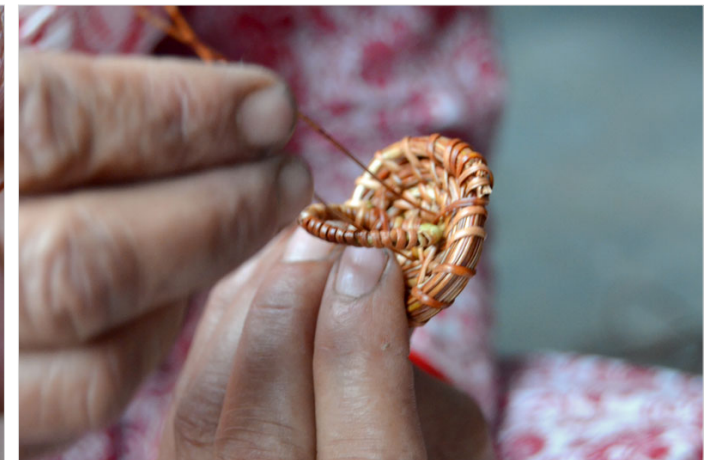
Single needle coil being attached to a multiple needle coil to make a ring
