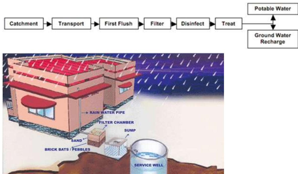
Fig. 10 Rainwater Harvesting at individual level
