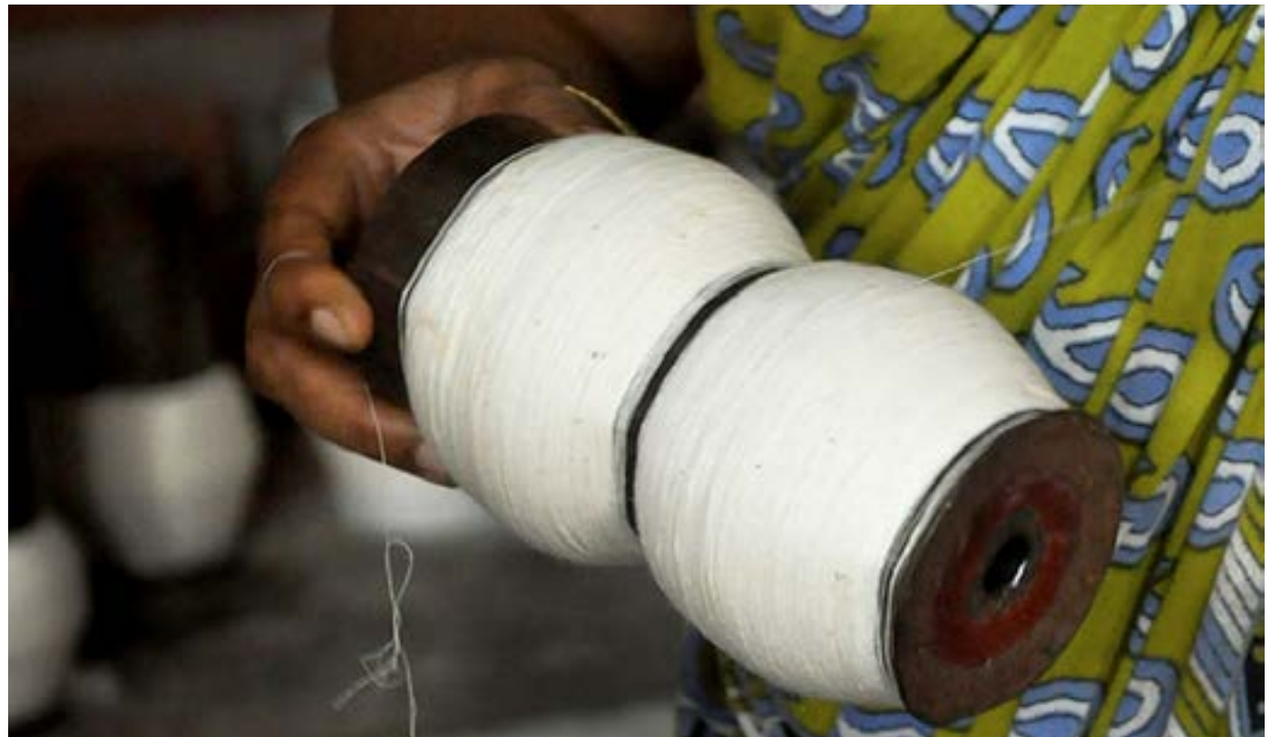
Cotton bobbin cones are sent to the warping machine.
