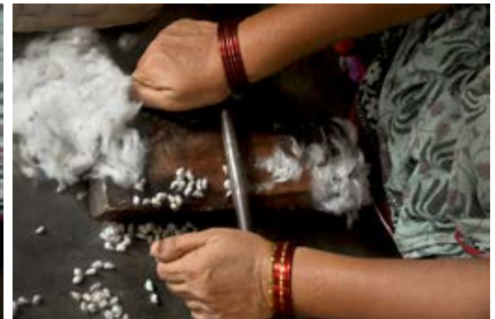
Seeds in the cotton bolls are separated through tapering it using a metal rod.
