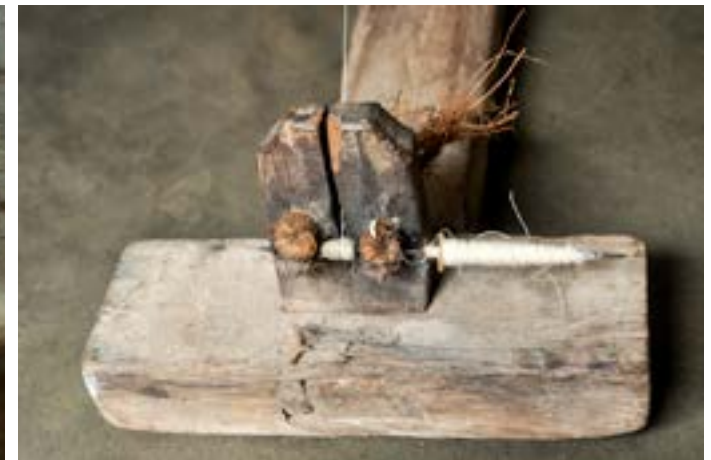
Customized spindle holder is used for holding the spindles to extract the thread from cotton fluff.
