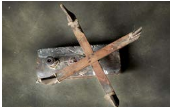
Customized spinner used to convert thread into yarn.
