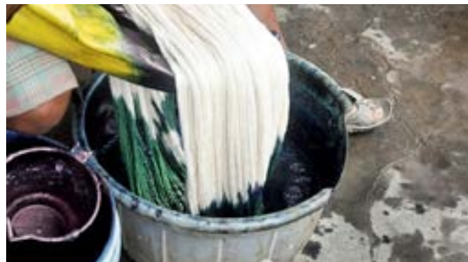
Wet yarn is dipped into the dye mixed container.
