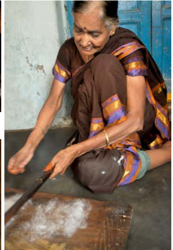
Artisan uses the customized bow to separate the fibers.
