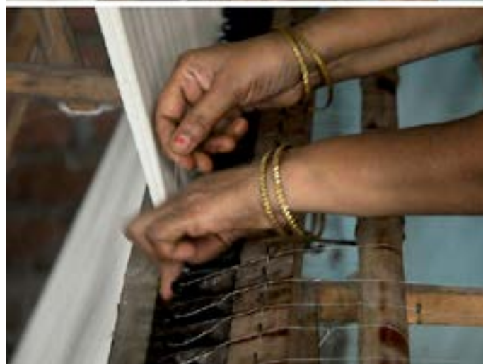
Threads from the cotton bobbin cones are attached to the warping machine.
