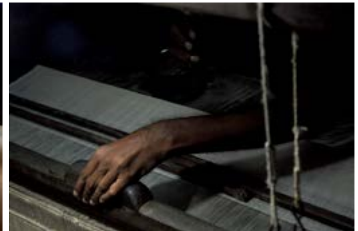
Weaving is formed by pulling the wooden frame towards the weaver.
