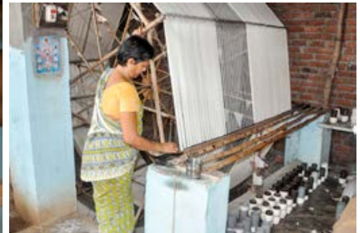
When the warping machine is spun, threads from the thread cones are wrapped on the warping machine.
