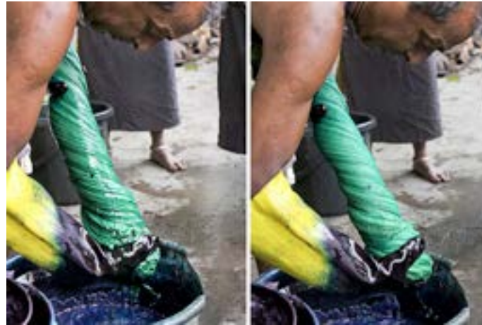
Yarn is twisted for better absorption of colour.
