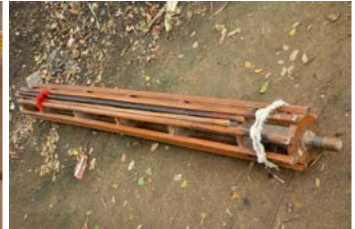
Warping beam is used in the warping process.
