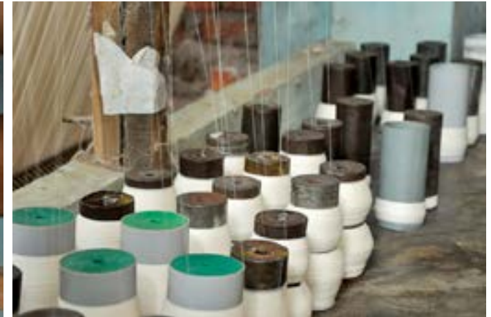
Several thread cones are attached to the warping machine.
