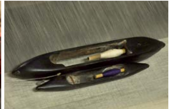
Flying Shuttle is used to carry the thread across the loom weft yarn while weaving.
