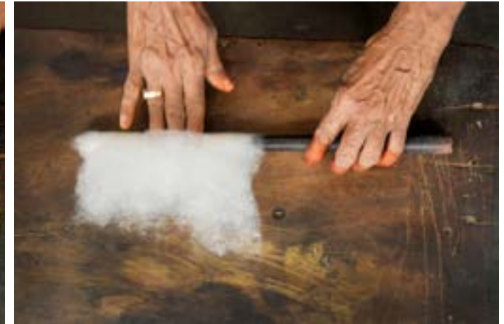
The fluffed cotton is rolled around the metal rod, and the rod is removed.
