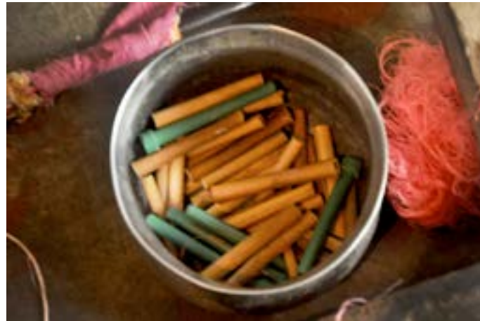
Pirns wound with the cotton yarns used for the weaving process.
