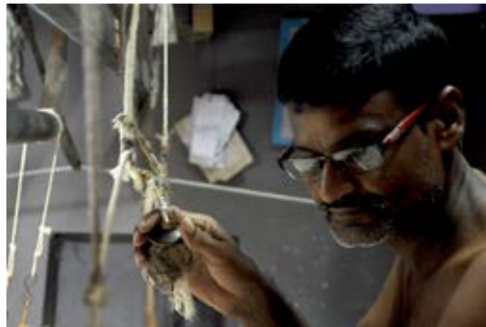
Artisan pulls the cord to move the Flying shuttle in respective directions.
