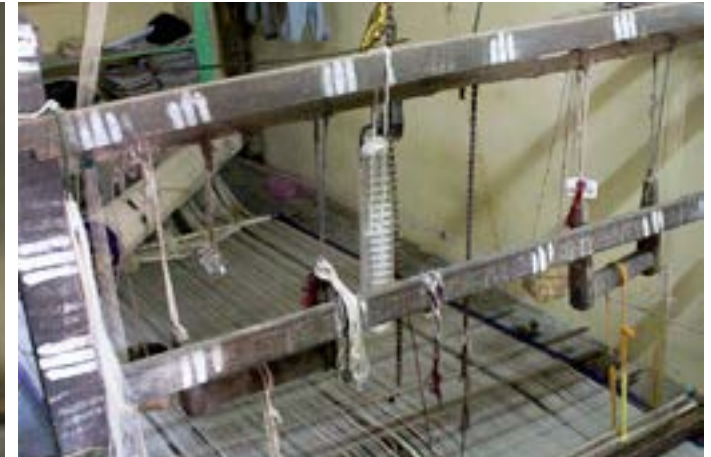
Handloom Pit is used for weaving fabric.
