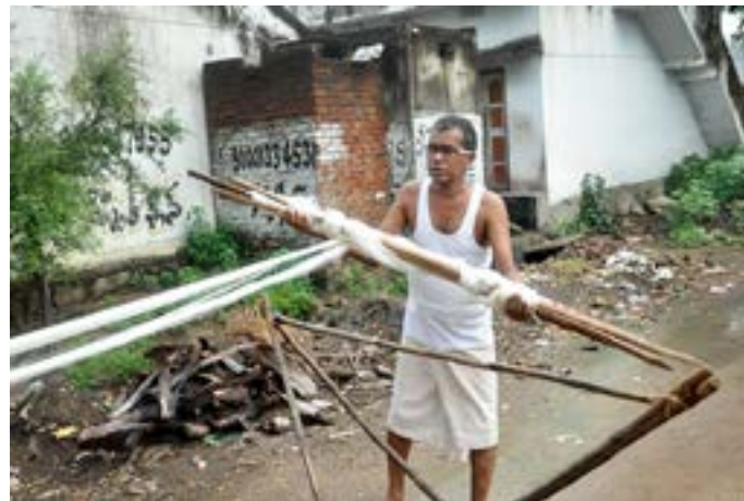
Artisan is making alignment setup for the warping process.
