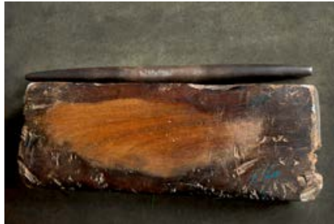
Flat wooden piece and a metal rod are used to remove the seed from cotton.
