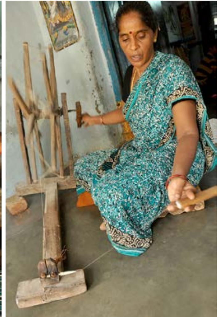
Artisan extracting thread in spindles using thread spinning wheel.
