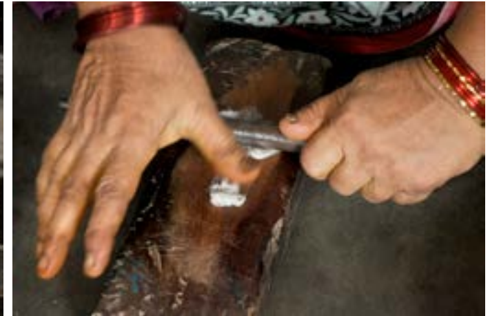
Cleaned cotton bolls are placed on a wooden piece, and a metal rod is rolled swiping the cotton bolls.
