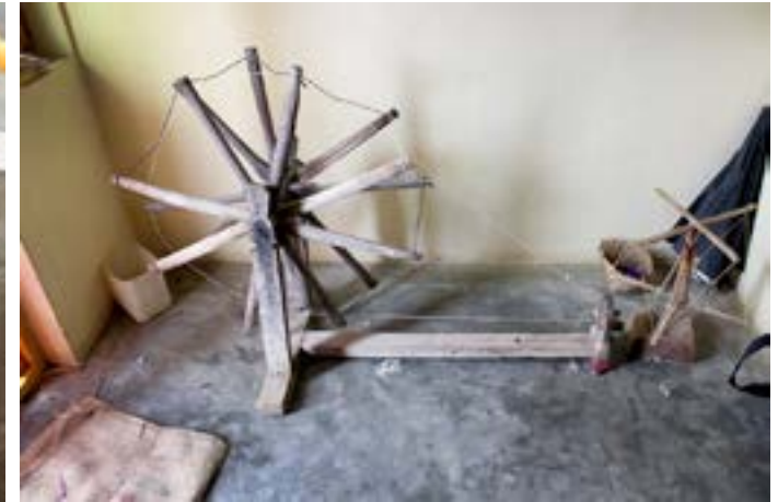
Charkha is used to wind yarns on to the pirns.
