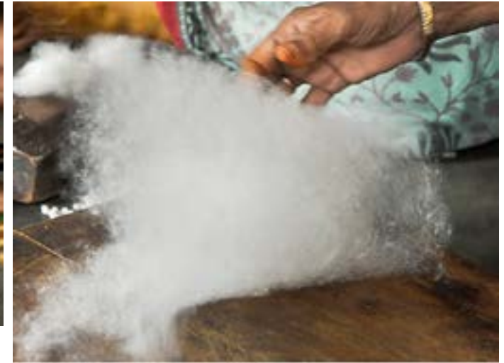
Separated fibers are recombined in opposite directions.
