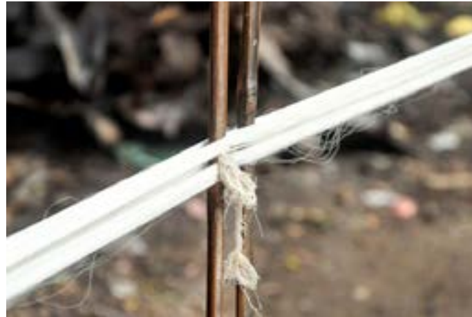
A bamboo stick is added in between the cotton threads.
