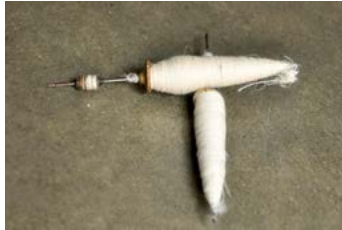
Spindles are used as axis point between thread warping wheel and cotton fluff.
