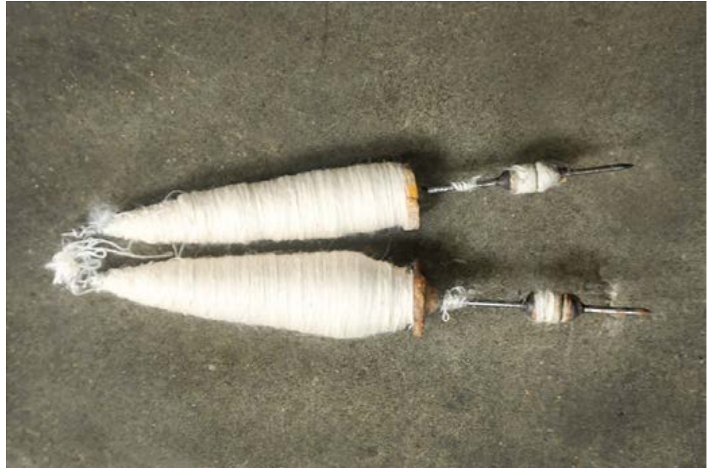
Spindles wrapped with extracted cotton threads.
