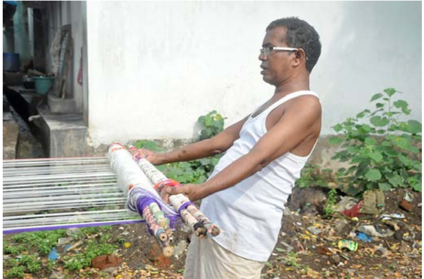
Artisan pulls back the thread and stretches it from one end for checking breakages.
