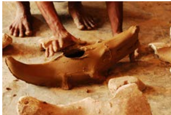
The image shows an example of a form that has been just dismantled from the mould.
