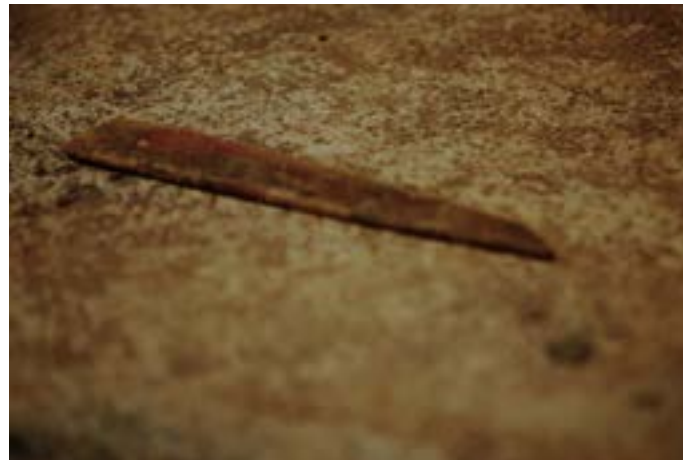
This tool is used on both sides. Both sides help to carve holes or circles on the body of the clay in different sizes.
