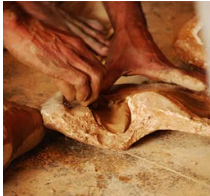
Filling the moulds with the clay by hands.
