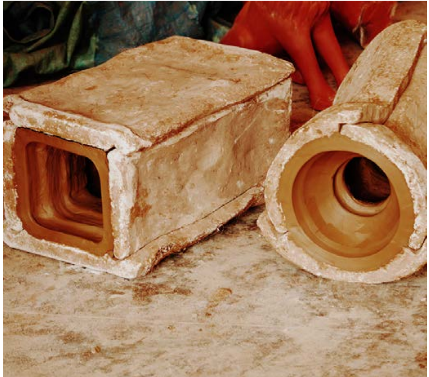
The moulds are kept for drying.
