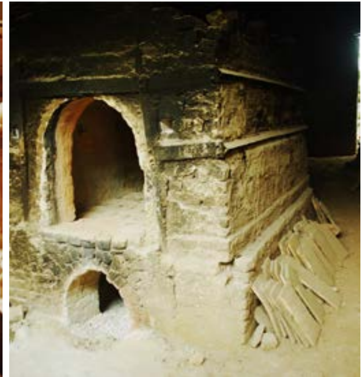
Shows the Furnace in which the clay models are baked.
