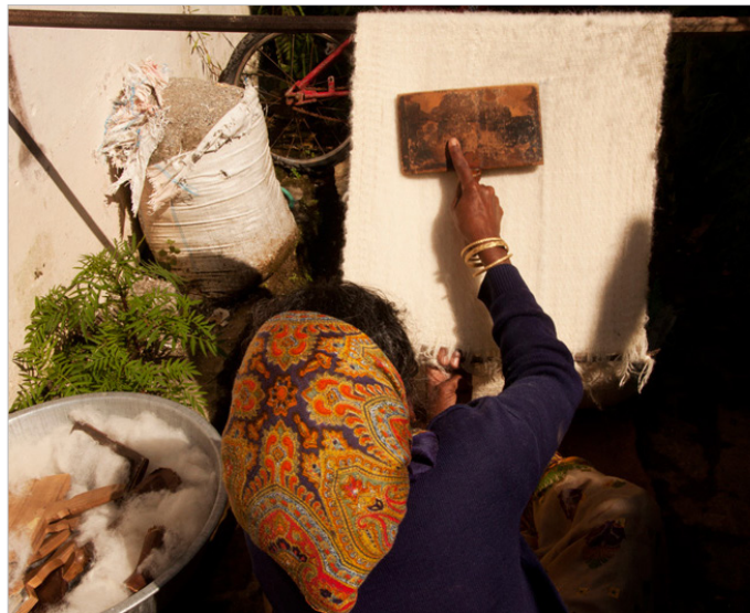
The finished blanket is brushed using the pointed nail brush.
