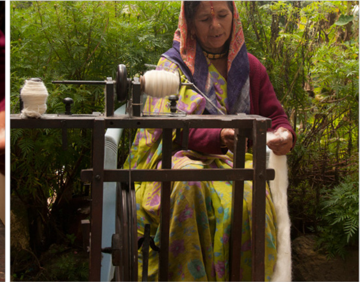
Artisan uses charkha machine to spin the wool into thread.
