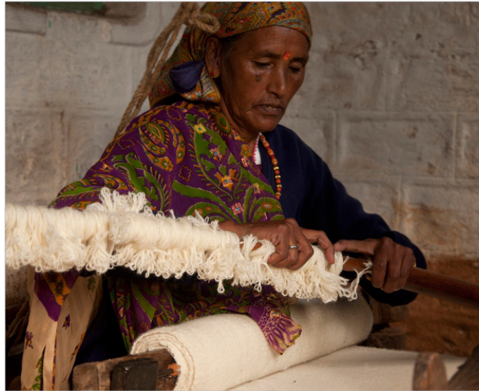
Woolen thread is stuffed into the fly/throw shuttle (which is a bamboo pole).
