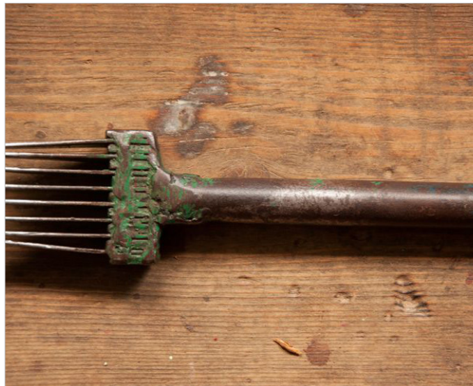
Panja a fork like tool used in beating on the woven threads.
