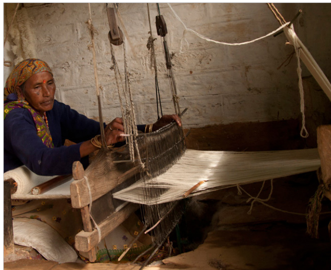
Artisan used four-pedaled loom to weave.
