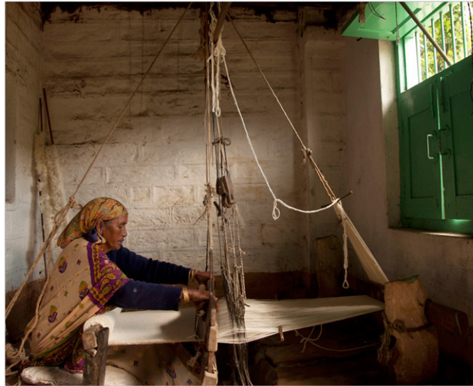
The threads passed through heddles and connected to take-up beam.
