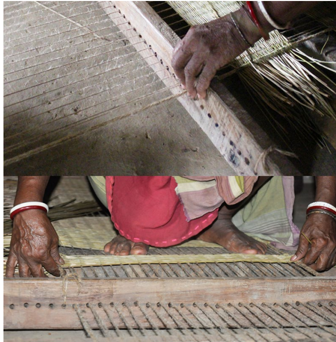
With the help of wooden combs, the reed stalks are pushed together to make them stay intact.
