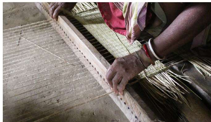
A wooden comb is used to align the yarn and push reed stalks together.
