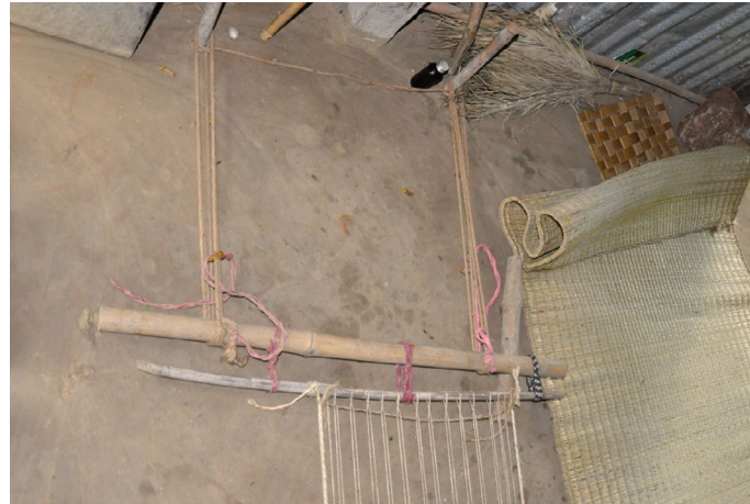
Thick bamboo stalks being tied for strong support.
