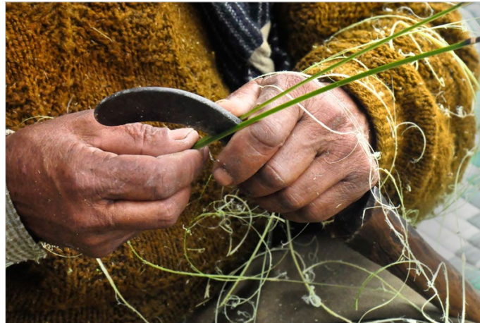
The bamboo is cut into thin strips and the outer layer of the bamboo is peeled using a sharp knife.
