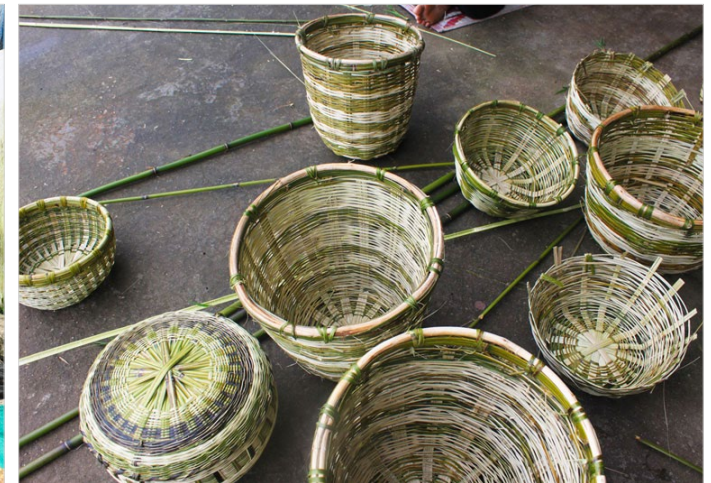
Thick cane poles are used to lock the borders of products for durability of products.
