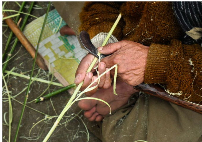
The bamboo is cut into thin strips and fiber is peeled to get smoother surface.
