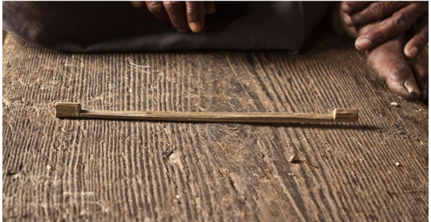
Bamboo stick is shaped to form the front part of the winnow.
