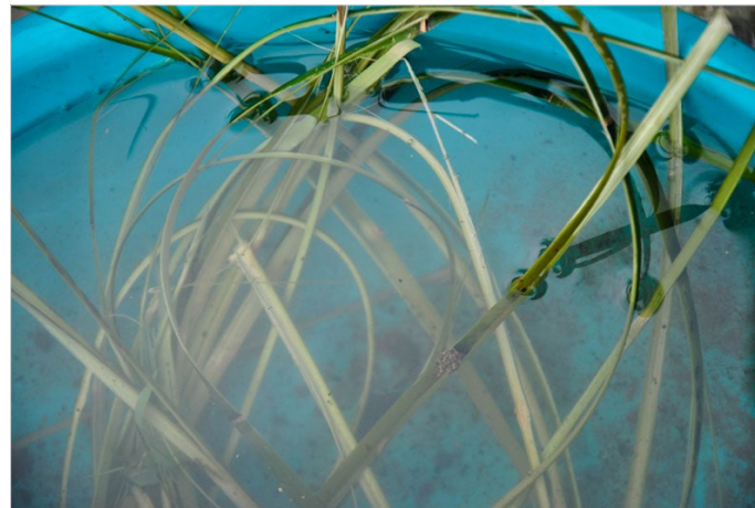
The strips of bamboo are soaked in water to retain moisture and to get flexibility while weaving.
