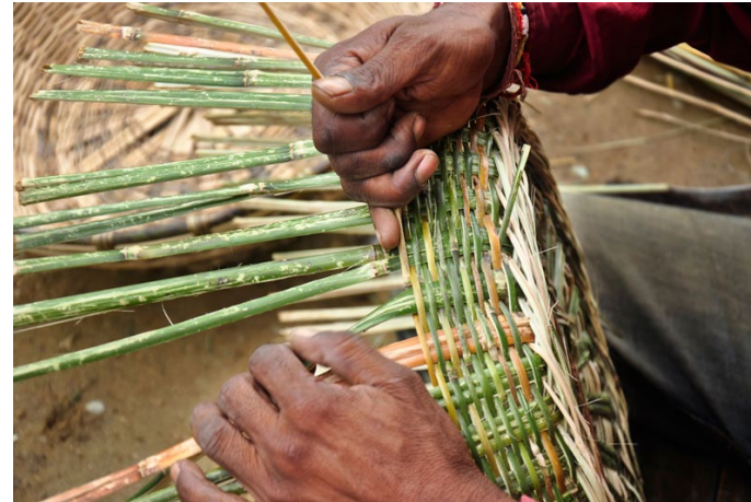
Bamboo strips are joined one after another for the continuity of weaving.
