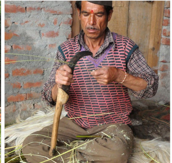
A typical curve shaped knife used to peel and cut the bamboo.
