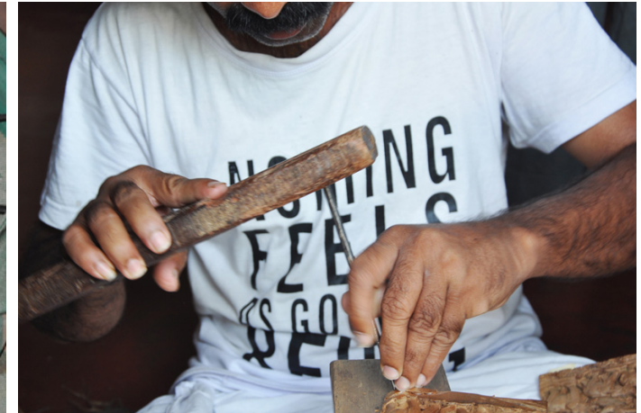
Wooden mallet and chisel is used in carving process.
