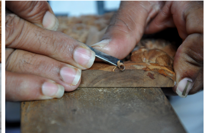
The excess wood is removed as per marked design.
