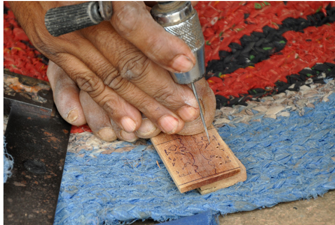
The design is marked on small chip of sandalwood and drilled to make frames.
