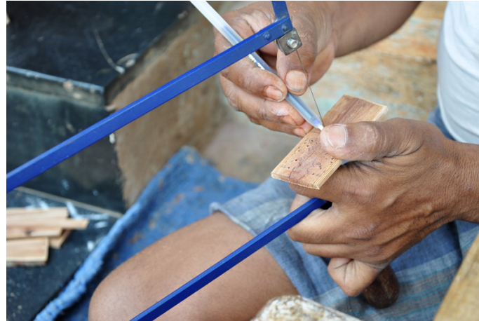
A coping saw is used to cut intricate external shapes.
