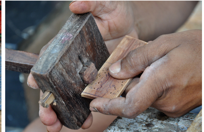
Border of frame is equally drawn with specific tool.
