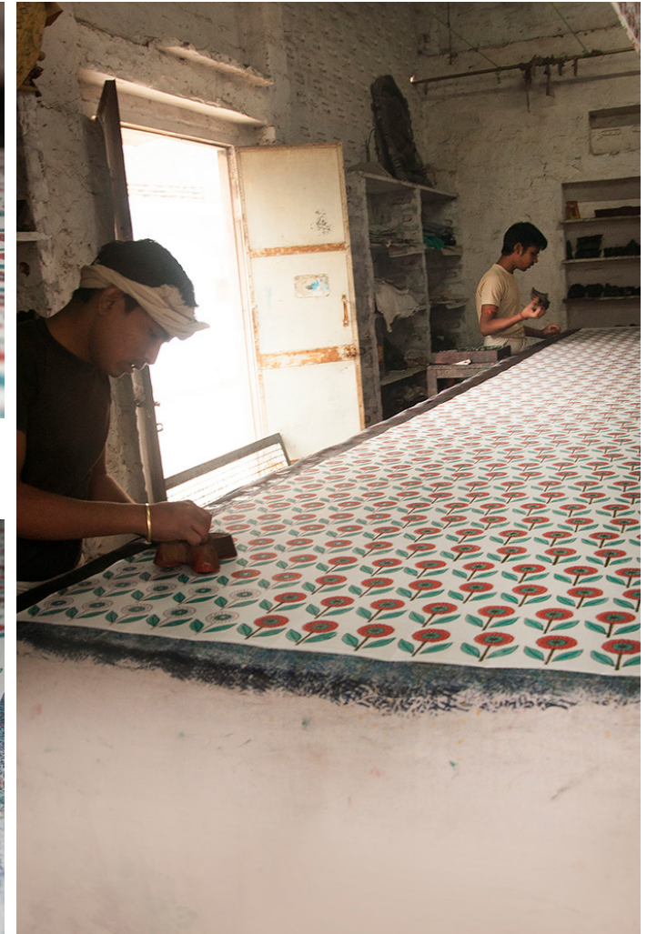
Two artisans working on a single piece of cloth, printing different colors of same motif.
