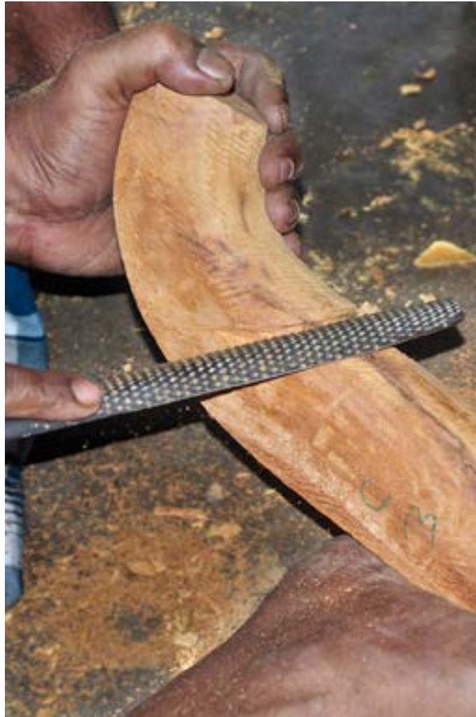
Parts of veena are filed to remove the rough edges.
