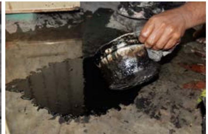
The molten wax is poured on the ground and kneaded/pressed into a dough.
