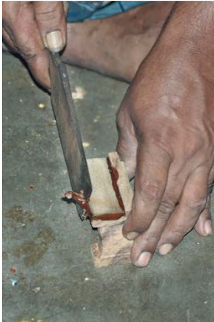
Excess of wax is removed with the help of chisel.
