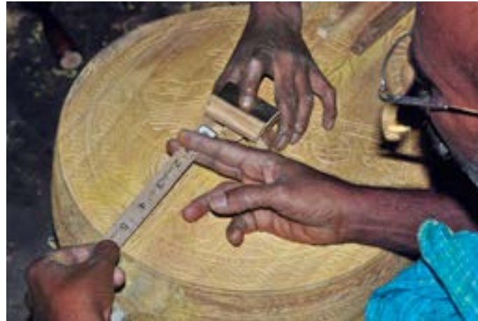
Measurements are taken to place the bridge on the veena at a precise place.
