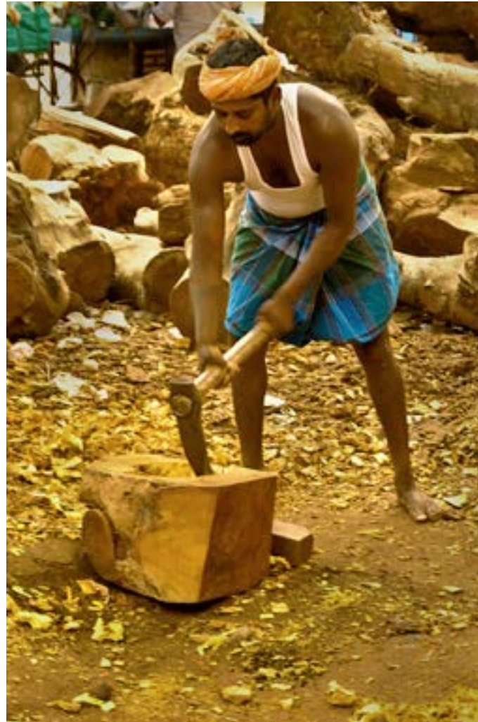
Jack wood is cut into basic shape of veena.
