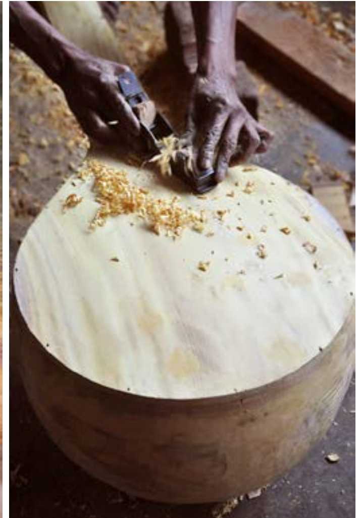
The wood surface is smoothed by scraping.
