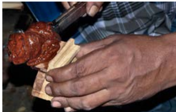
The melted wax is applied on the wooden bridge.
