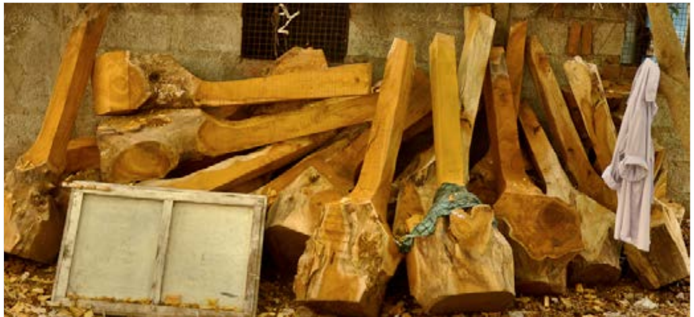
Jackfruit tree log/wood cut in the basic shape of veena.
