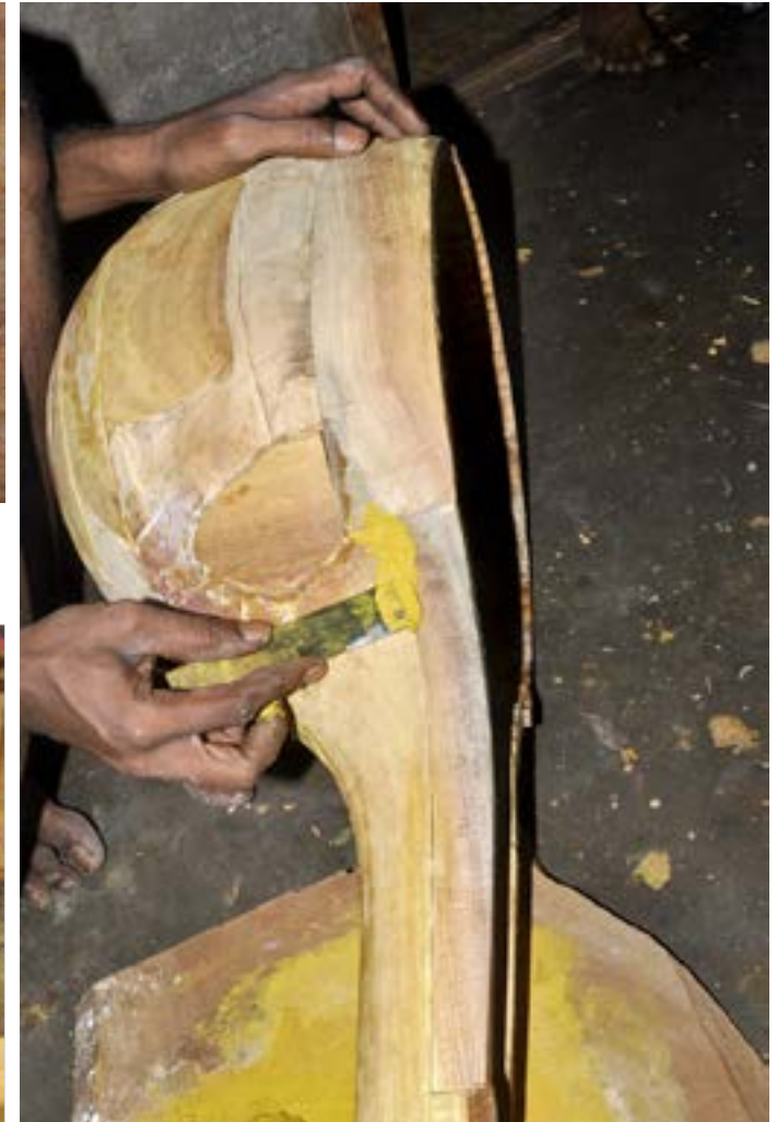
The wood husk mixture is applied on the wood to fill the cracks.
