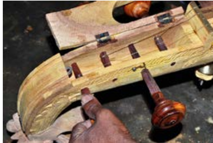
Pegs are turned to tighten the strings.
