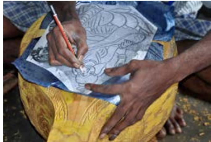
Rough sketch of the design to be carved is traced on the veena.
