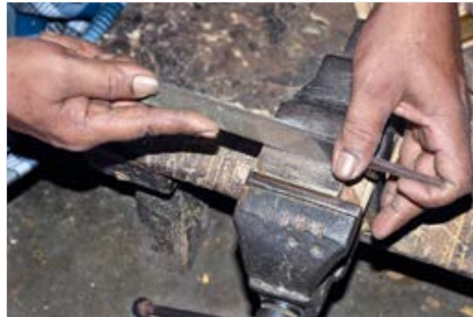
The brass bar is filed/polished to refine the edges.
