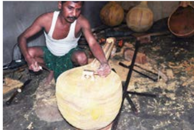
The bridge is fixed to the veena.
