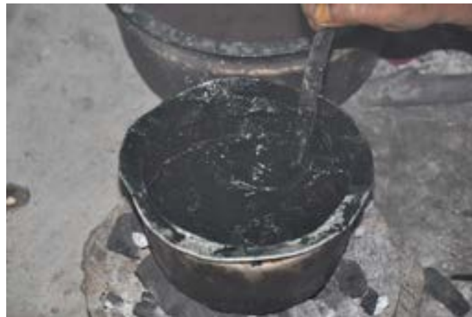
Mixture of bee wax and charcoal powder is melted.
