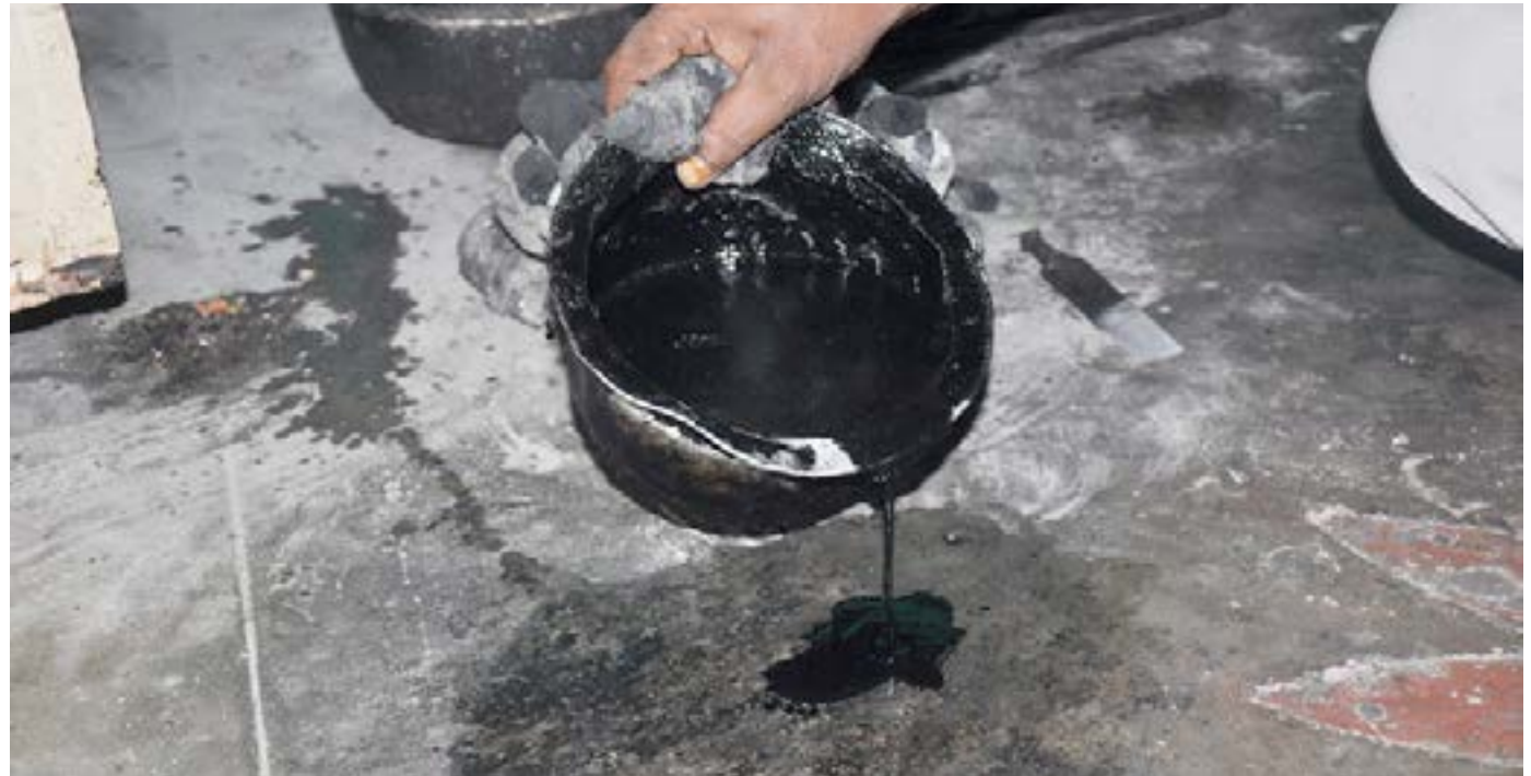
Mixture of beeswax and coal powder used to make the base for the brass metal frets.
