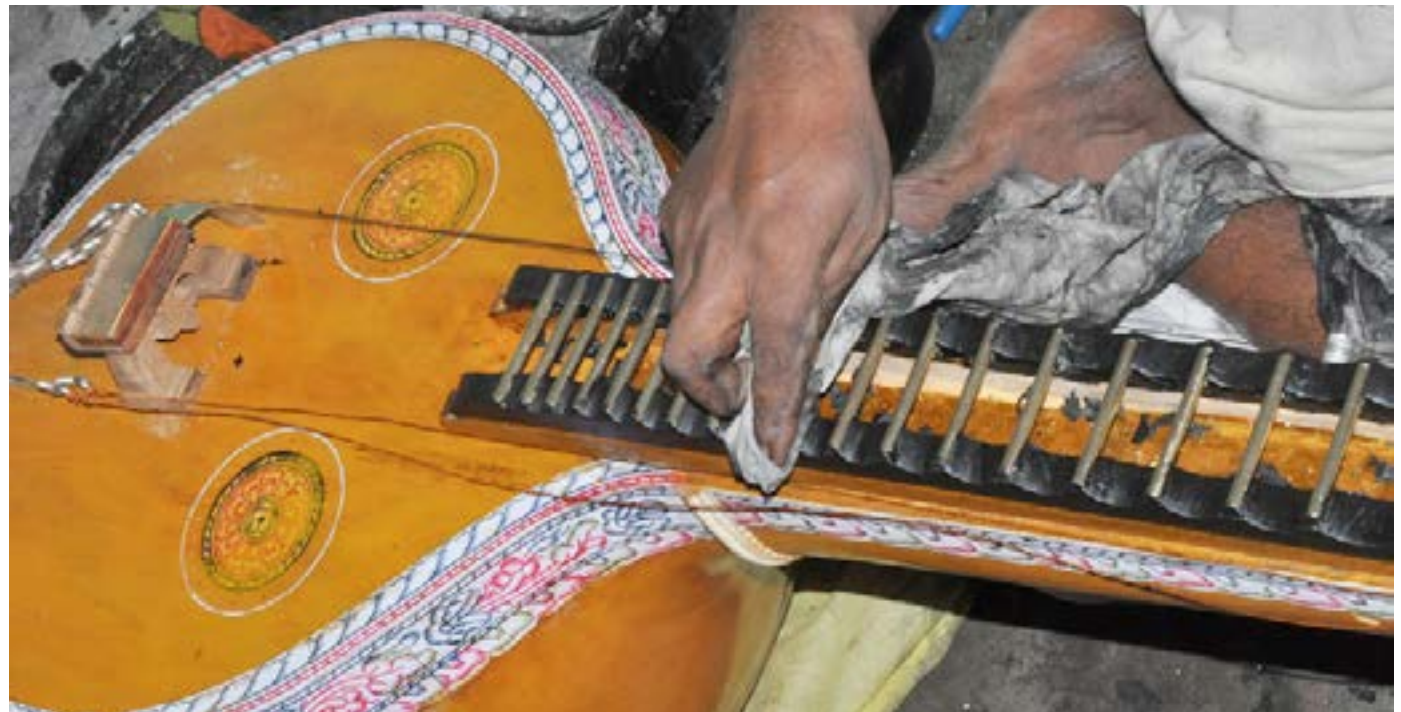
The wax strip is cleaned with kerosene to give smooth finishing and shine.
