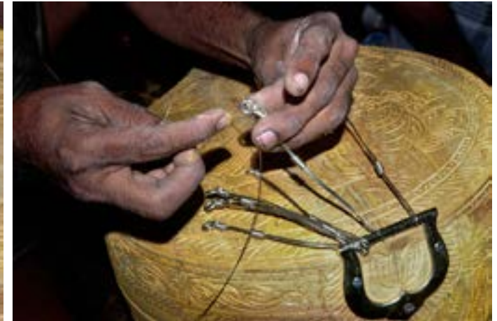
The strings are attached to the metallic clasp.
