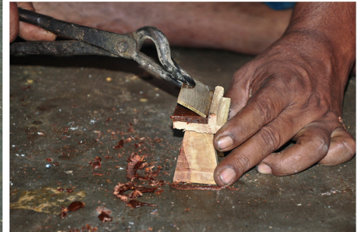
The heated brass piece is placed on the wax to fix firmly.
