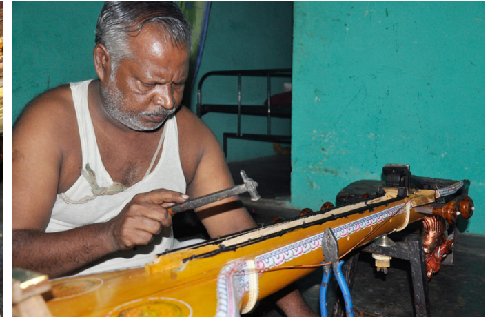
Nails are hammered to hold the bee wax strip firmly.
