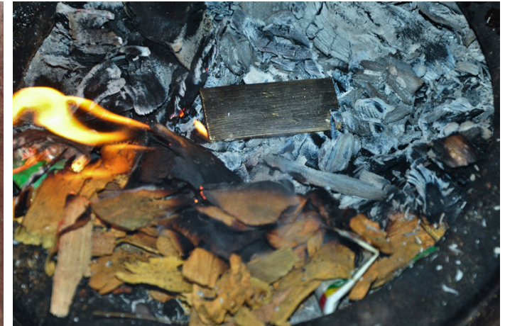
The brass bar is again heated to fix it on the wax.
