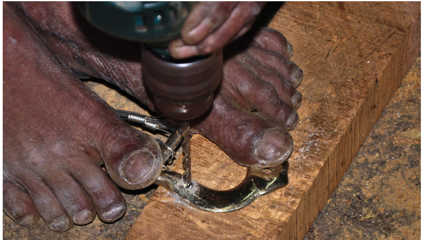
A hole is drilled on the metallic clasps.
