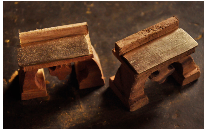
Wood is carved/cut in the shape of a bridge.
