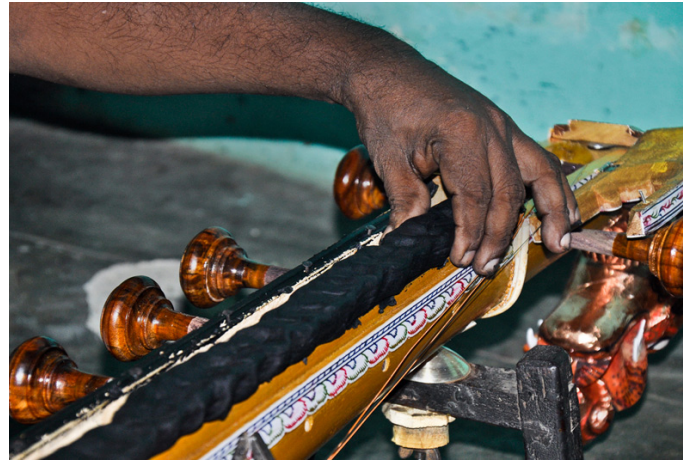
Strips of wax dough is made and fixed on the veena's neck.
