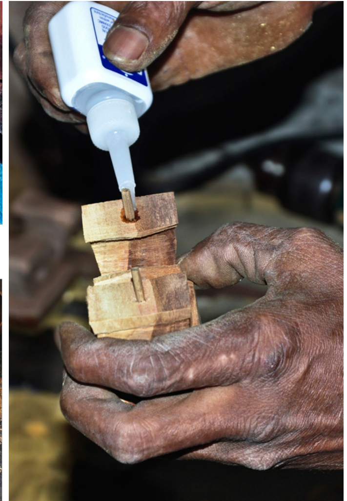
Adhesive and wood husk is applied underneath the bridge piece.
