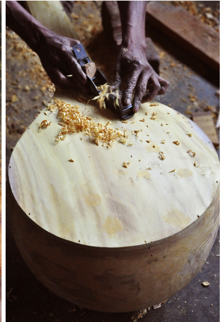
The wood surface is smoothed by scraping.
