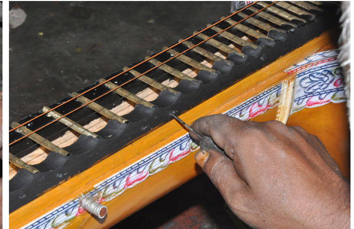
Holes are made on the wax strip to specify the main tune notes.
