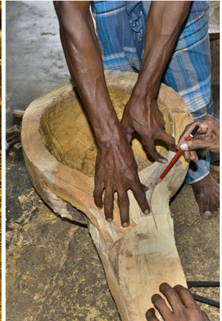
Measurements are marked for the exact shape of the veena to be carved.
