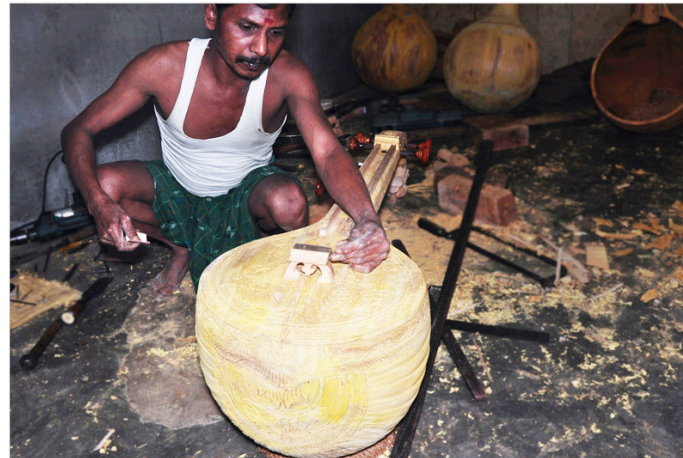
The bridge is fixed to the veena.
