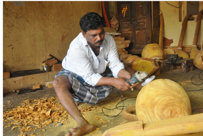
Buffering machine is used to buffer the wood surface for a smooth finishing.
