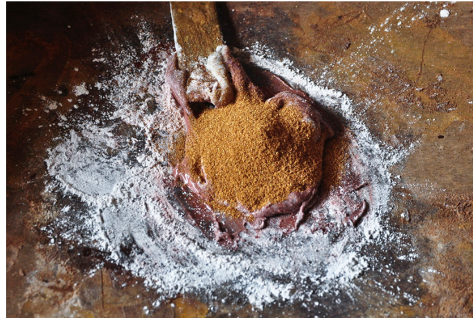
Mixture of jack wood husk, pop powder, yellow colour powder and adhesive is made.
