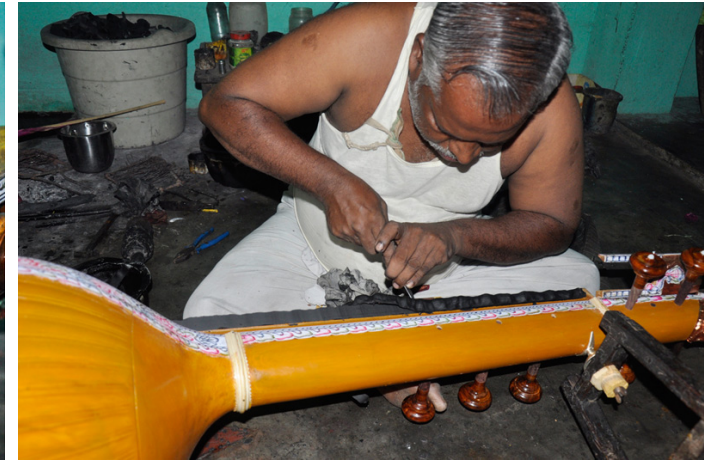
Artisan fixes the brass metal frets on the wax strip.
