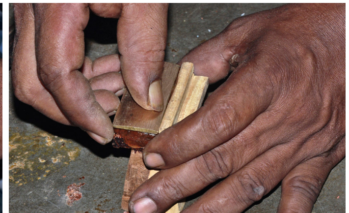
A flat brass bar is fixed on the bridge with help of bee wax.
