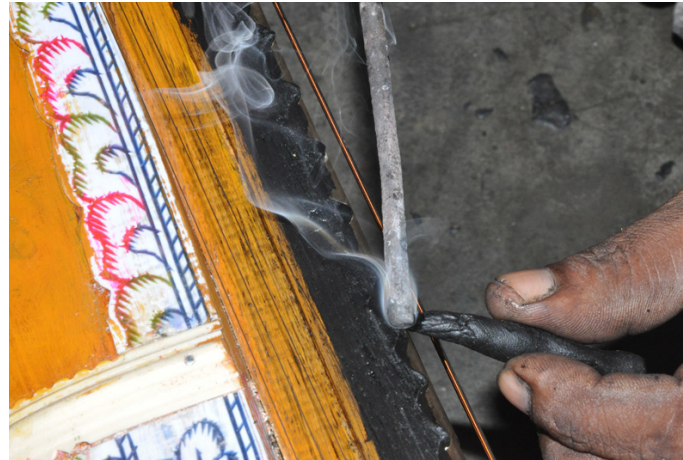
The edges of the frets are locked with wax.
