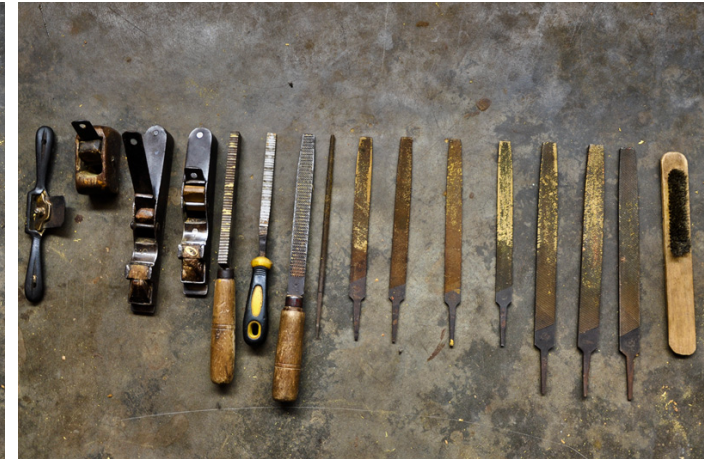
Multi sizes of files and wood scrapers used to smoothen the wood surface of veena.
