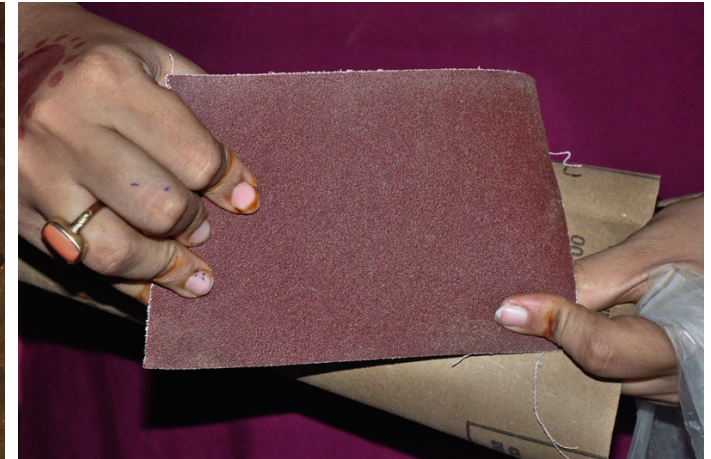
Sandpaper is used to smoothen/polish the wood surface.
