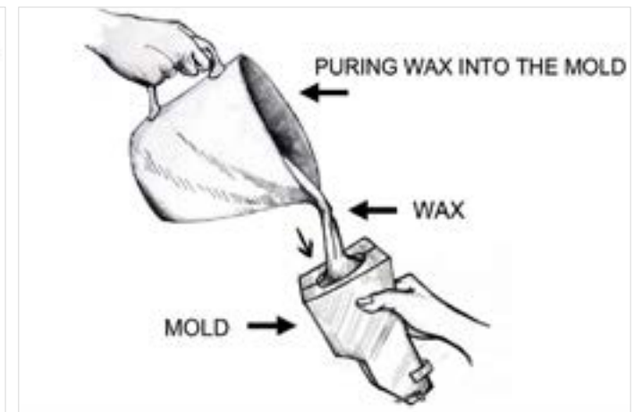
Molten wax is poured into the mold and allowed to set for 20 minutes.
