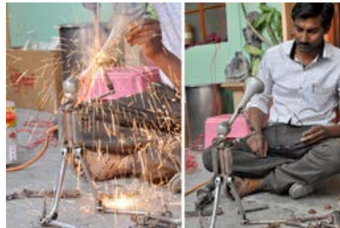
The funnel being welded to make a trumpet and some small iron rods to form its hands.
