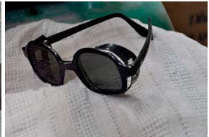
Welding goggles were used to protect the artisan's eyes from the spark emitted during the welding process.
