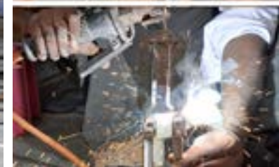
The second pedal rod is welded, to complete the lower body.
