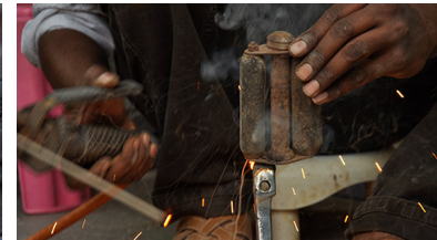
Welding cycle pedal rod as a base to form the legs of the sculpture.
