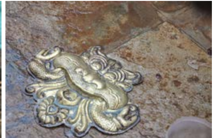
Product is washed with tamarind pulp to obtain shine and luster.
