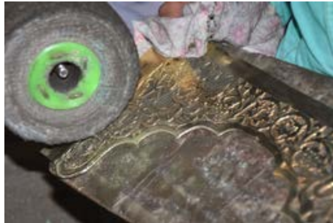
The article is buffed and polished.
