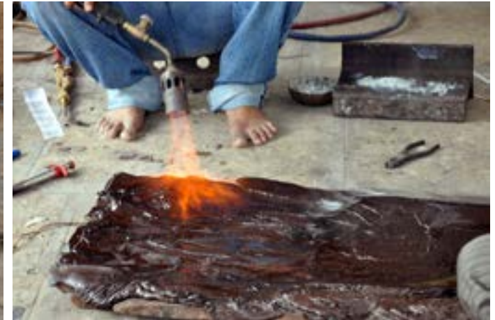
Melted lac is spread on the wooden plank and heated.
