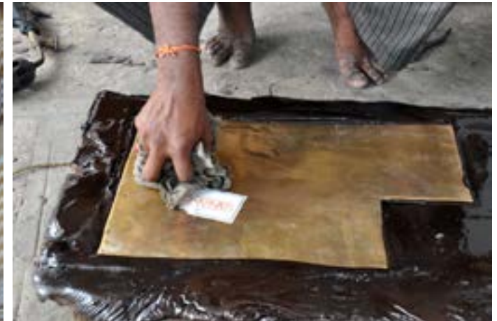
Metal sheet is placed on the melted lac and kept to dry.
