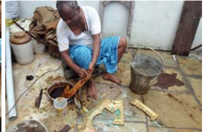
The embossed sheet is washed with tamarind pulp.
