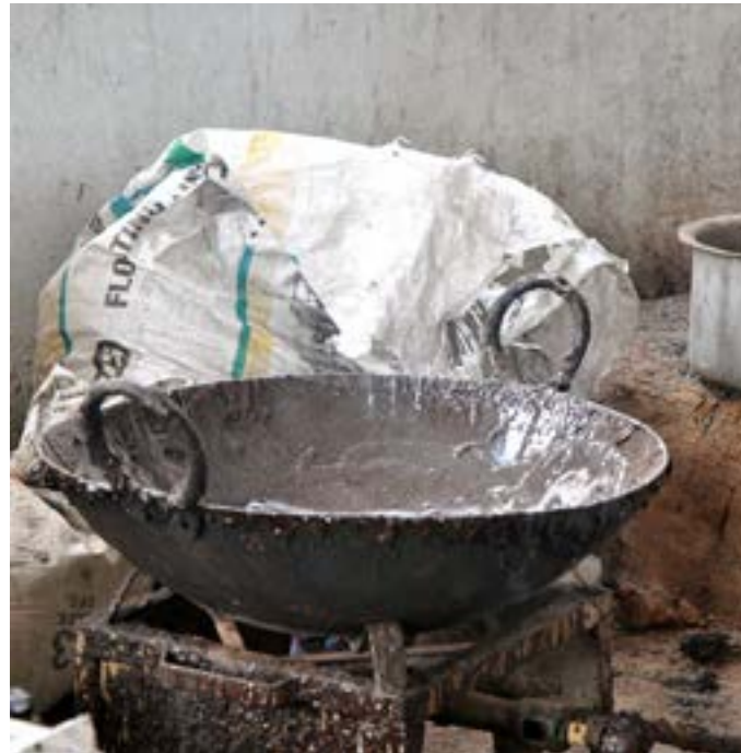
Karahi- thick, circular, and deep cooking pot used to melt the lac.
