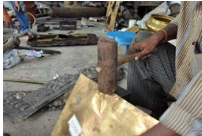
Metal sheet is hammered on the sides.
