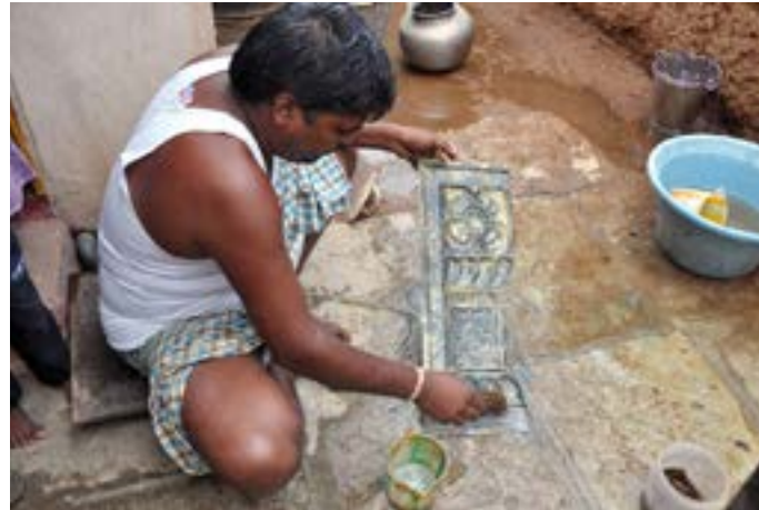
Finished product is washed with acid.
