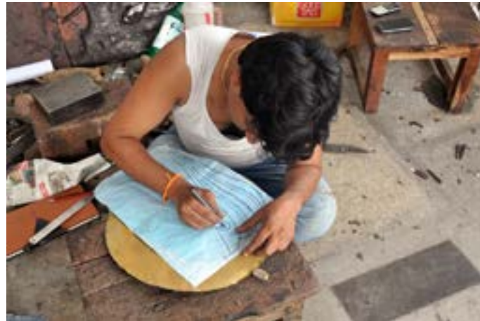
The design is drawn on a sheet.
