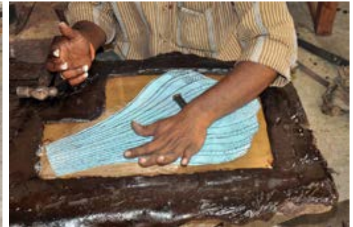
The design sheet is pasted on the metal sheet.
