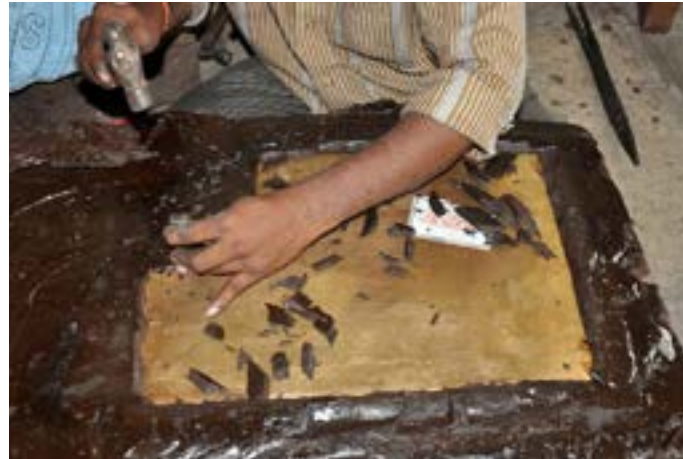
Extra lac on sides are hammered and removed.
