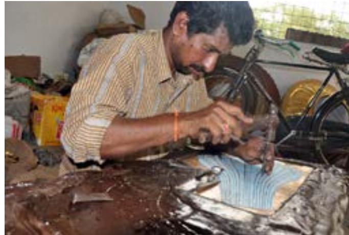
Artisan carves the design with chisel following the design line.
