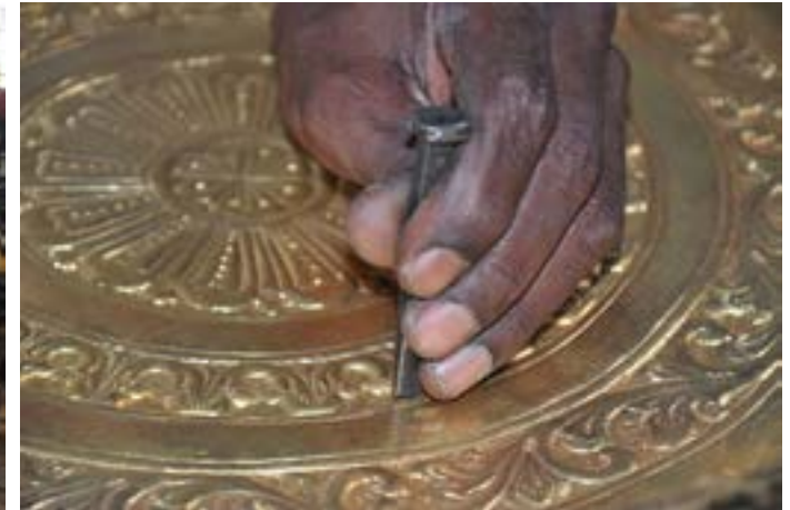
Detail work is embossed with small chisels.
