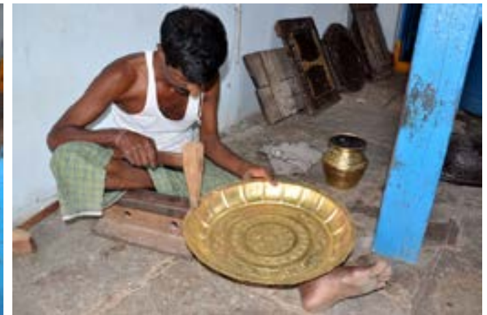
Sides of the art plate is hammered and flattened.
