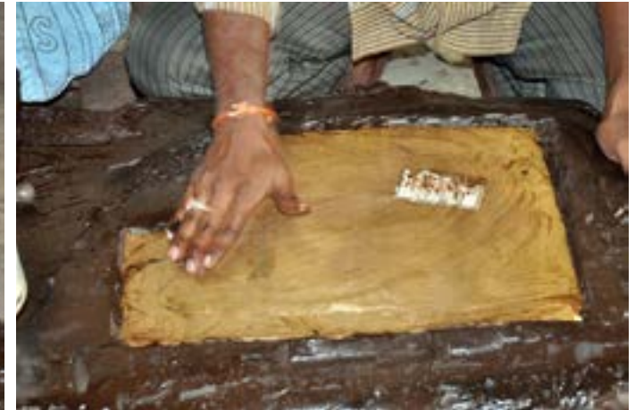
The metal sheet is cleaned with tamarind pulp.
