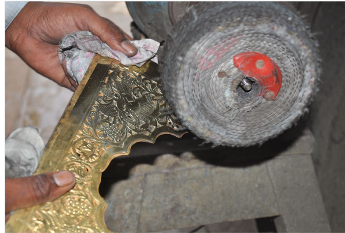
Buffing process is done to smoothen the sharp edges and gives shine to the product.
