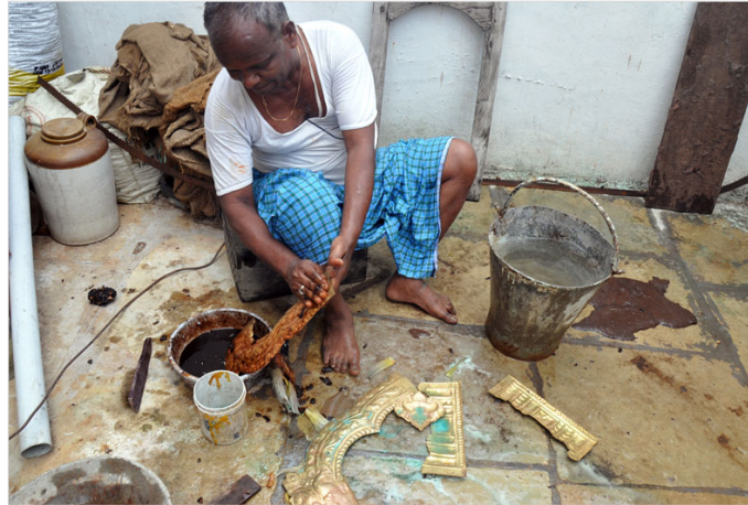
The embossed sheet is washed with tamarind pulp.
