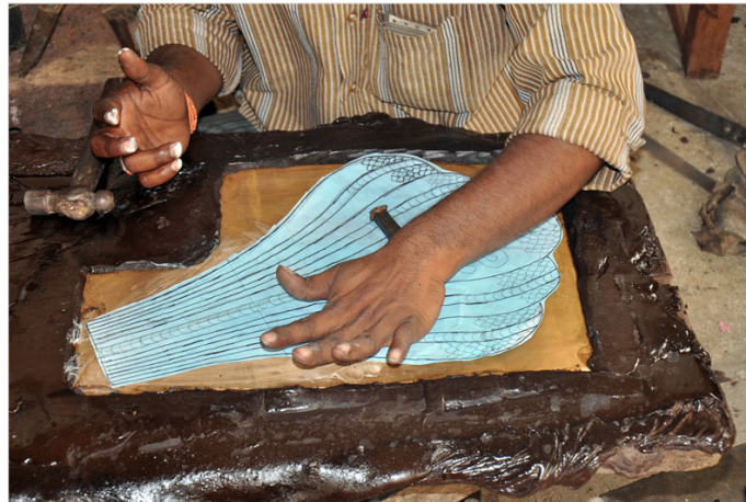
The design sheet is pasted on the metal sheet.
