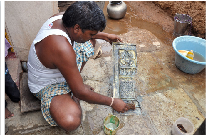
Finished product is washed with acid.
