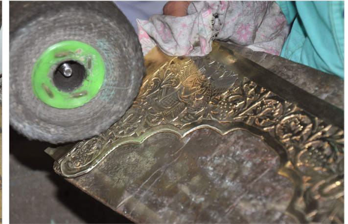
The article is buffed and polished.
