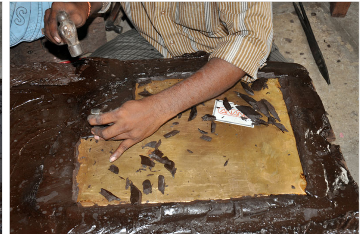
Extra lac on sides are hammered and removed.
