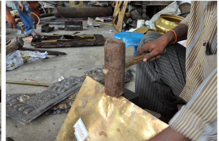
Metal sheet is hammered on the sides.
