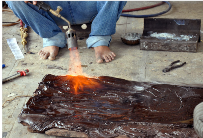
Melted lac is spread on the wooden plank and heated.
