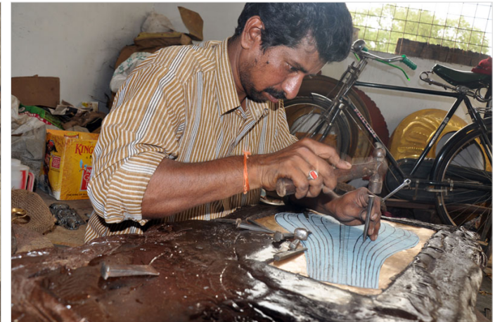
Artisan carves the design with chisel following the design line.
