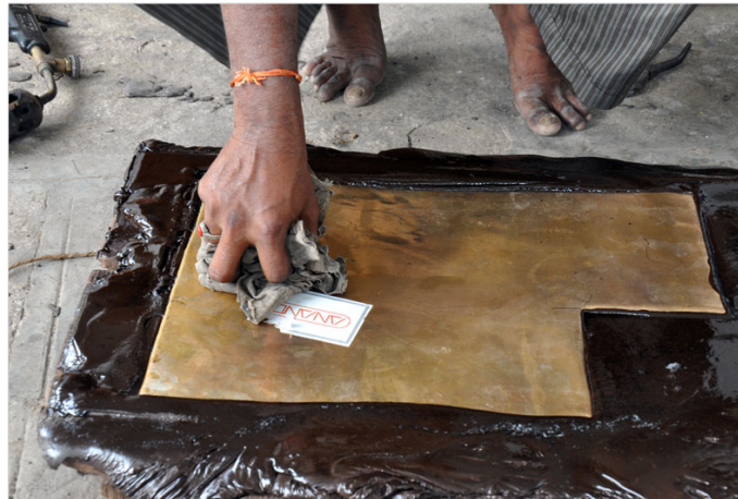
Metal sheet is placed on the melted lac and kept to dry.
