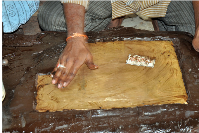
The metal sheet is cleaned with tamarind pulp.
