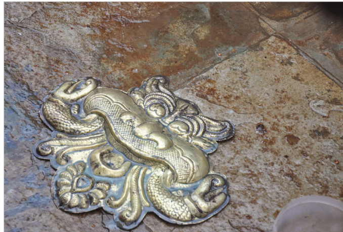
Product is washed with tamarind pulp to obtain shine and luster.
