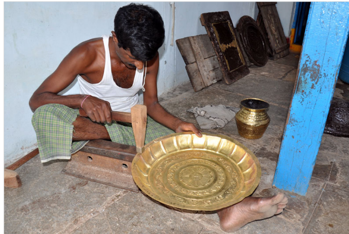
Sides of the art plate is hammered and flattened.
