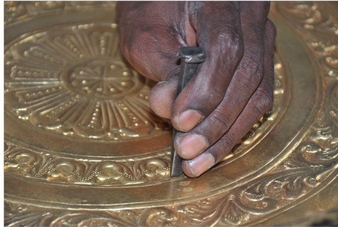
Detail work is embossed with small chisels.
