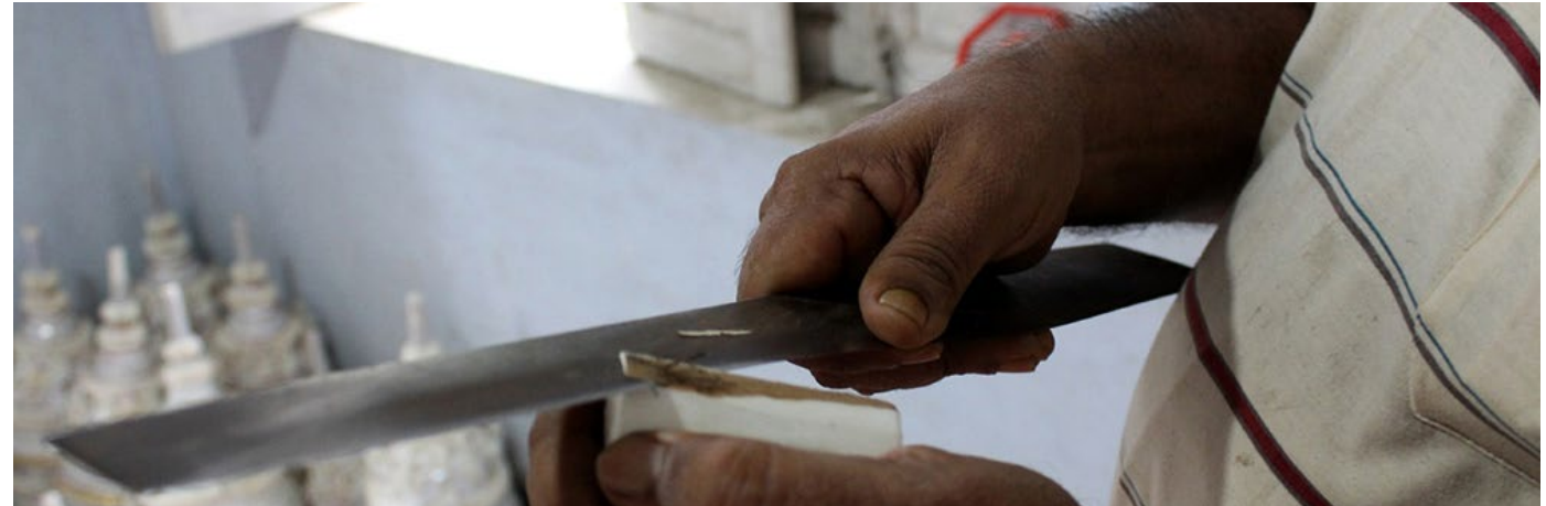
The thick outer skin of the shola wood is removed using a Kath (knife).
