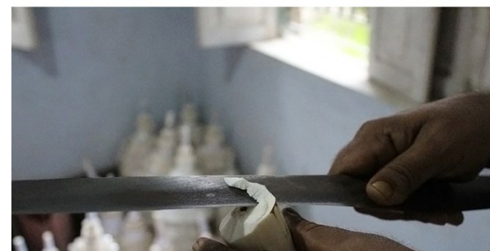
Artisan using shaving tools to turn shola plants into thin sheets.
