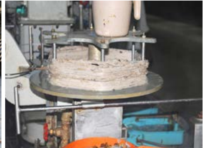
The waste from the brushing device is wound.
