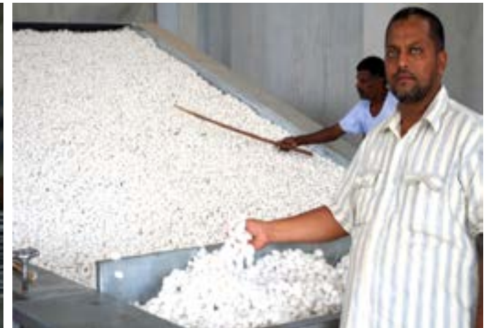
They are spread evenly over the surface to ensure heating and extermination of the worms.
