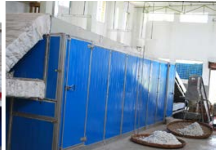
Hot Air Cocoon Drying Machine is the latest machinery used to dry the cocoons.
