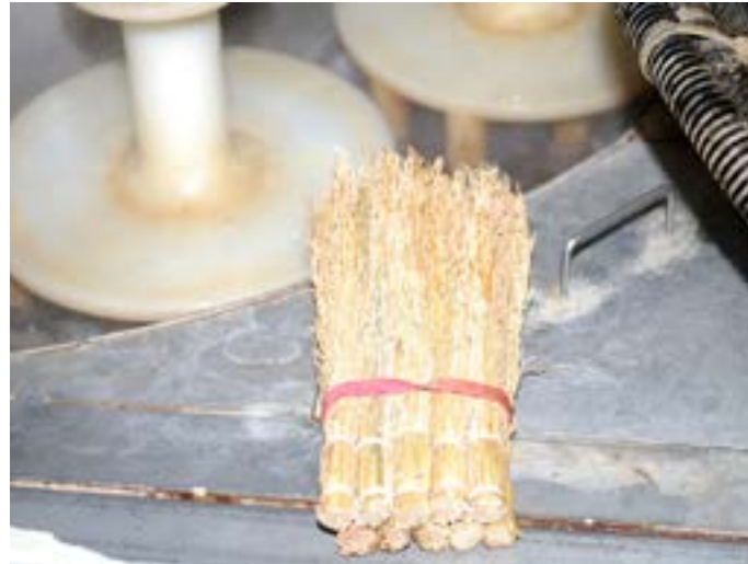
A bunch of coarse paddy stalks are attached to the brushing device.
