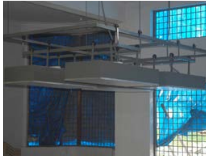
Test Plate is a special equipment to inspect the quality of raw silk.
