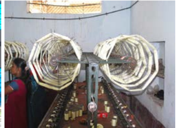
The yarn is wound on the silk winding machine to be reeled into spools.
