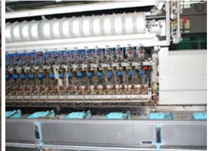
Automatically the filament is picked from the cocoon and reeled.
