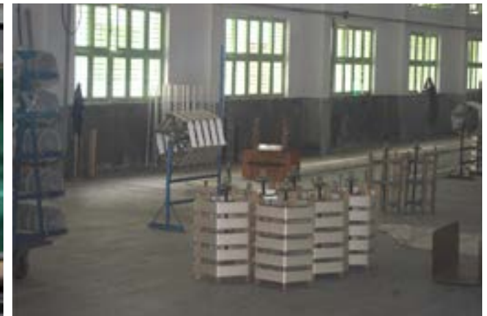
The hanks are detached from the reeling machine for further compression and packaging.
