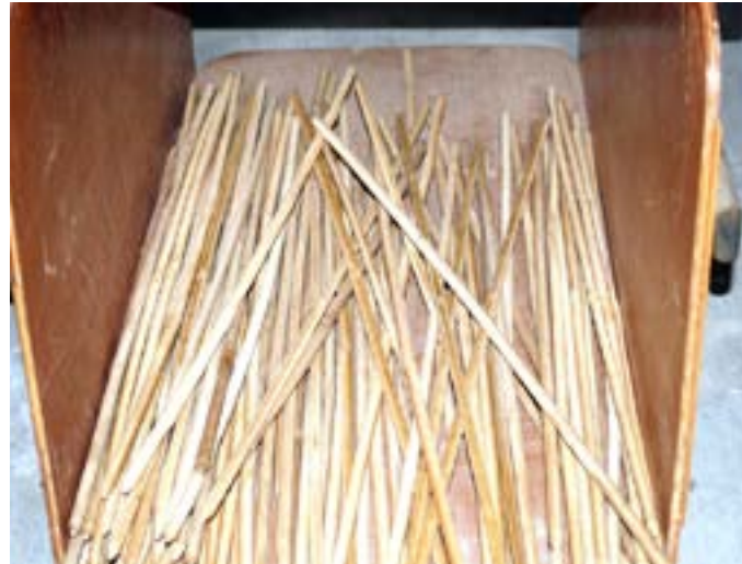
The bamboo sticks are used to stretch the yarn and increase its strength.
