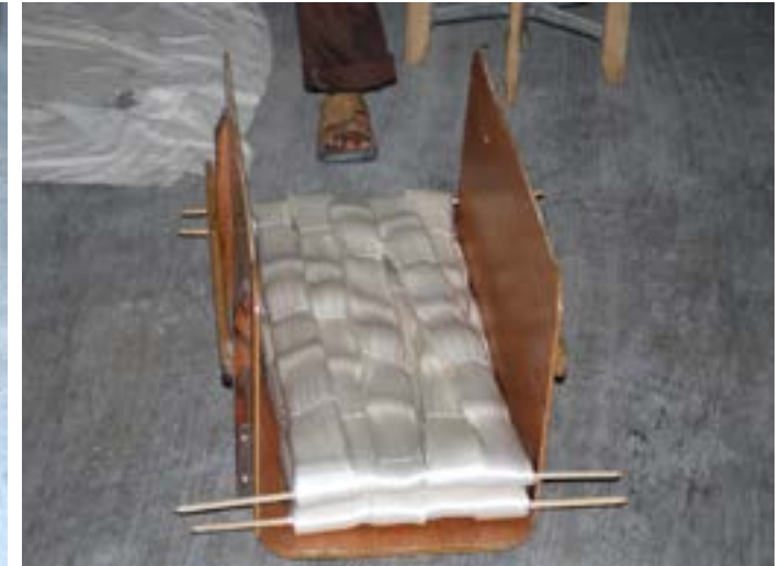
The yarn is affixed to the bamboo sticks and stacked one above the other.
