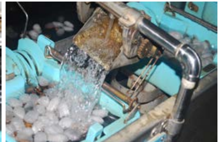
This machine maintains the water level in the tray for cooling and segregation of adjoining cocoons.
