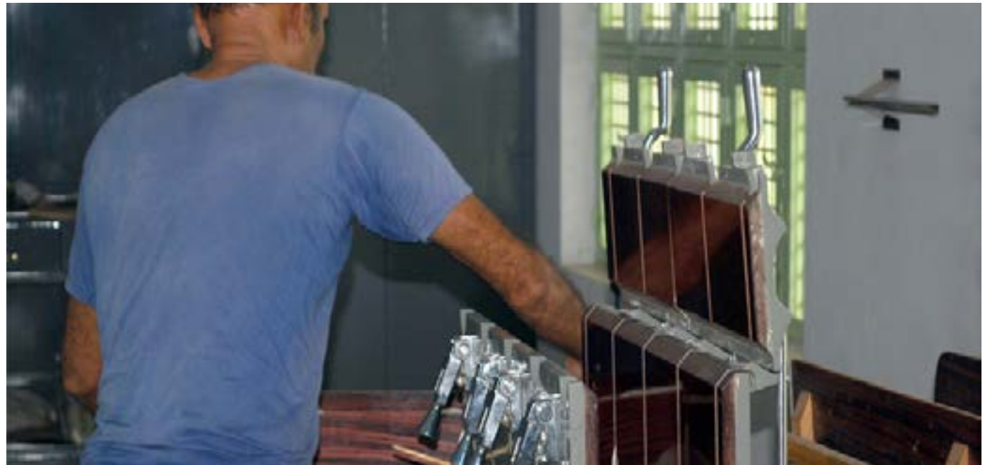
The silk yarn is placed in the compression machine to enable compression of the yarns.
