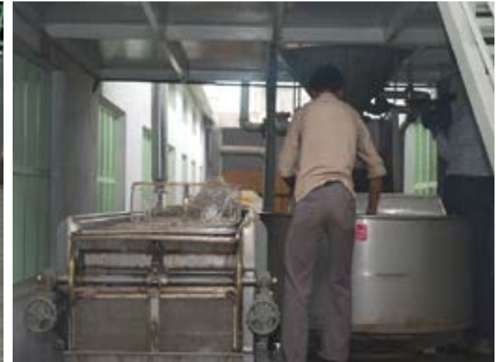
After the process of cocoon cooking, they are transferred to trays for cooling.
