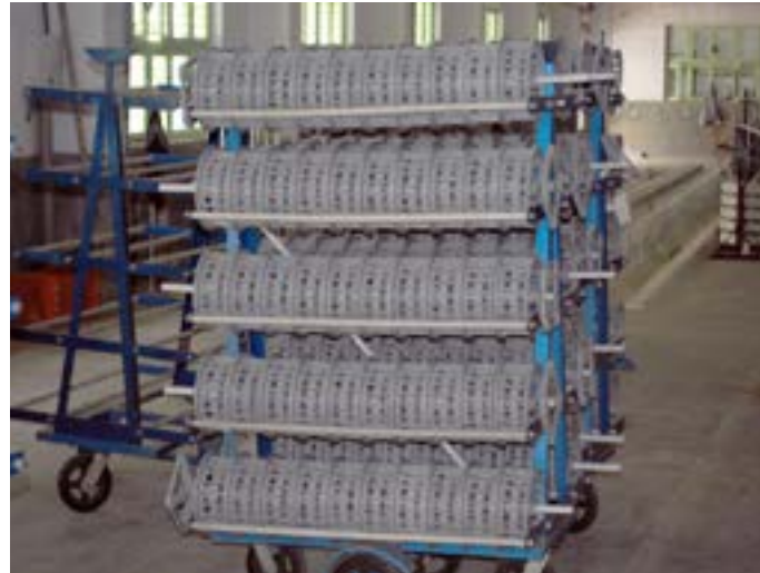
The hanks are to be loaded on the machine to enable the reeling of the silk yarn.
