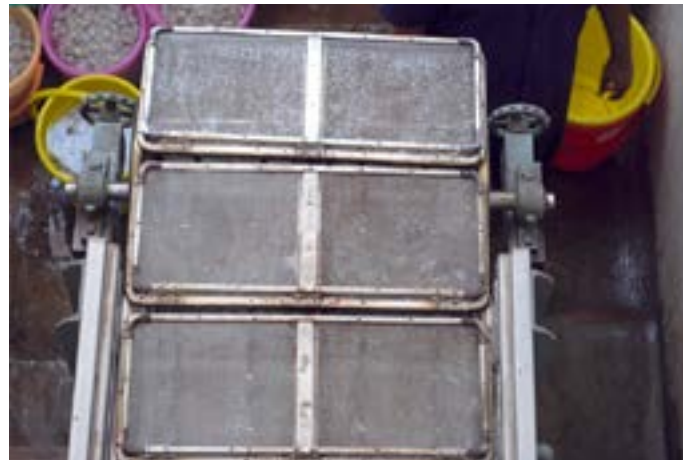
The tray has pores for the water used for cooling to be drained out.
