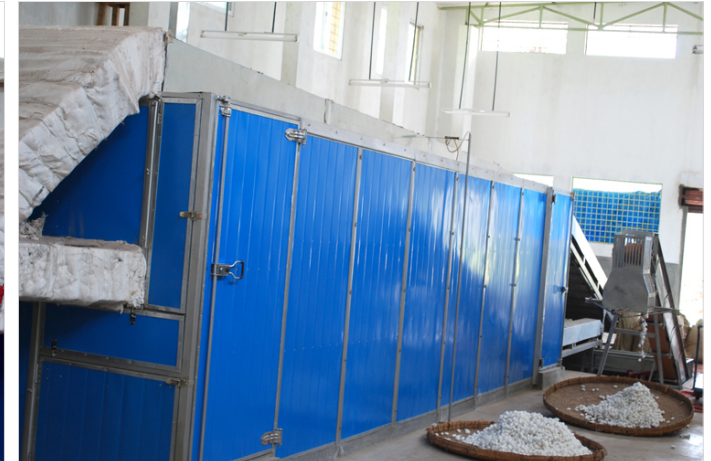
Hot Air Cocoon Drying Machine is the latest machinery used to dry the cocoons.
