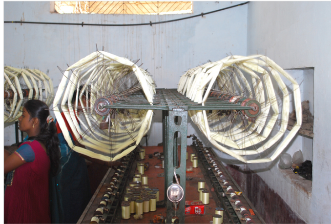
The yarn is wound on the silk winding machine to be reeled into spools.
