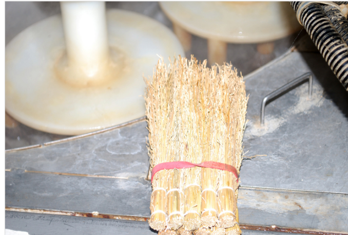
A bunch of coarse paddy stalks are attached to the brushing device.
