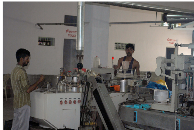
People feeding the cocoons to automatic silk reeling machine to undergo cleaning and reeling process of the cocoons.
