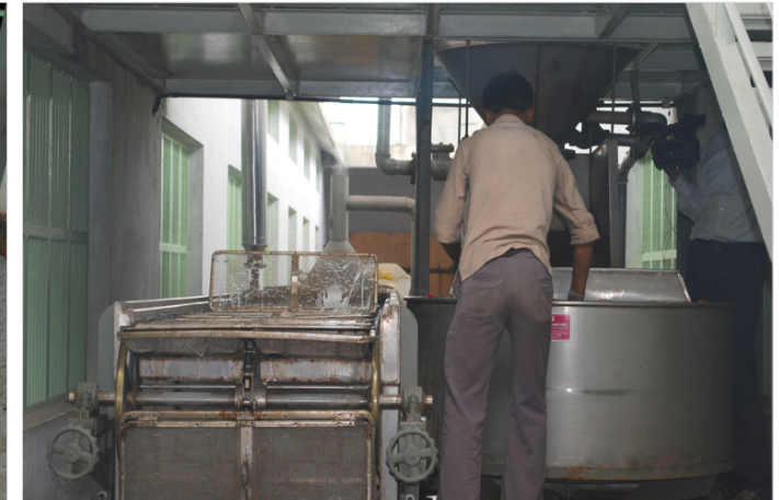
After the process of cocoon cooking, they are transferred to trays for cooling.
