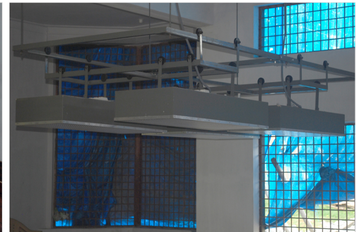
Test Plate is a special equipment to inspect the quality of raw silk.
