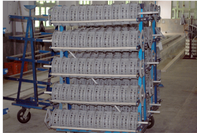
The hanks are to be loaded on the machine to enable the reeling of the silk yarn.
