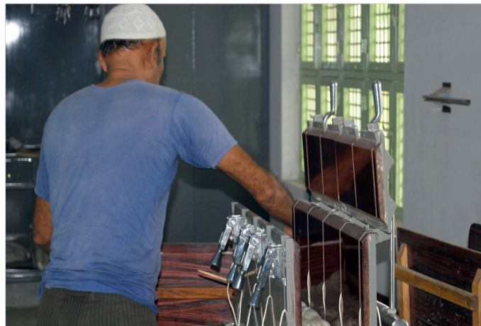
The silk yarn is placed in the compression machine to enable compression of the yarns.
