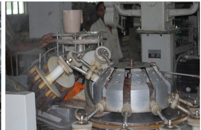
The brushing device to remove the coarse fibers of the cocoons.
