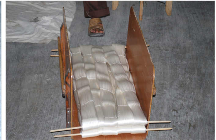
The yarn is affixed to the bamboo sticks and stacked one above the other.
