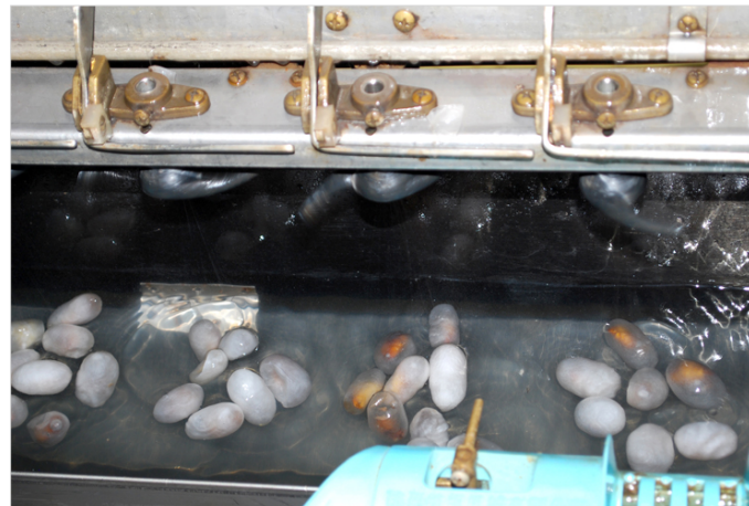
The machine automatically picks the filament from the cocoon and reels it.
