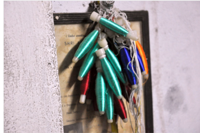
Plastic weft winding pin to be used inside the shuttle.
