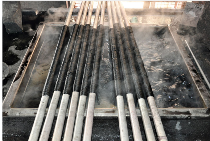
The bundle of yarn are hanged/ hung from the metal rod and dipped in a tank with boiling water and color.
