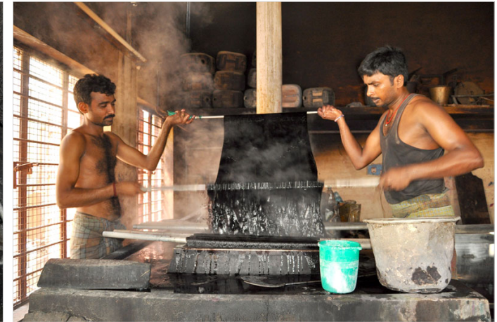
Two artisans work together to rotate/roll the yarns systematically so that the color spreads evenly.
