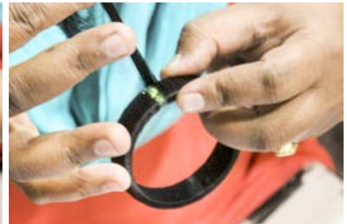
Artisan making sure there are no gaps after the winding process is completed.
