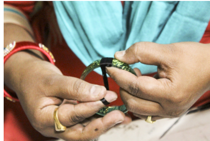
The artisan starts winding the thread around the bangle which is applied with glue.
