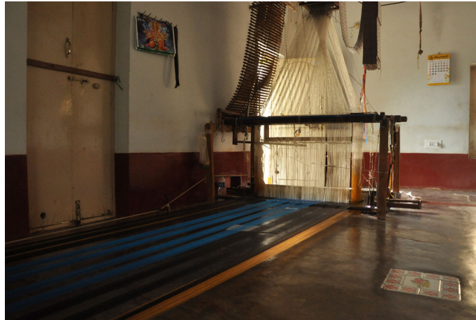
Pit loom is used for saree weaving.
