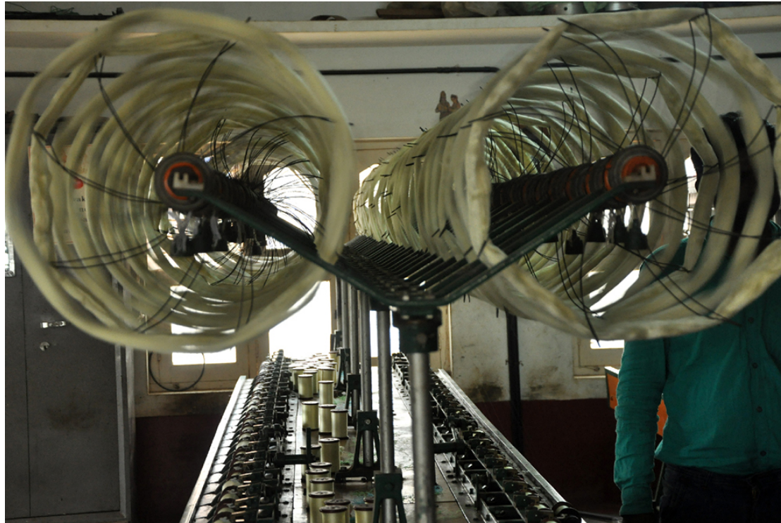
Reeling threads from the winding creels to the spindles.
