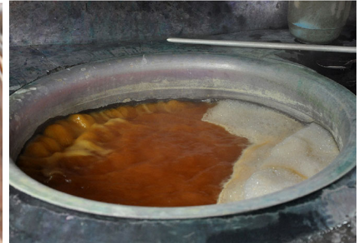
Dry colour, baking soda, and chemicals being added to the boiling water.
