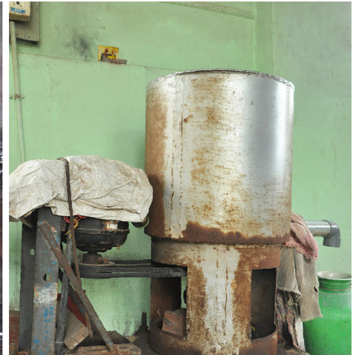
Dryer machine used for removing the excess water.
