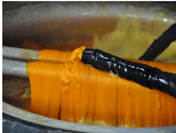
Dyeing process, by tying the portion of yarns by rubber tubes and plastic.
