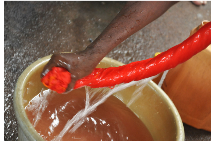
After dyeing the yarns being dipped in water and squeezed.
