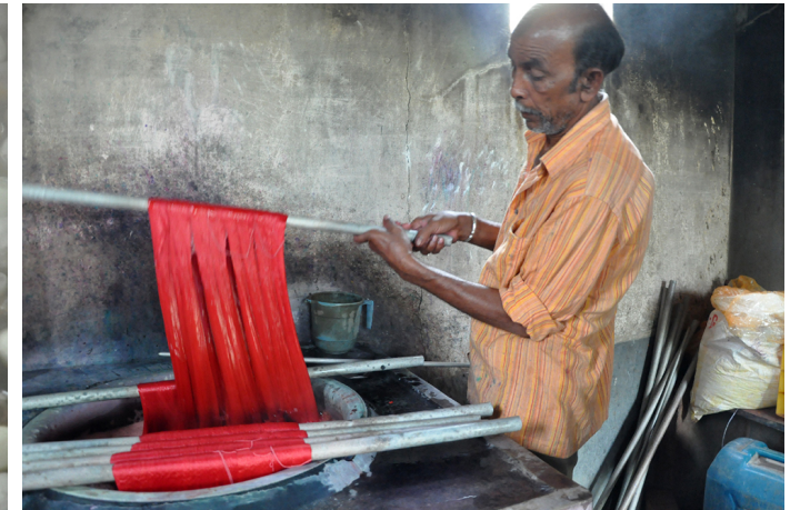
The yarns are rolled to the rod and dipped in the solution during the dyeing.
