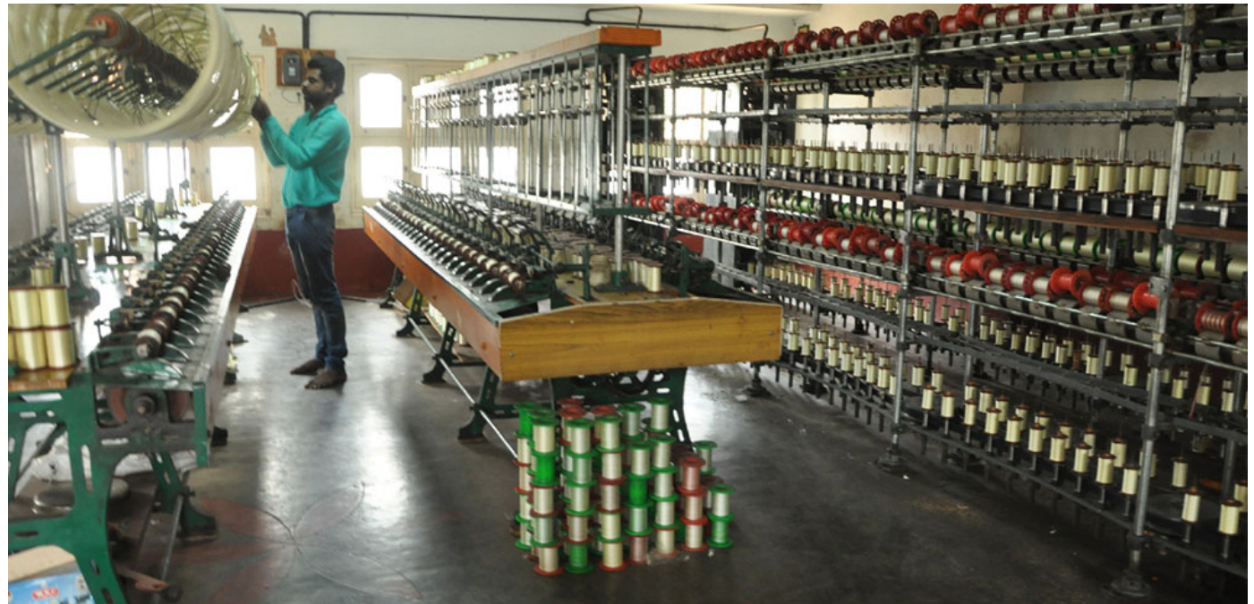
Joining thread from the machine to the spindle by twisting.
