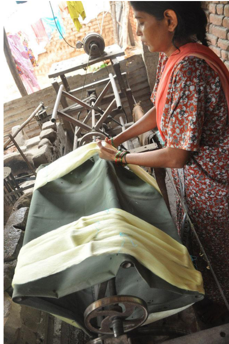
Yarn bundles being removed from the warping machine.
