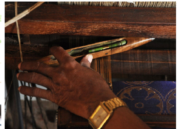
The thread of fly-shuttle is connected to the warp threads, and the shuttle passes through the opening of the warp shed.
