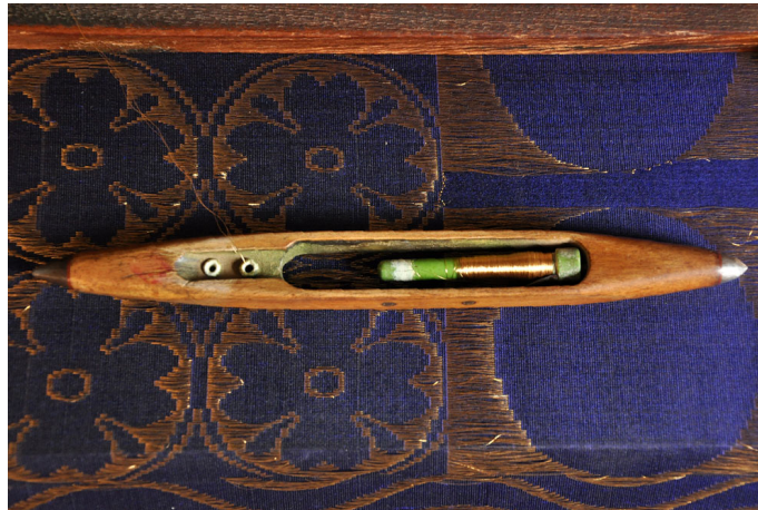
Flying shuttle used for the weft insertion while weaving.
