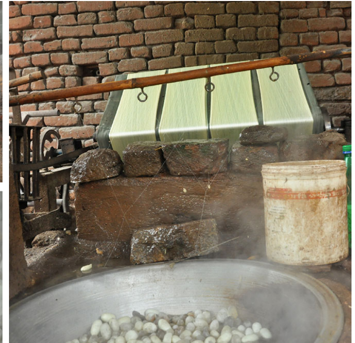
This machine automatically picks the filament from the cocoon and reels it.
