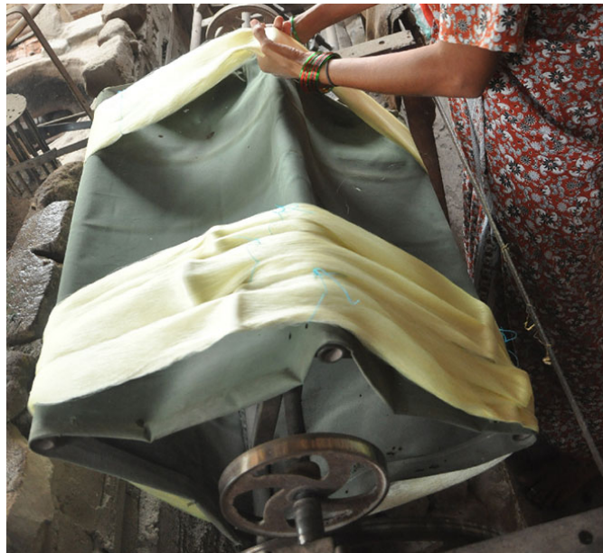
Yarn bundles being removed from the warping machine.
