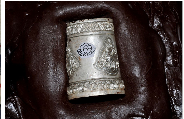
A silver glass is placed on molten lac, which holds it firmly.
