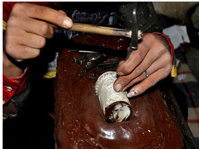
The artisan carves the design with chisel and hammer following the stencil.
