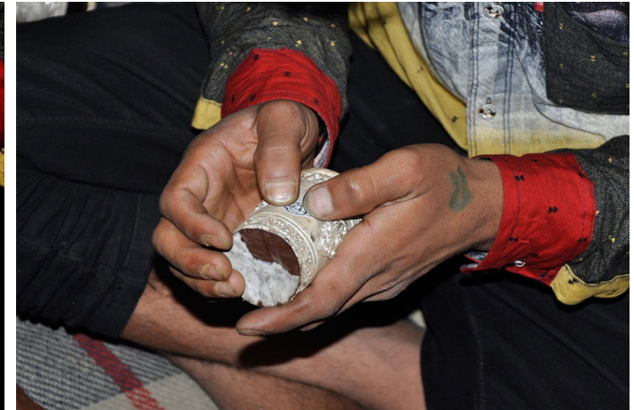
The design stencil is stuck onto the silver plate using adhesive.
