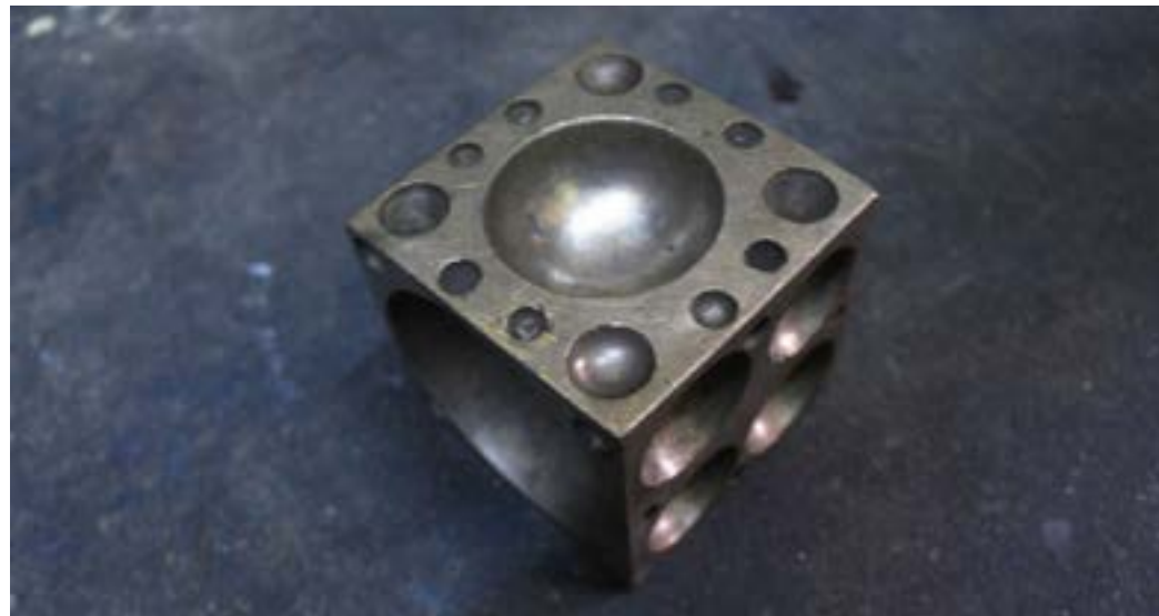
Kansula box is used for making the sheets into curved shapes.
