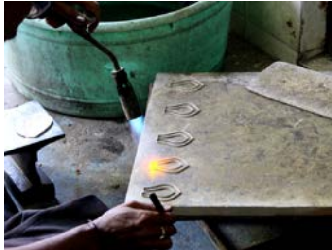
The frame is annealed using heat to add strength to the structure.
