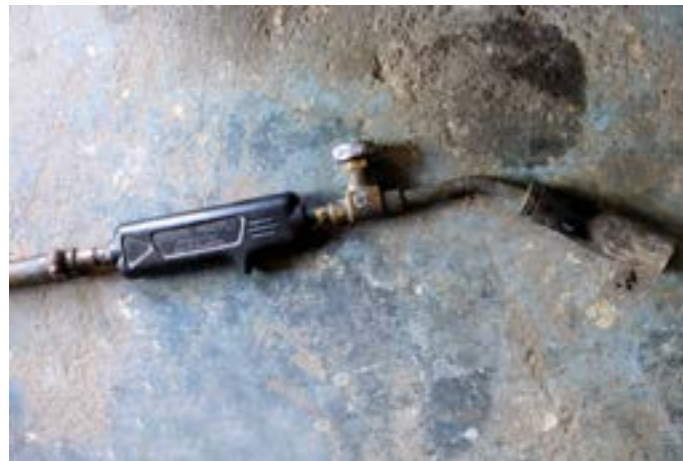
Torch burner is used to heat the silver for shaping.
