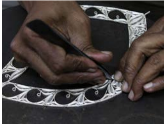
Maskala tools used to fix the wires inside the frame.
