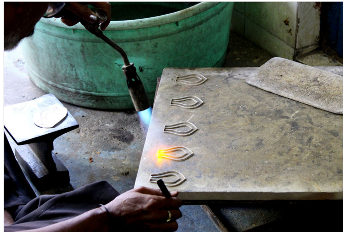
The frame is annealed using heat to add strength to the structure.
