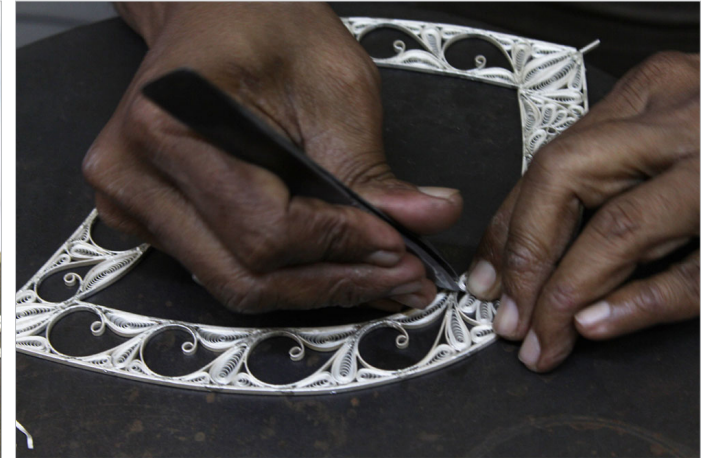
Maskala tools used to fix the wires inside the frame.
