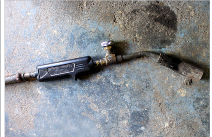
Torch burner is used to heat the silver for shaping.
