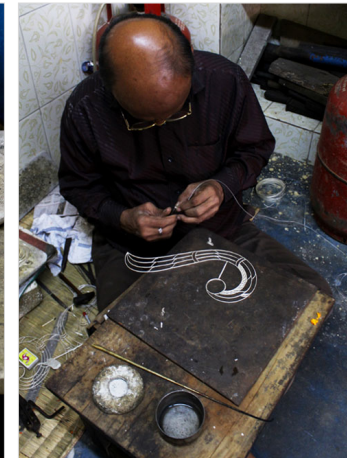
Silver wire is twisted to make a design and inserts in the frame.
