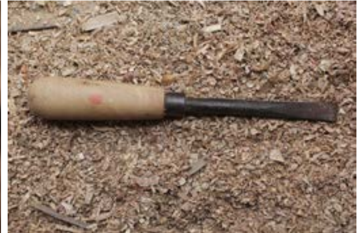
Chaudhara is used for external carving.
