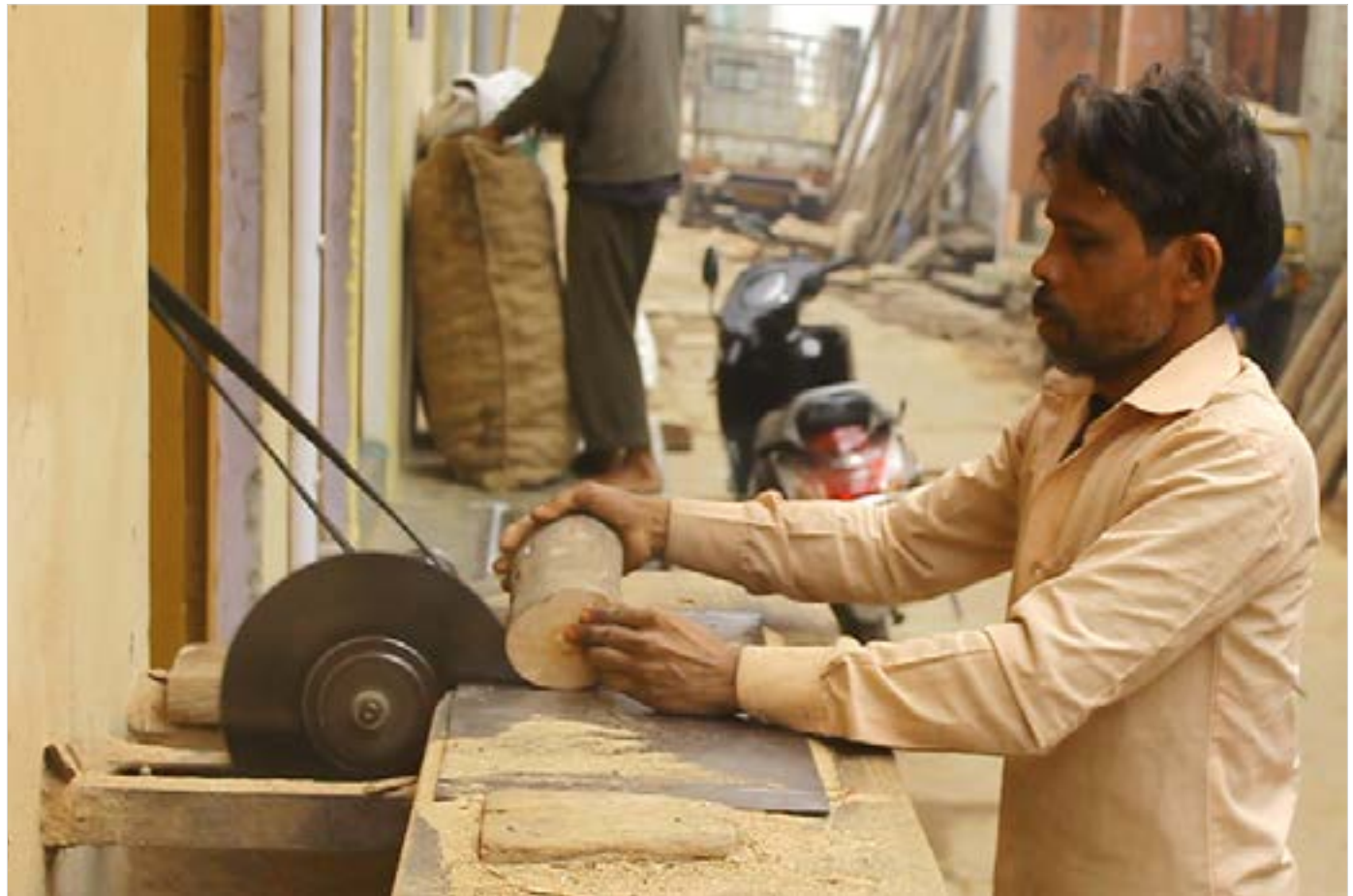
Cutting wooden log in small pieces.
