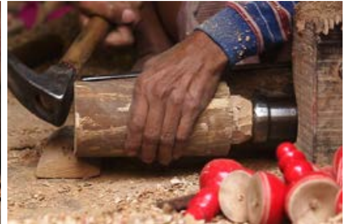
Fixing wooden block in chuck.
