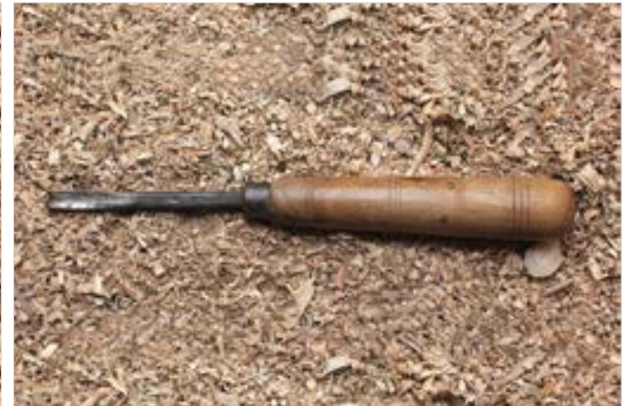
Small Rukhani is used for carving design.
