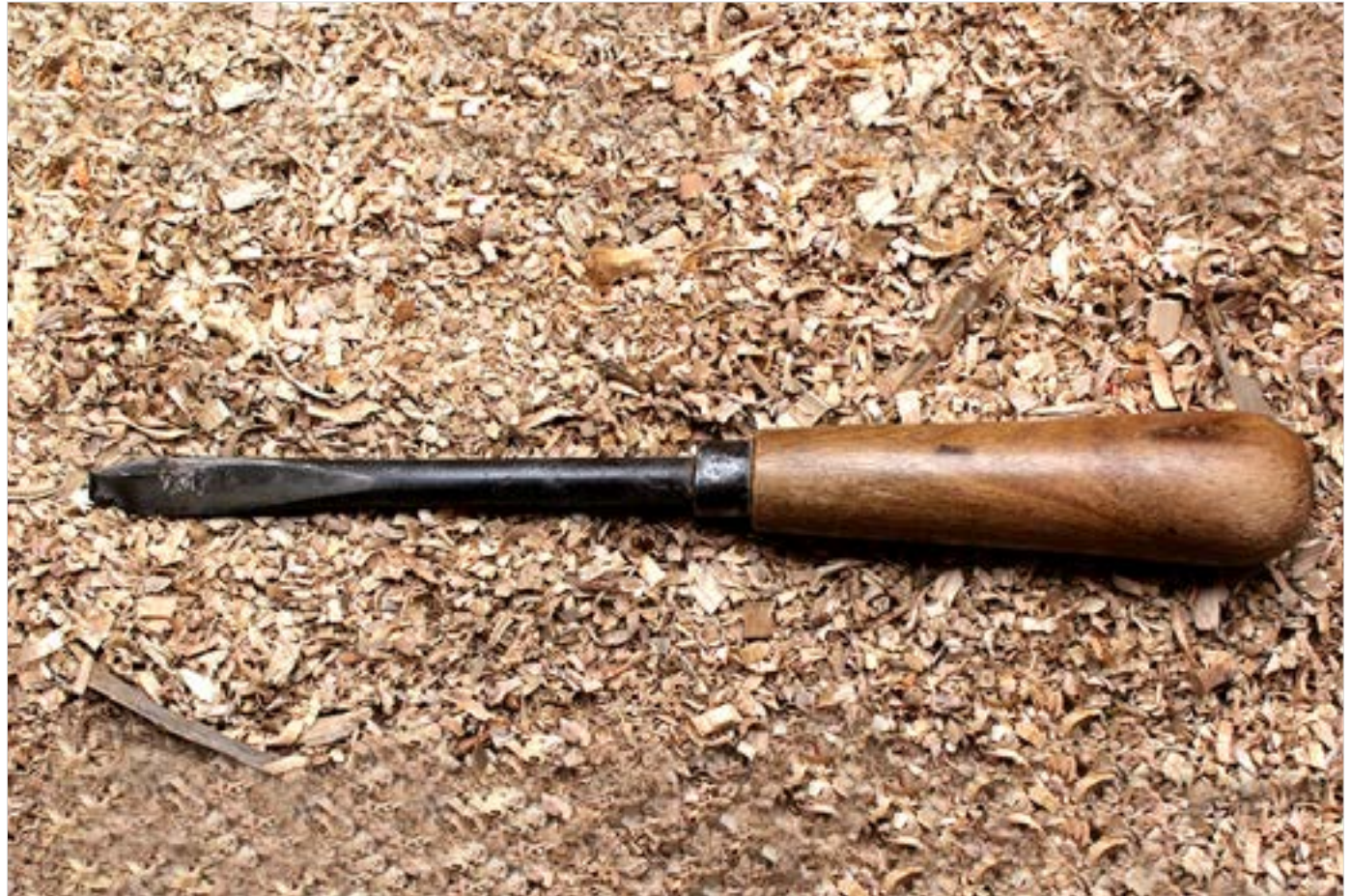
Tripkala is used for fine carving. It has three sharp edges.
