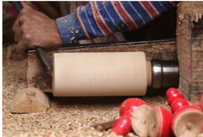
Making cylinder Shape.
