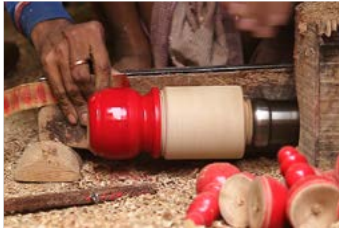
Rubbing with local material to shine the product.
