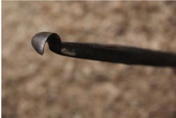
Banki is used for carving the inner part of Sindoora.
