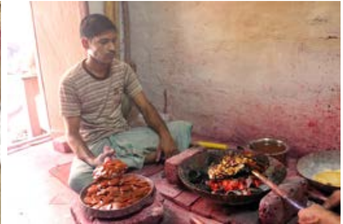
Lacquer is melted using burning coal.
