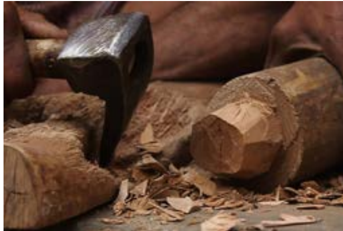
Peeling one side of wooden piece to make it fit for chuck.
