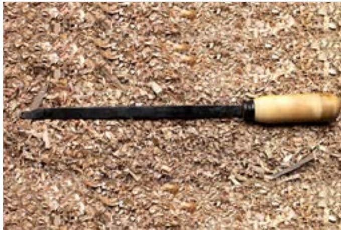
Battali is used for cutting and separating work from the wooden block.
