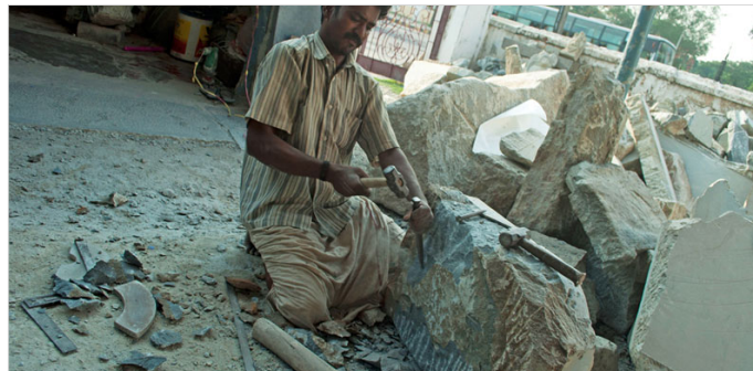
Big block of stone is first roughly cut.
