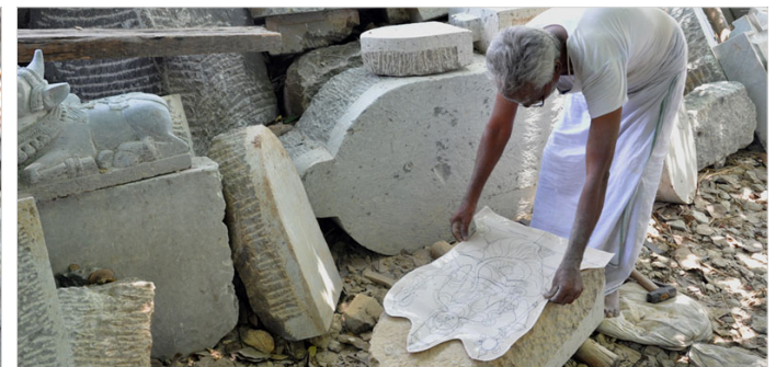
Design reference is placed on the stone to mark the shape.
