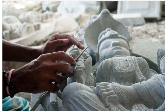
Files are used to give detailed carving.
