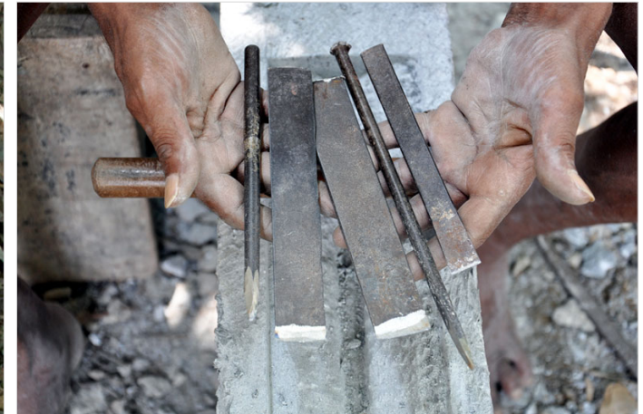
Wide and point-edged chisels used for detailed carving.
