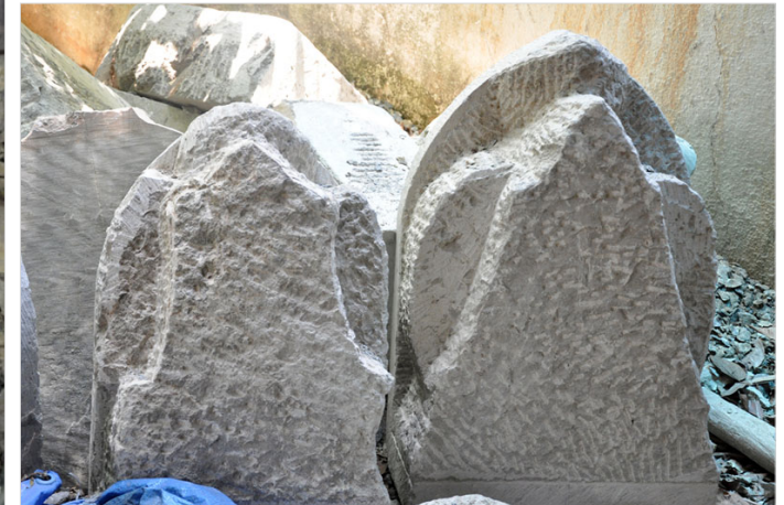
The unwanted portion of the stone is removed.
