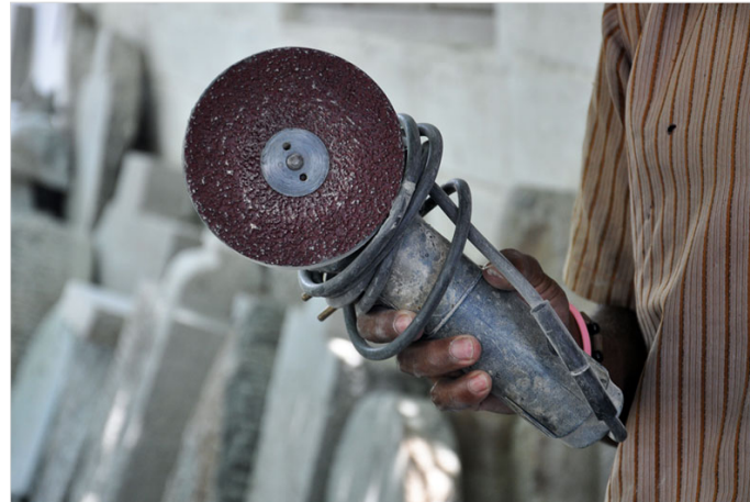
Automated tool used to smoothen the outer surface of stone.
