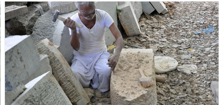
The rough outer texture is removed by carving.
