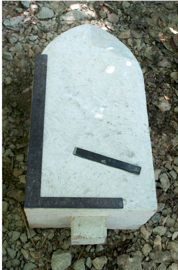
Scale is used to mark dimensions.
