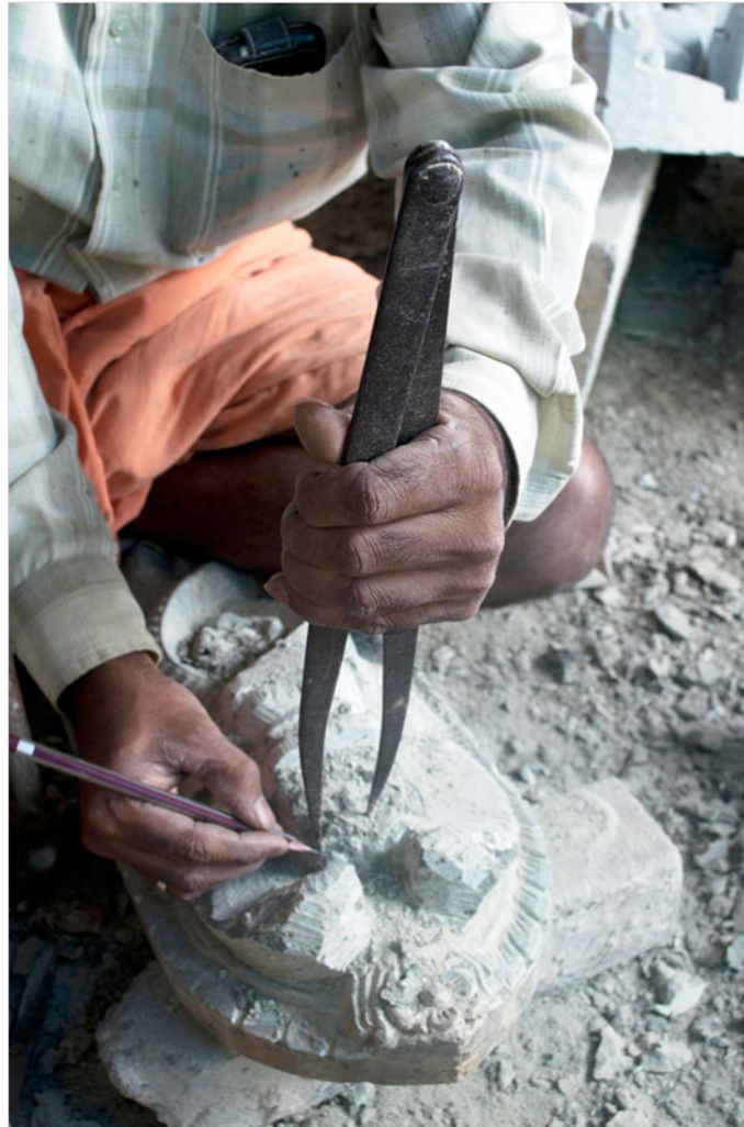
Dimensions of the face are being marked on the stone.
