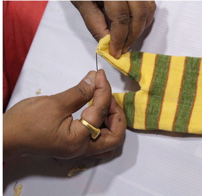
After stitching, the sock is turned back to tie the knot at the corners.
