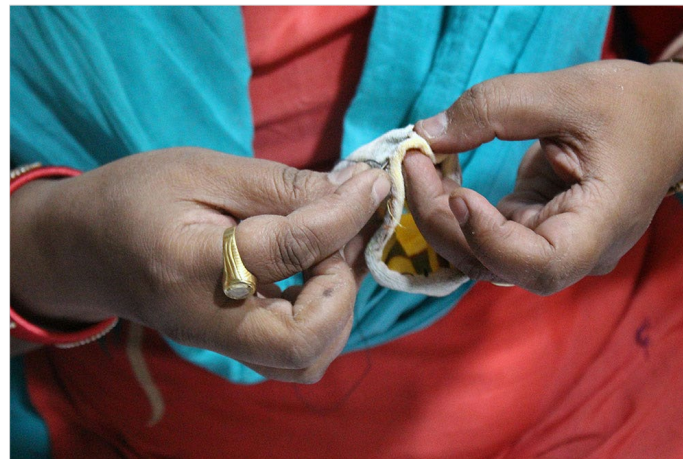
The rest of the sock fabric which was cut at the start is being sewed together through the edges inside out.
