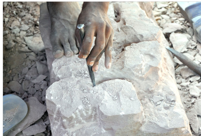
Major carving is done using large chisels.
