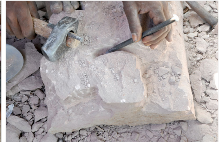
Shapes obtained through the process of hammering and chiseling.
