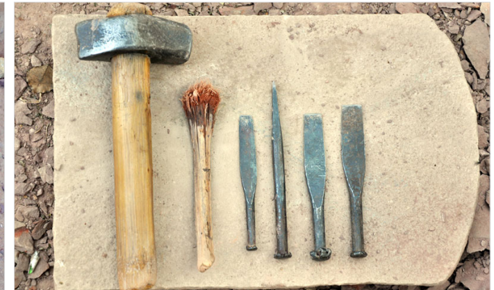
Stem of coconut tree used to clean the stone during carving.
