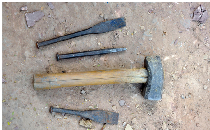
Hammer and chisels are the main tools used in stone carving.
