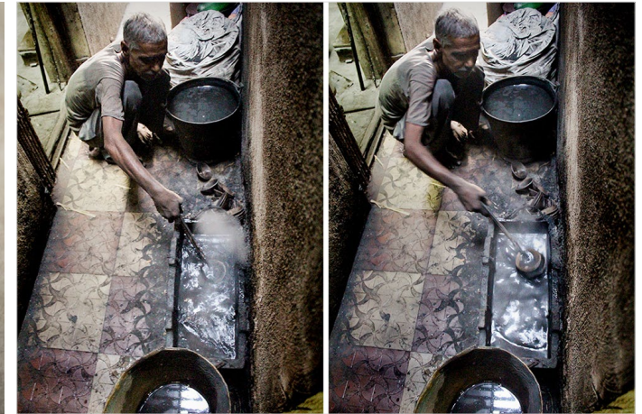
Artisan dipping the cymbals into the water first to make it cold and then into a specific chemical for good quality sound.
