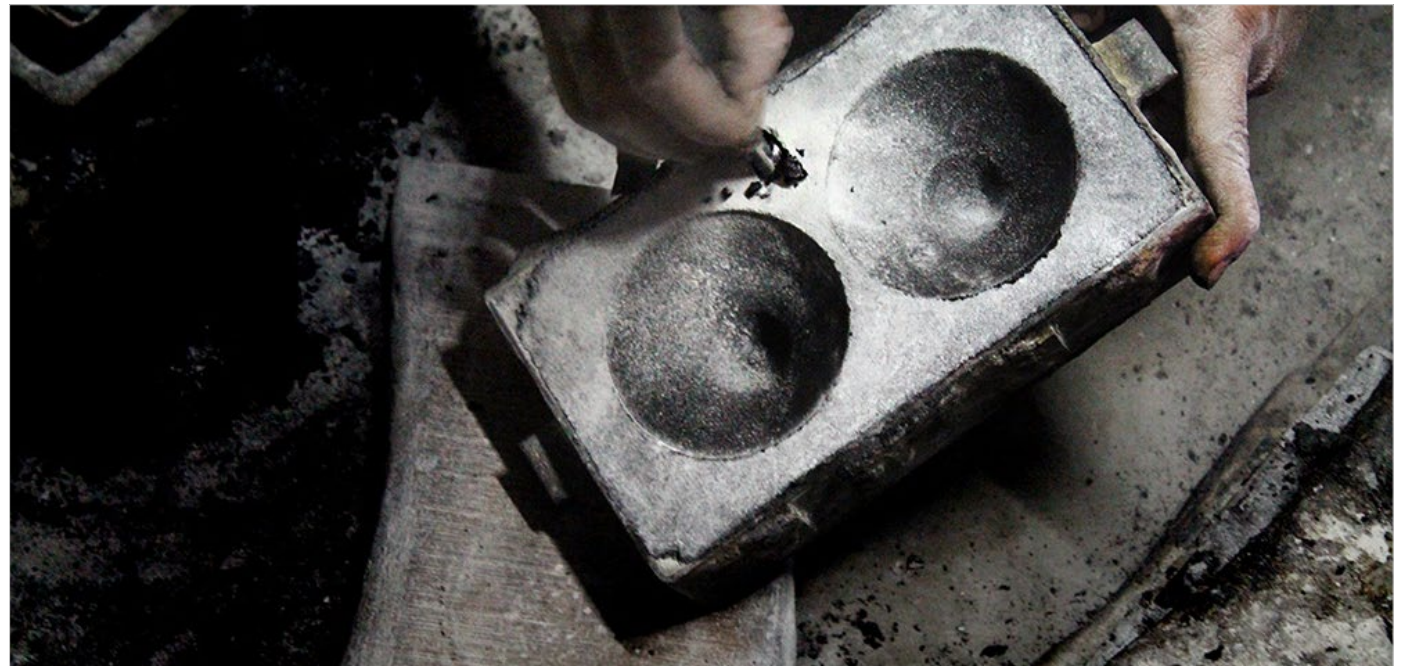
Artisan making a hole in the mold using a small chisel.
