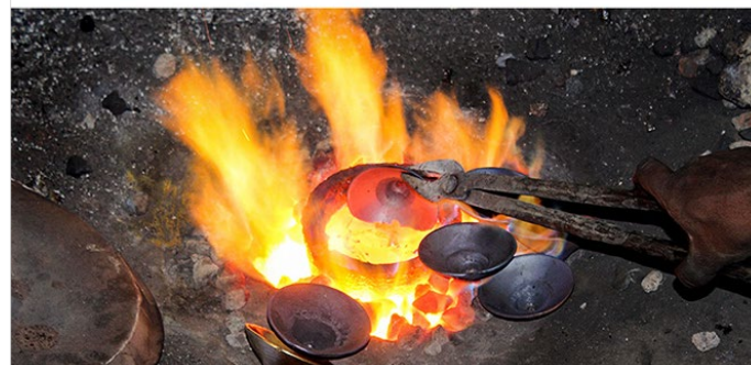
Old bronze wires and pieces being dropped inside the crucible for melting.
