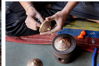
Scraping is done to the topmost part of the cymbal as well.
