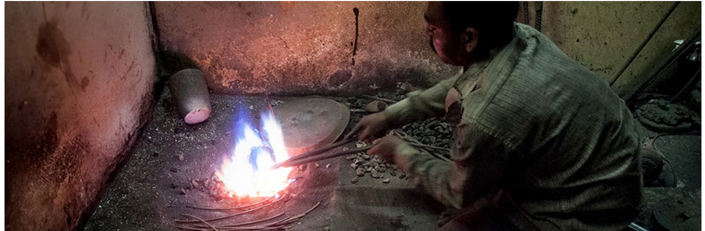
Artisan placing crucible inside the fire pit.
