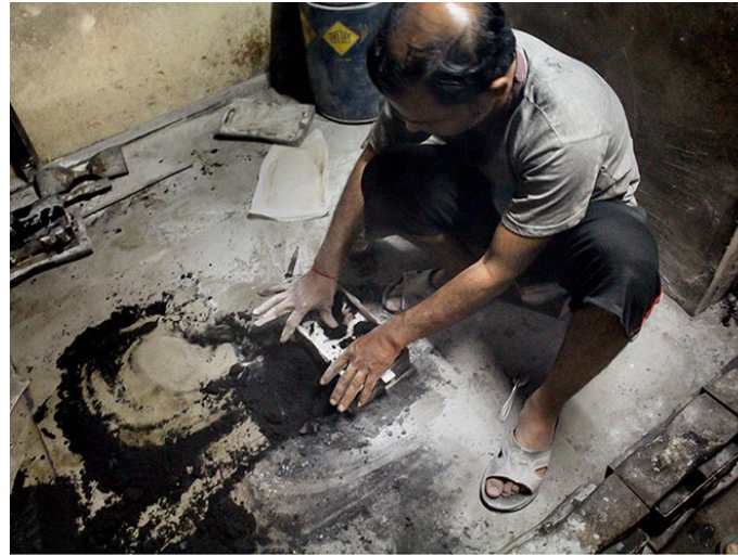
On the second layer mold, the backside of the cymbals is printed.
