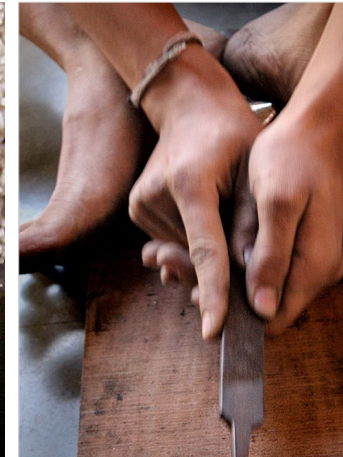
Scraping is done to the topmost part of the cymbal as well.
