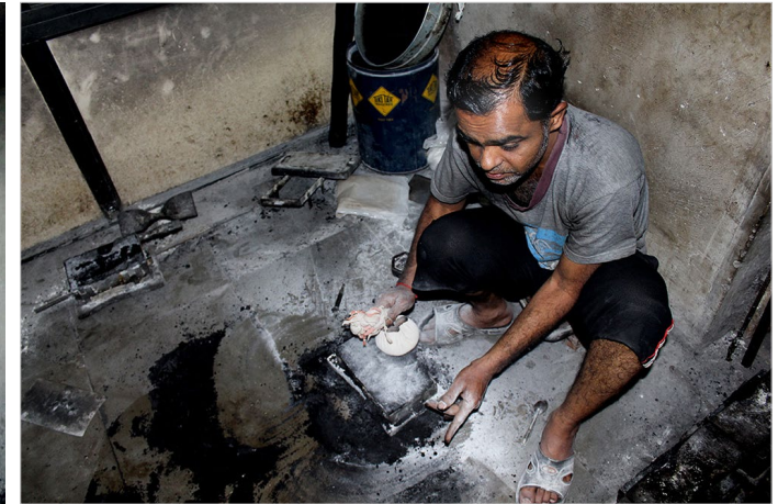
Artisan sprinkling wheat flour on the top surface of the stuffed mold.
