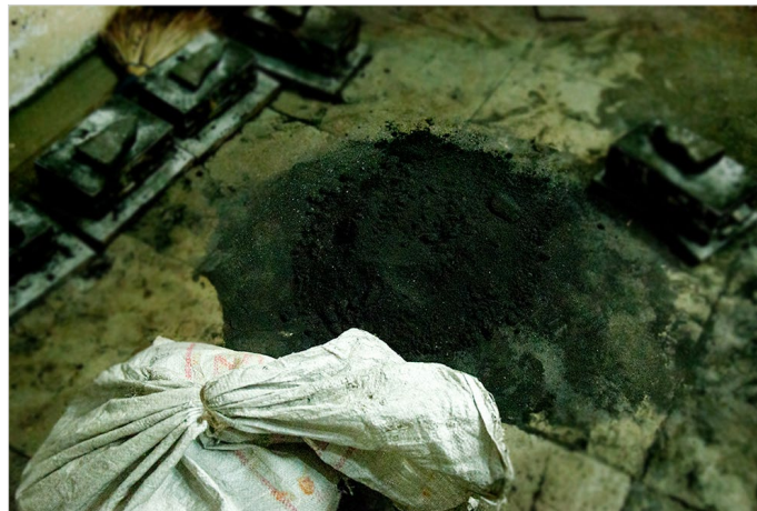
Black sand, a mixture of bituminous powder and sharp sand that is stuffed inside the iron mold after filtration.
