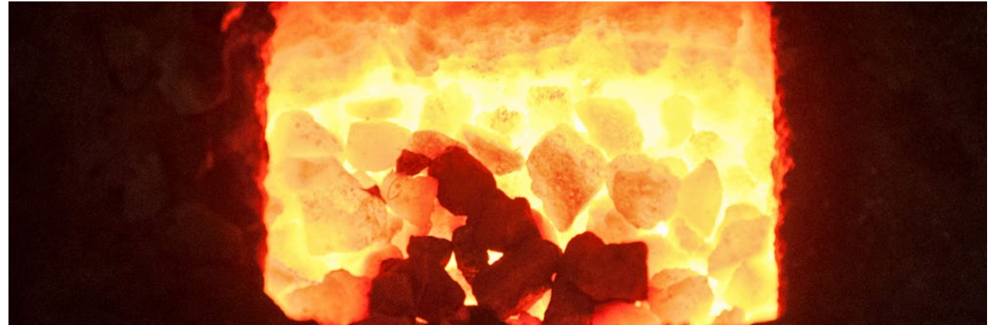
A fire pit that burns at around 1200°C temperature to melt bronze pieces.
