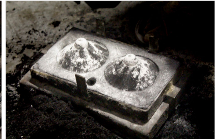
On the second layer mold, the backside of the cymbals is printed.
