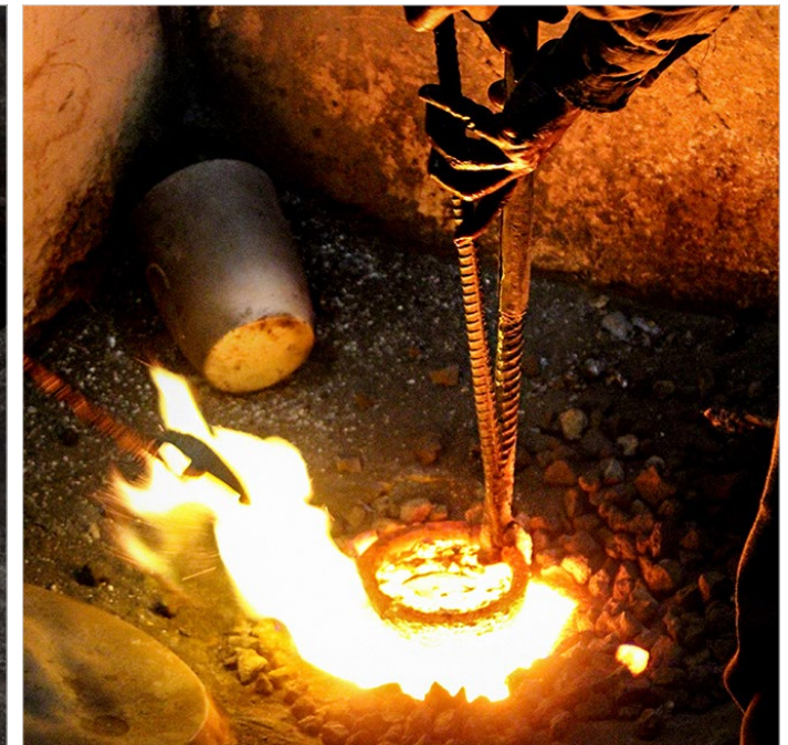
Artisan raising a crucible filled with molten bronze from the fire pit using an iron holder.
