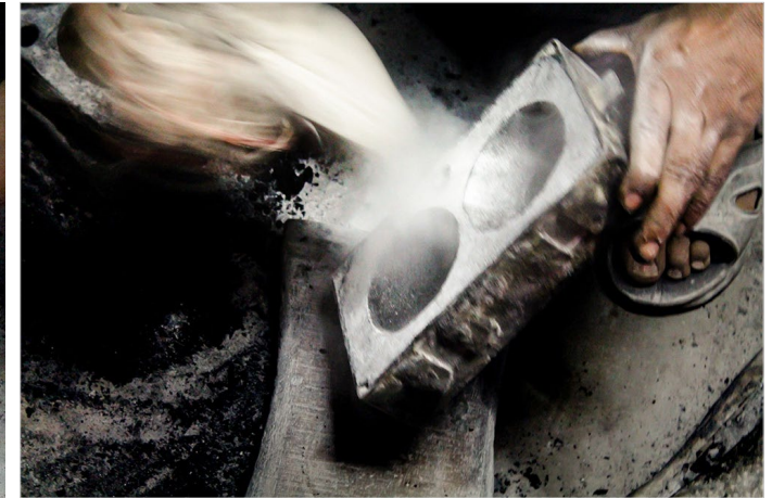
The bronze cymbals are removed from the mold and the mold is then sprinkled with flour.
