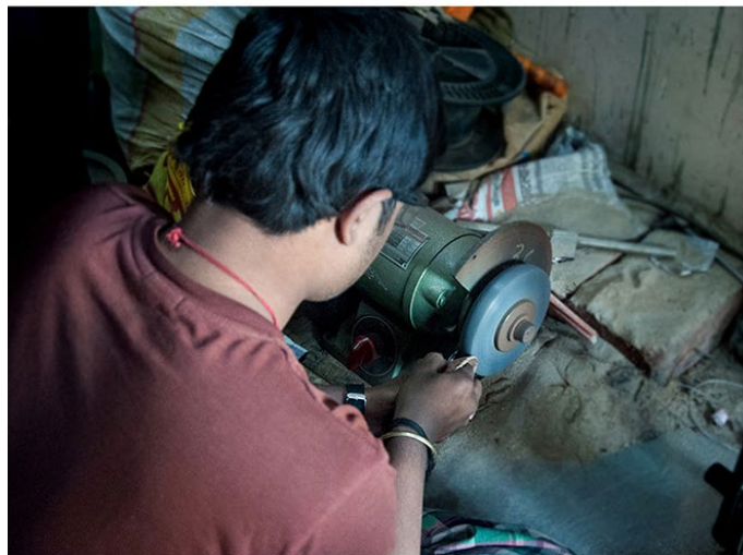
Artisan grinding the raw cymbals with power sander for smoother surfaces.
