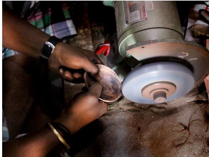
Cymbal being fixed on a lathe turner.
