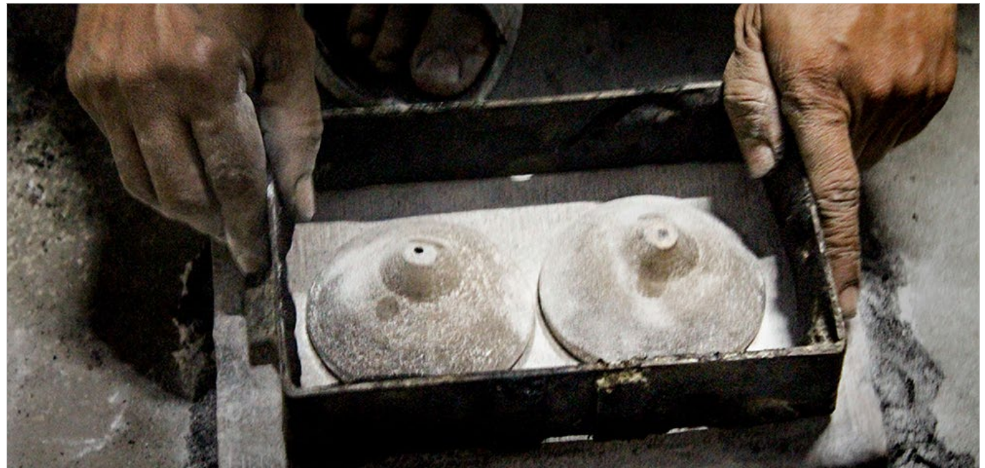
The first layer mold being fixed on the cymbals and wood piece.
