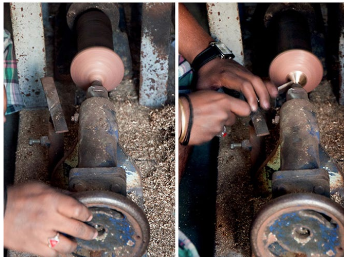
Artisan scraping certain unwanted areas of cymbal using a file scraper.
