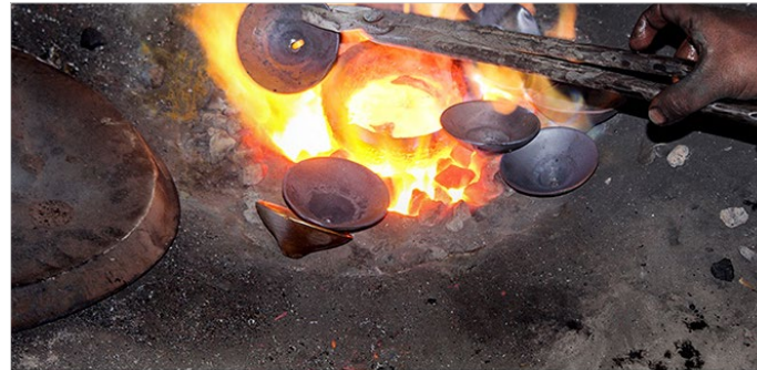
Artisan placing crucible inside the fire pit.
