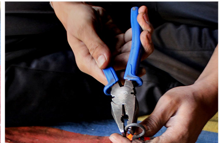
A cutting plier used to bend iron nails as per the required shape.
