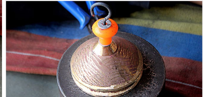
Artisan bending the sharp edge of the nail into a circular shape using a cutting plier.
