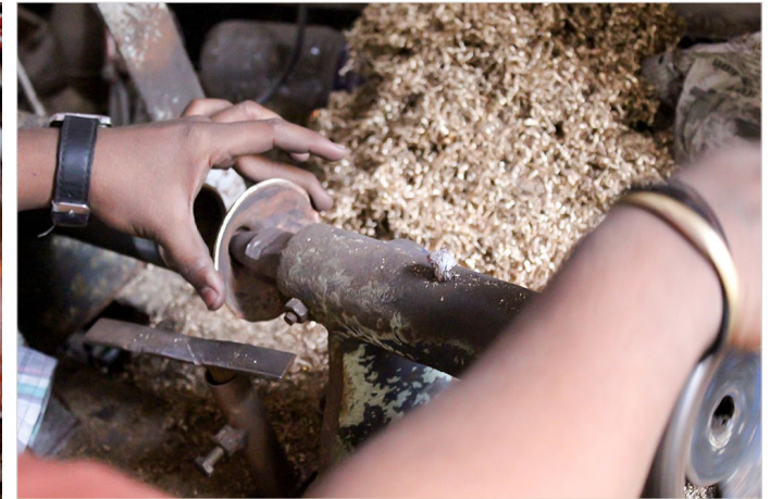
Cymbal being fixed on a lathe turner.
