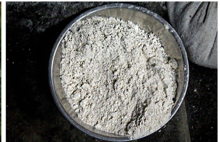
Wheat flour used to apply on the black sand mold to free the casting easily from the sand.
