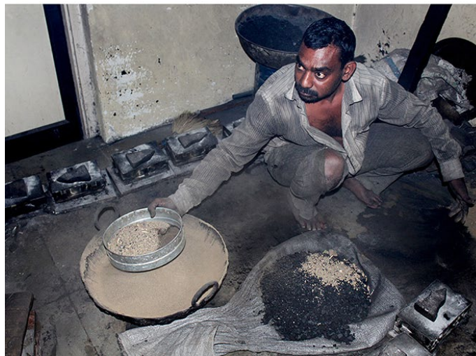
Artisan filtering the hard particles of bituminous powder and sharp sand together using a sieve.
