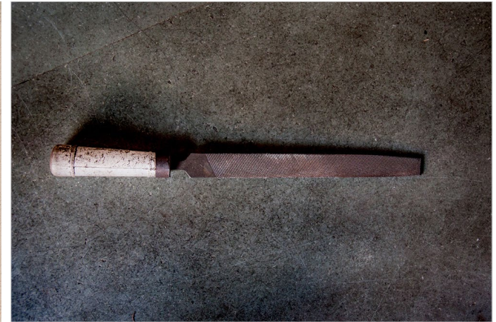
A rectangle file is used to smoothen the outer surface of the cymbal.
