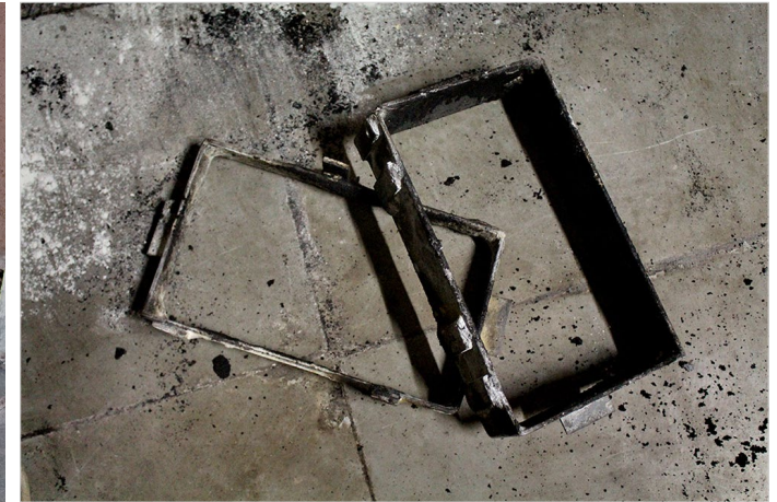
Iron molds used for casting the cymbals.
