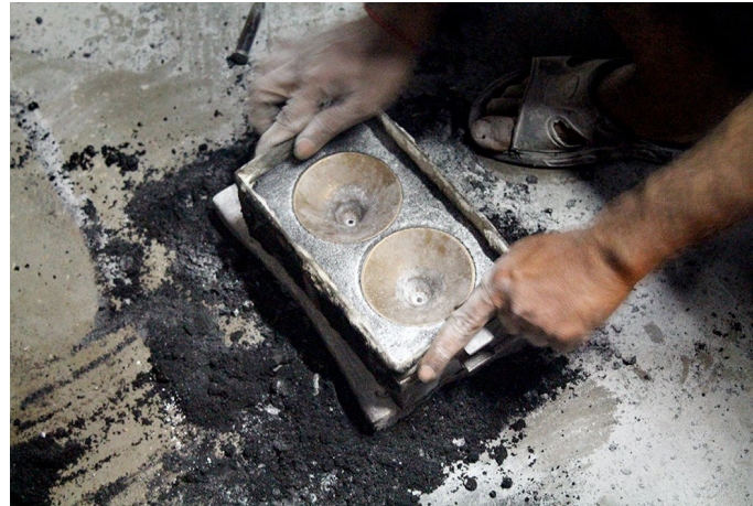
The mold is flipped upside down to check the front part of the cymbals.
