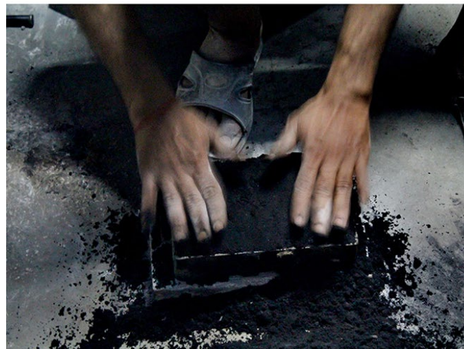
The black sand is stuffed inside this mold.
