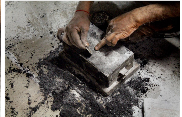
Artisan using a steel spoon to make a hole in the second layer mold.
