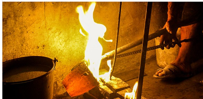
The molten bronze is poured into the mold through a hole on it.
