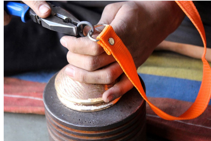
A strap being fixed into the circular-shaped nail and tightening them without leaving a gap.
