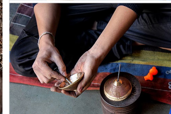
Artisan fixing iron nails to the holes made on cymbals.
