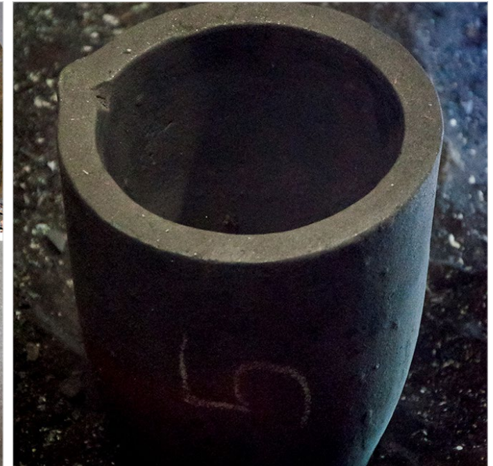
Crucible of clay in which bronze pieces are placed before exposed to fire.
