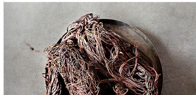
Bronze pieces and Copper wires are the main raw materials to make cymbals.
