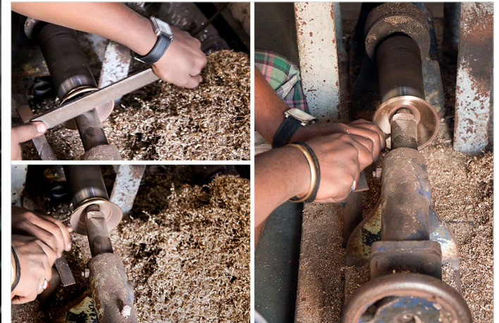
A rectangle file is used to smoothen the front part of the cymbal.
