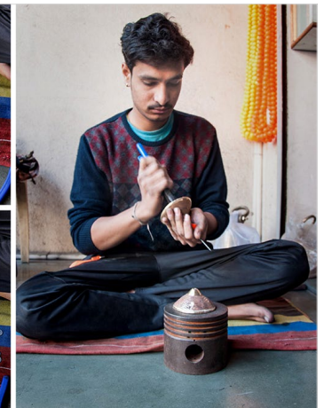
Artisan fixing iron nails to the holes made on cymbals.
