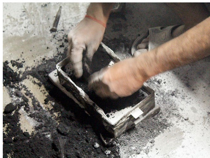
Artisan filling the black sand on to the second layer mold.
