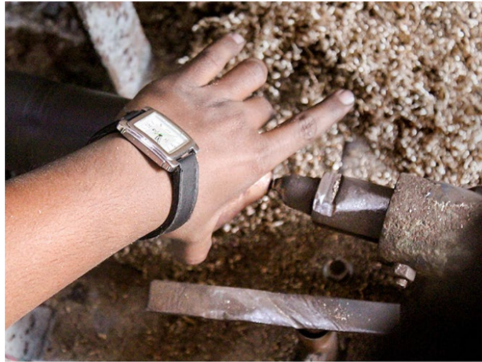
Scraping is done to the topmost part of the cymbal as well.
