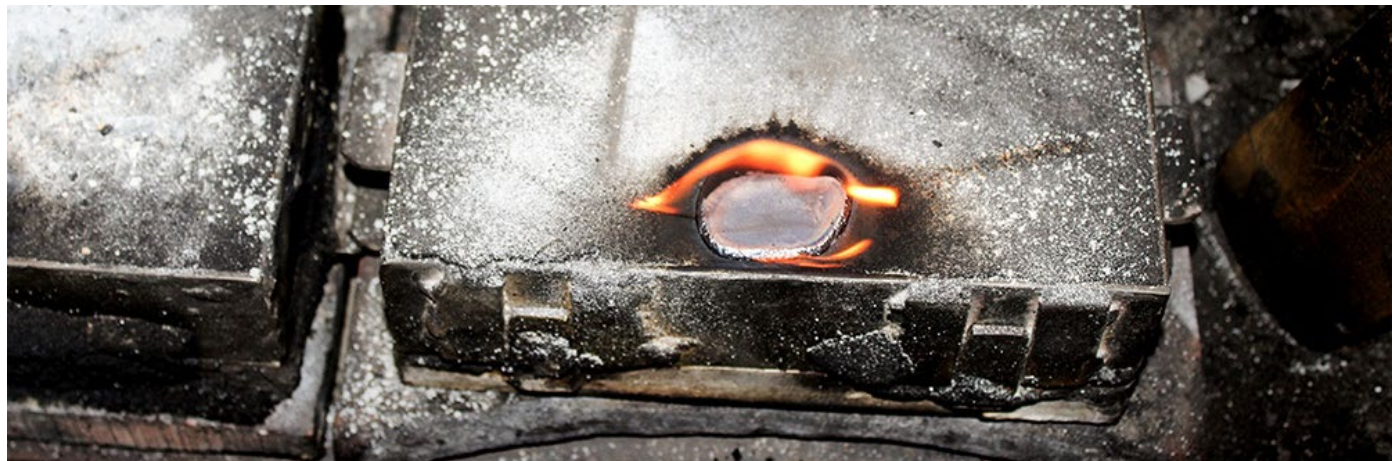
The mold is left for cooling after the molten bronze is filled in.
