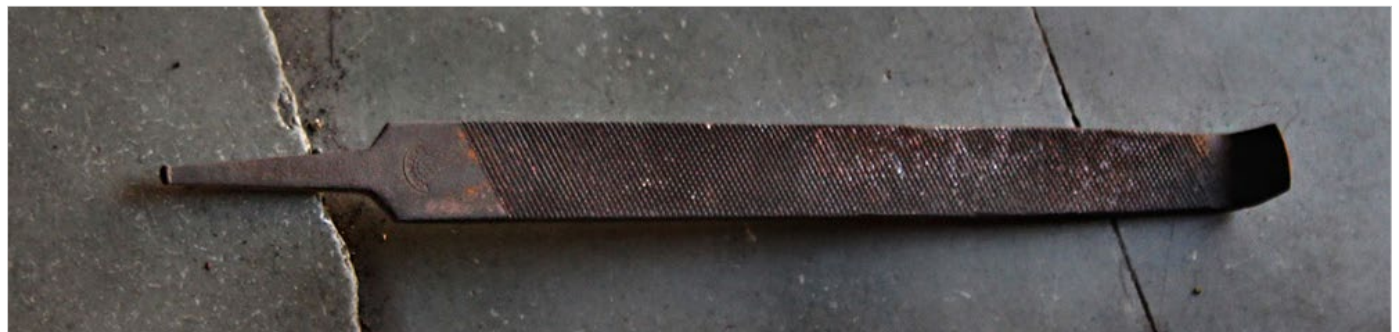
File scraper used to scrape out roughness from the cymbals.
