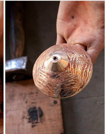
Scraping is done to the topmost part of the cymbal as well.
