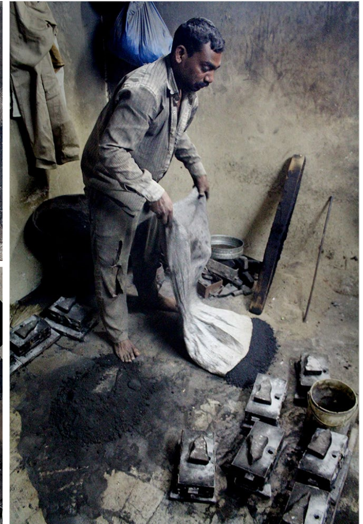
The mixed black sand being dropped from a polymer bag onto the floor.
