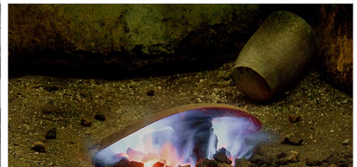
A bronze plate covers the top of the crucible placed over the fire pit to absorb more heat.
