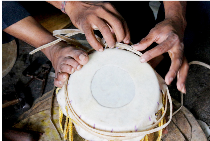
Leather strips are added between the twisted strips to make pudi or drum head.
