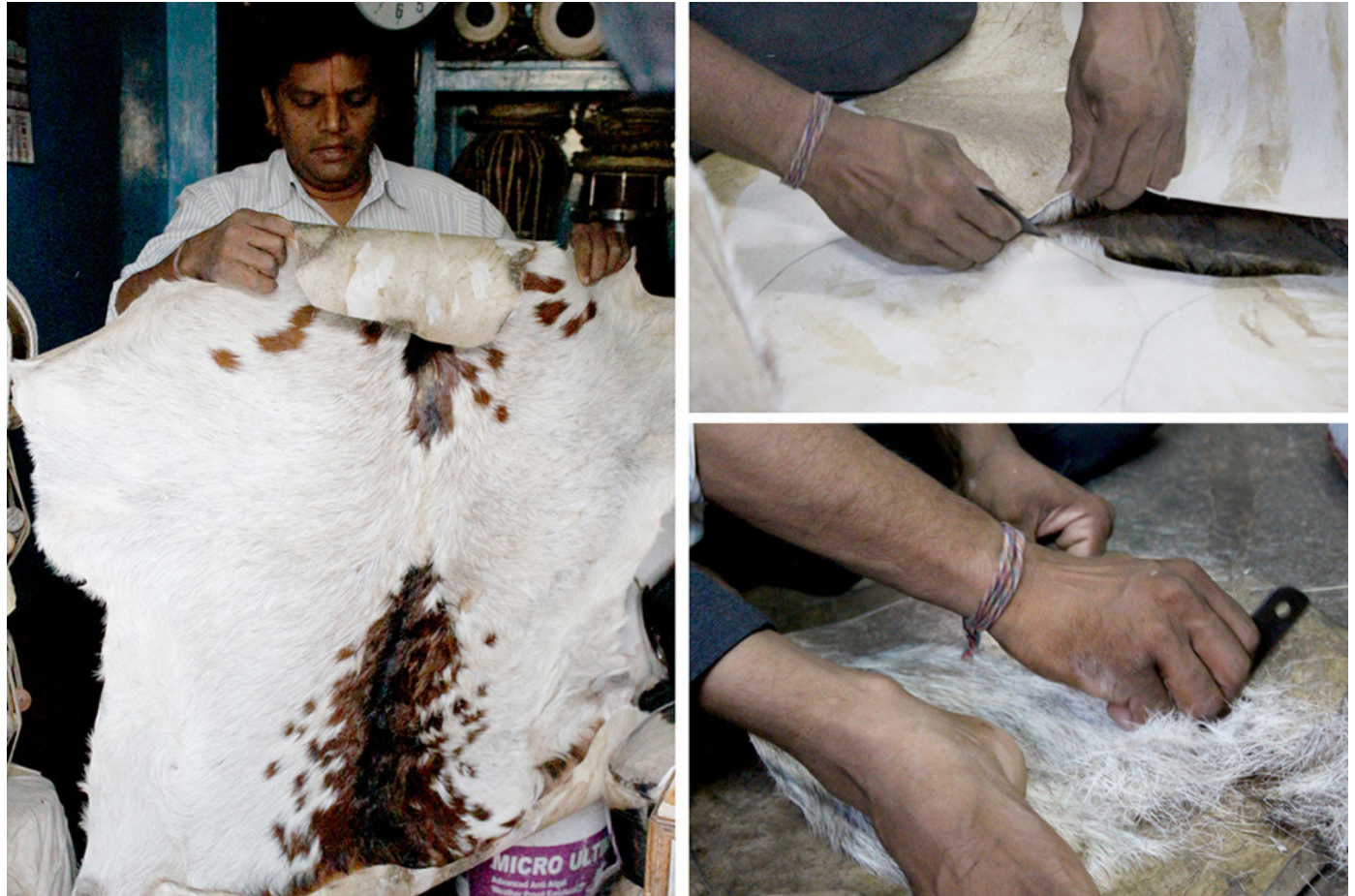
A selected goatskin is cut and the unwanted layer is removed by using sharp tool.
