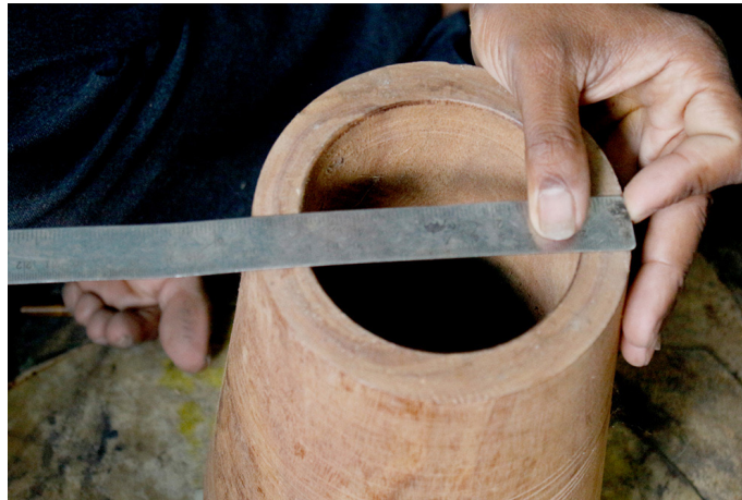
Measuring the wooden body of the Dayan using metal scale.
