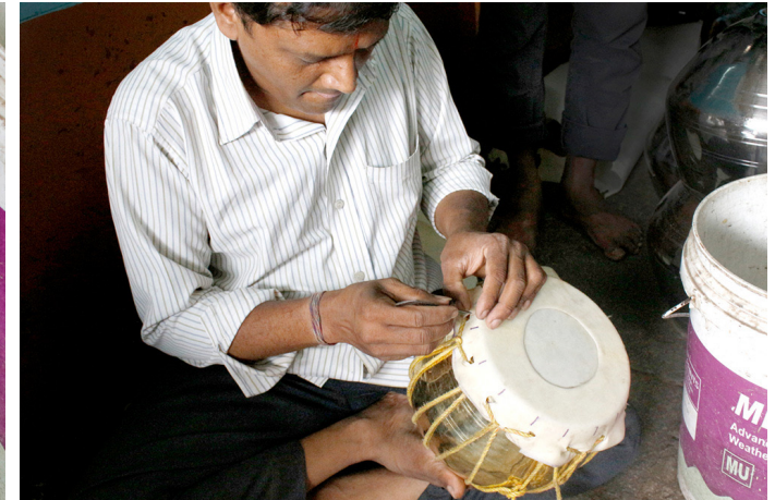
Sharp tool is used to make small slits for lacing.
