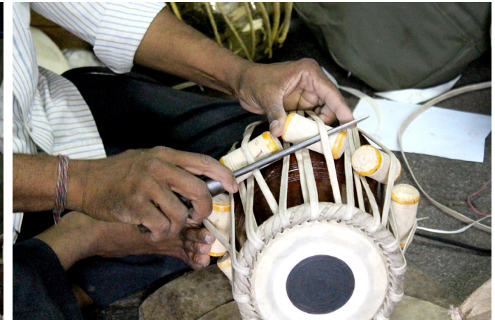
The 'gatta', made of wood is added between the leather strips for tuning.
