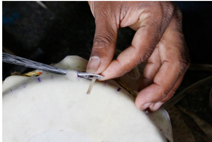
The edges of the leather strips are cut to obtain a thin edge.
