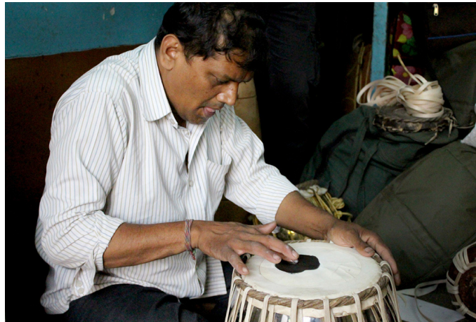
Applying syahi masala at the center of the pudi or table head.
