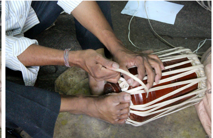
The edges are again weaved for the stiffness and endurance.
