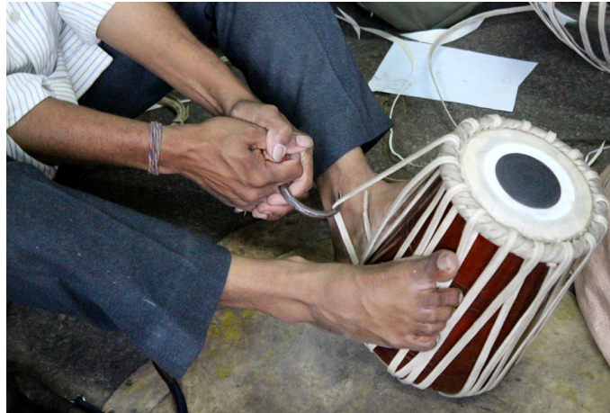
Leather strips are tightened by pulling them with the help of customized hooks.
