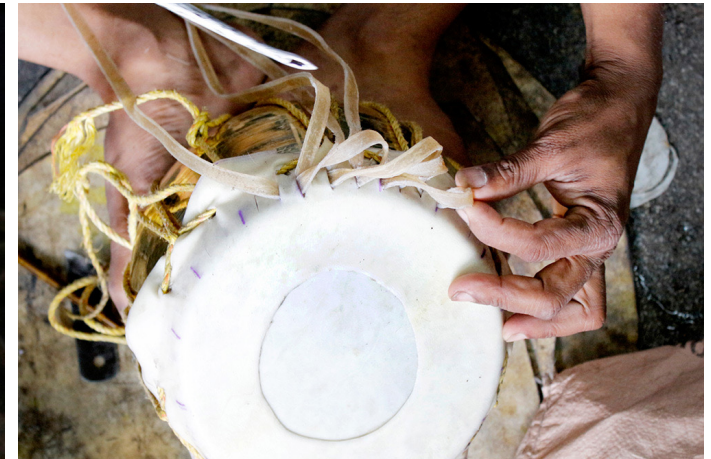
Leather strips are inserted through the slits and twisted and then pulled out.
