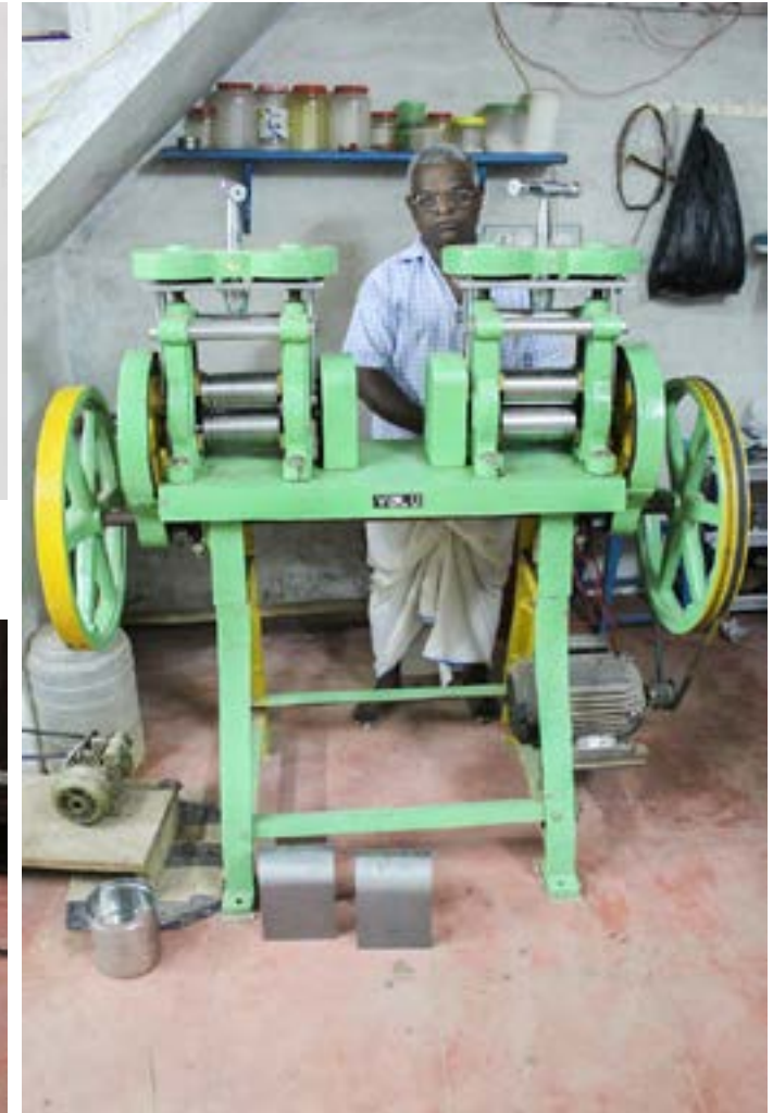
A rolling machine is used to flatten the silver strips to the required size and thickness.
