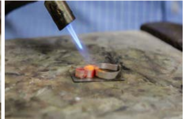
The silver is soldered to the base piece.
