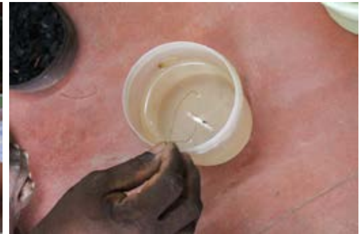
The silver is soaked into nitric acid.
