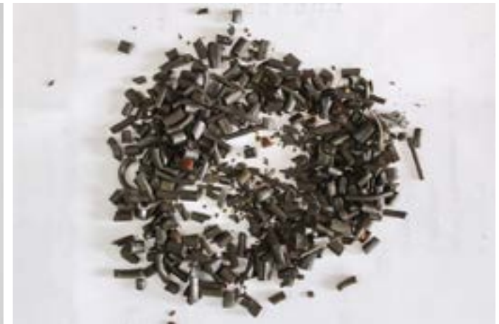
A mixture of lac and black stone powder is used to stick the pearls.
