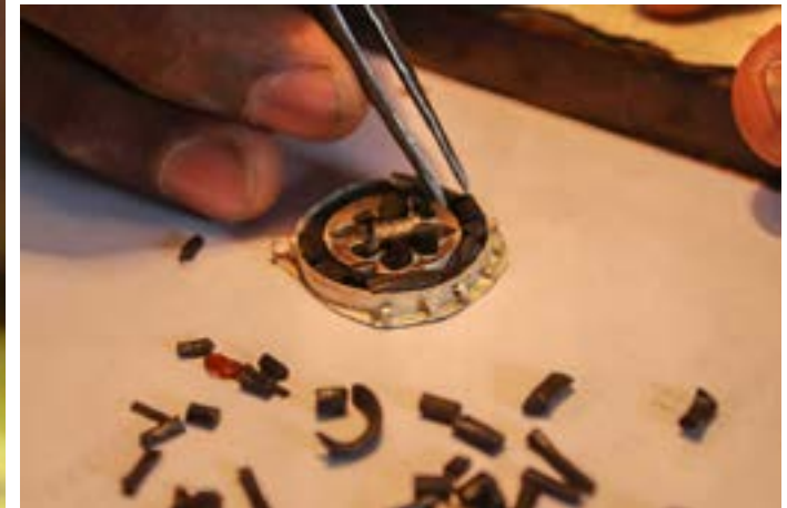
The lac mixture is filled into the design.
