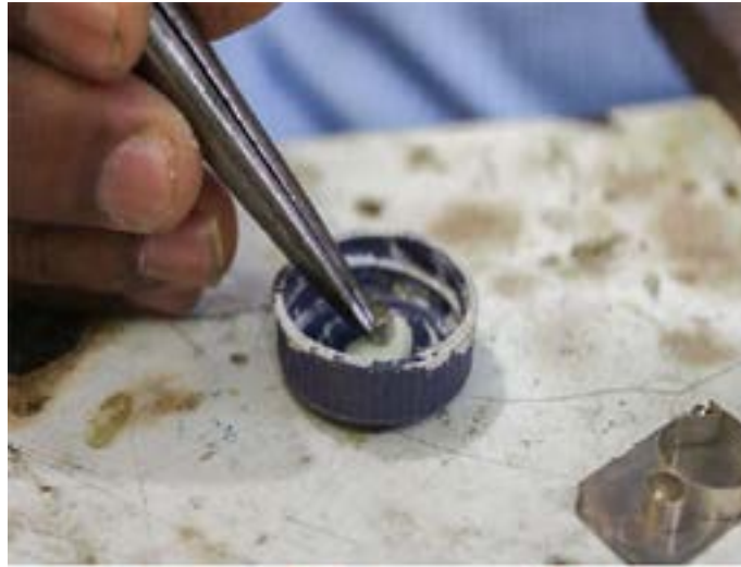
The silver is soldered to the base piece.
