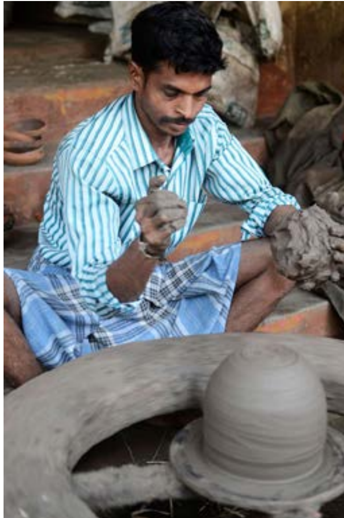
Clay dough is placed in the center of the potter's wheel. The clay dough is being shaped.
