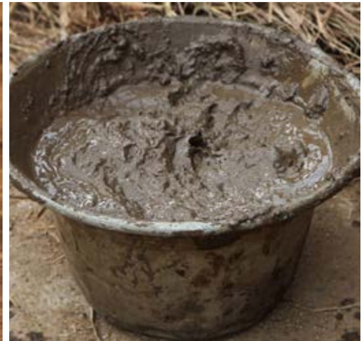
Mixture of clay, sand and water used in baking process.
