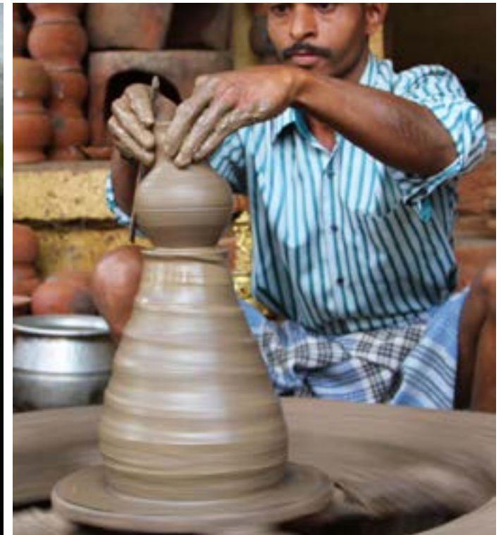
Mouth of the pot is being shaped.
