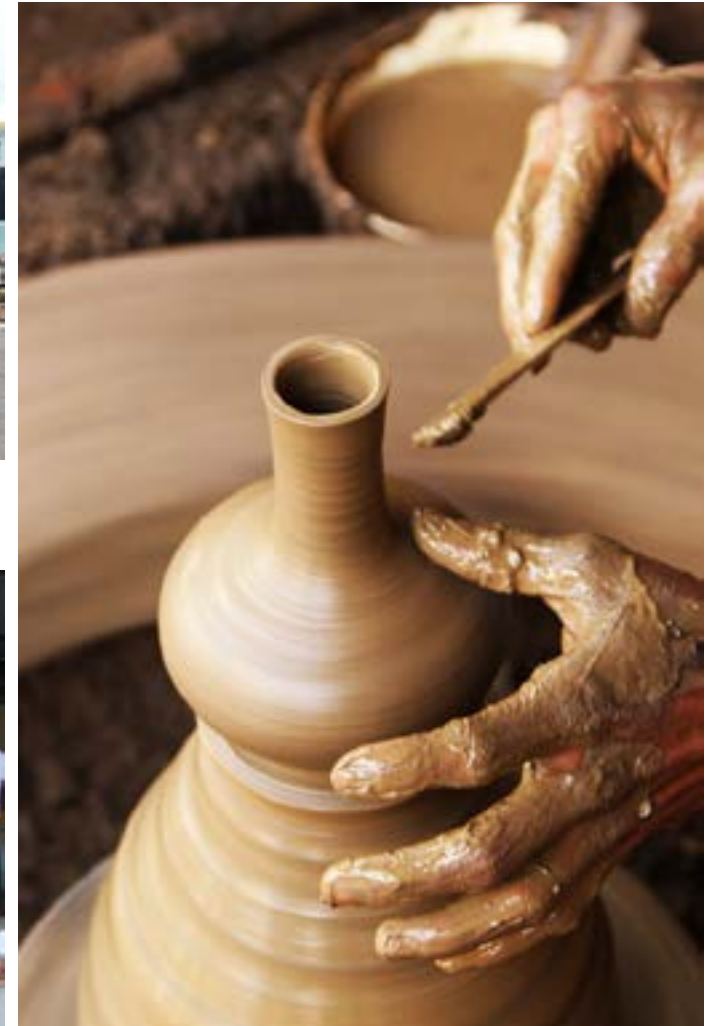
The surface of pot is smoothed using wooden filer.
