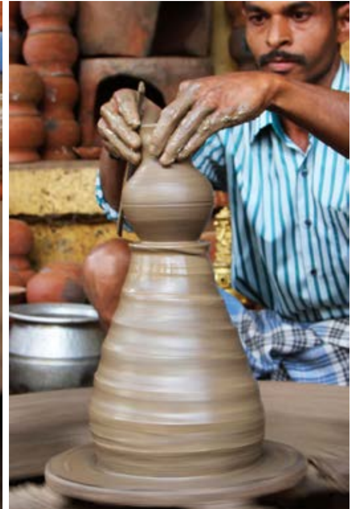
Wooden stick is used to make the surface even.
