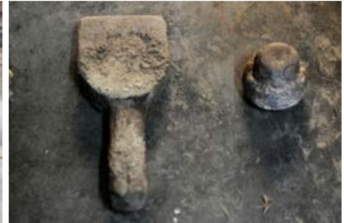
Wooden mallet is used to beat the product until proper shape is acquired after baking.
