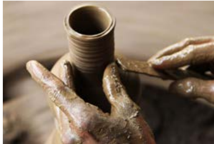
Neck of the pot is being shaped.
