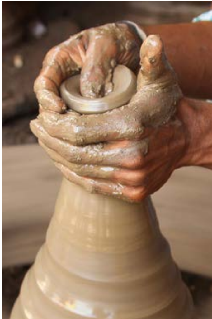
The mouth of the pot is being shaped.
