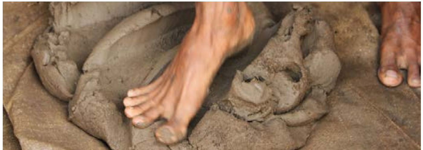
Clay is thoroughly kneaded to enhance its inner flexibility.
