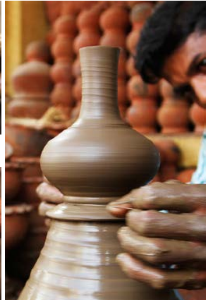
The finished product is removed from the potter's wheel using thin thread.
