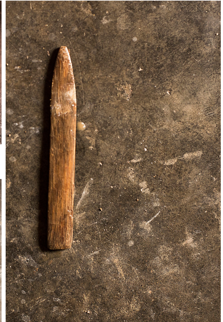
Tool made up of bamboo, which is used in detailing and shaping of terracotta idols.
