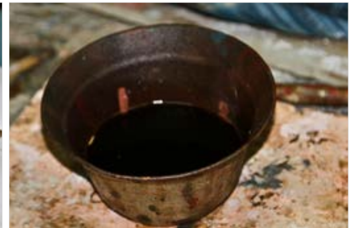
Solution of grease and kerosene is applied on the idol before putting the mould paste to avoid smudging of the design.
