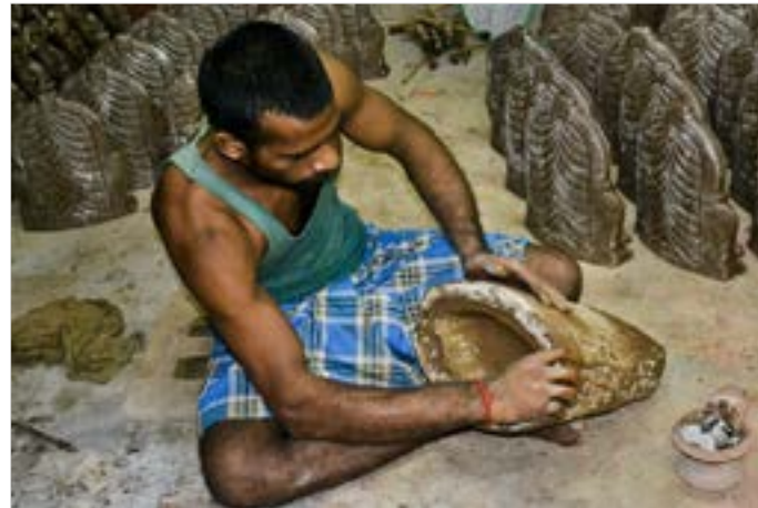
Base of idol is made hollow.
