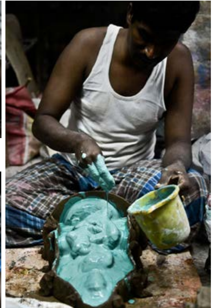
The first layer of the mould consists of casting powder solution.
