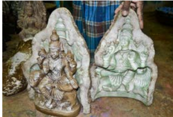
Image showing the detail design impression made by the mould on the clay.
