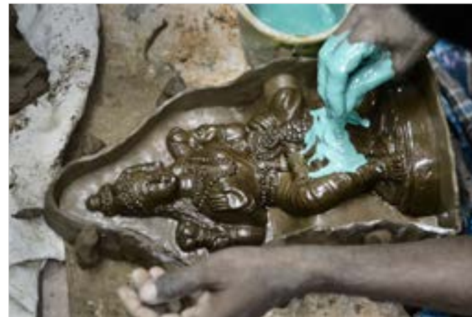
Artisan applies the casting paste on the idol.
