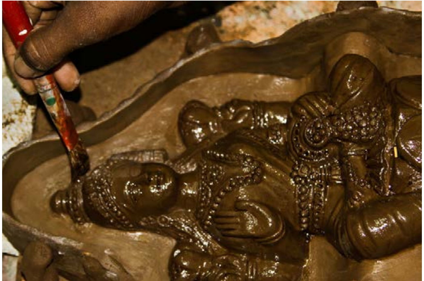
Mixture of grease and kerosene is applied to avoid smudging of design.
