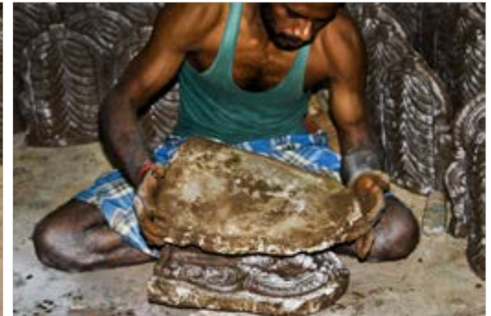
Artisan removes the prepared idol from the mould.
