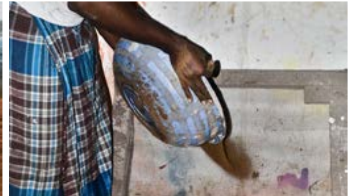
Clay is filtered to remove lumps and other impurities.
