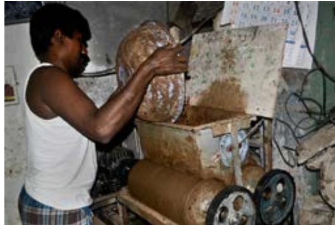
The soaked mixture is put in mixing machine.
