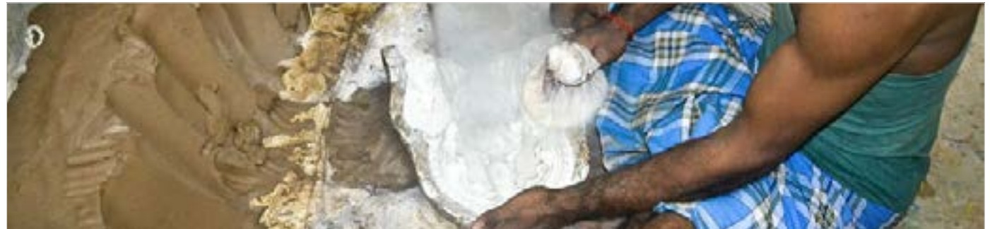
Pop powder is sprinkled on the mould.
