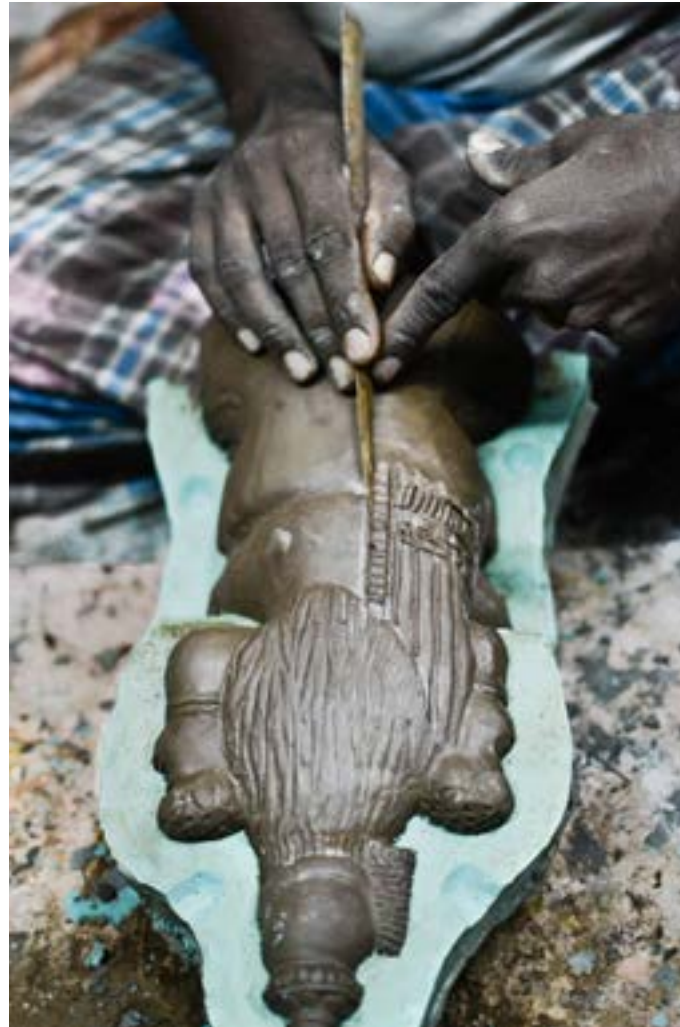
For the other side of the mould, artisan carves the design.
