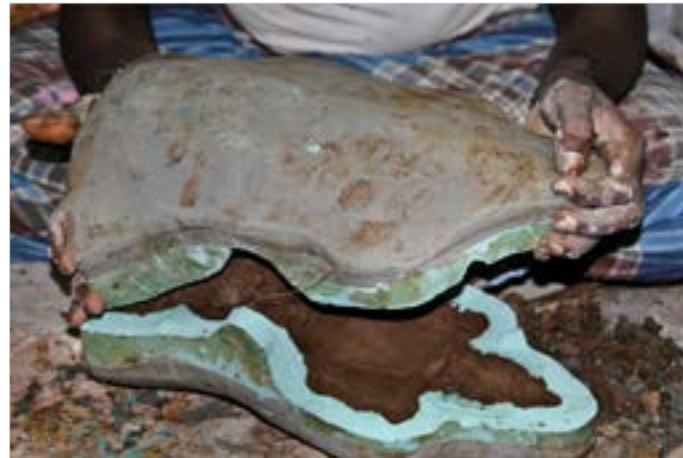
Once the mould is dried it is removed.
