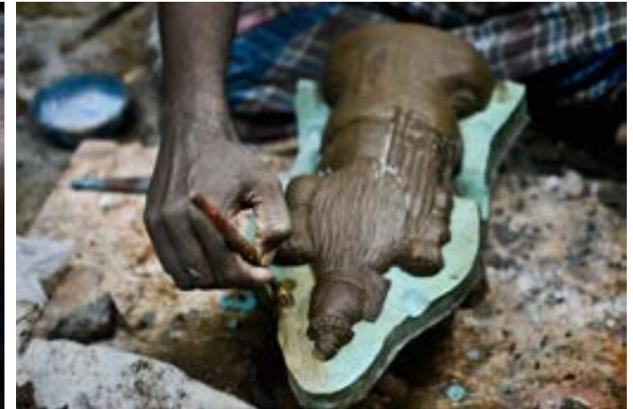
Soap is applied on the sides of the prepared mould to avoid sticking either sides of the mould.
