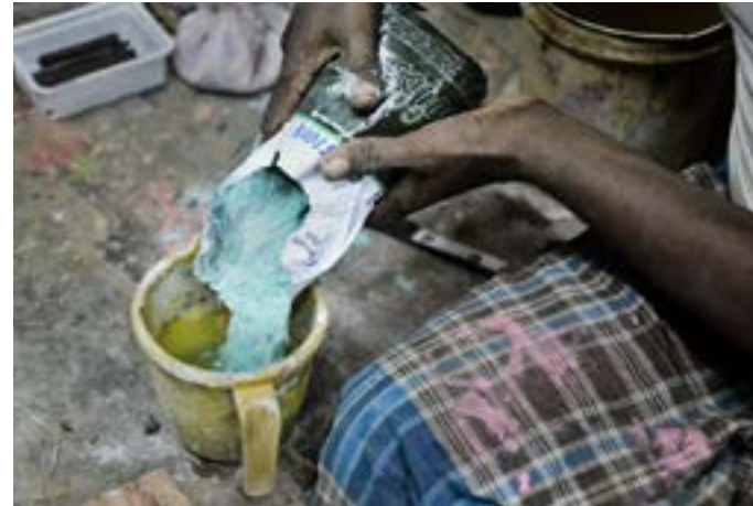
Solution of dental casting powder is prepared for the mould.
