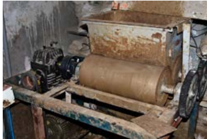
Mixing machine to mix the clay and sand into dough.
