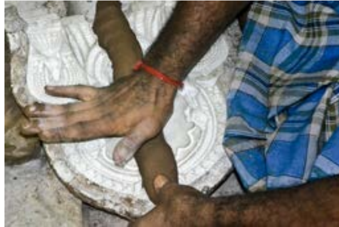
Clay is set in the mould to make the idol.
