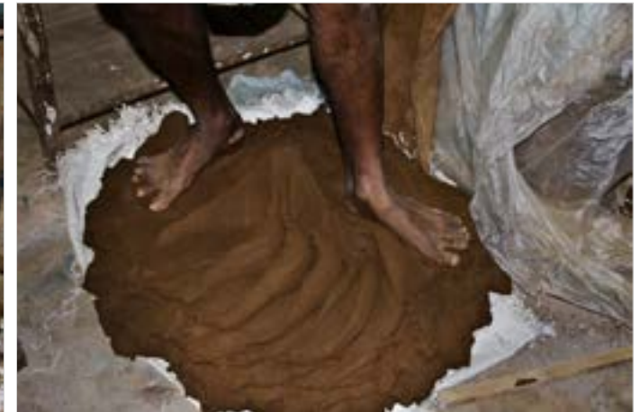
The clay is again kneaded finely with legs to enhance the elasticity of the clay and stored in room temperature.
