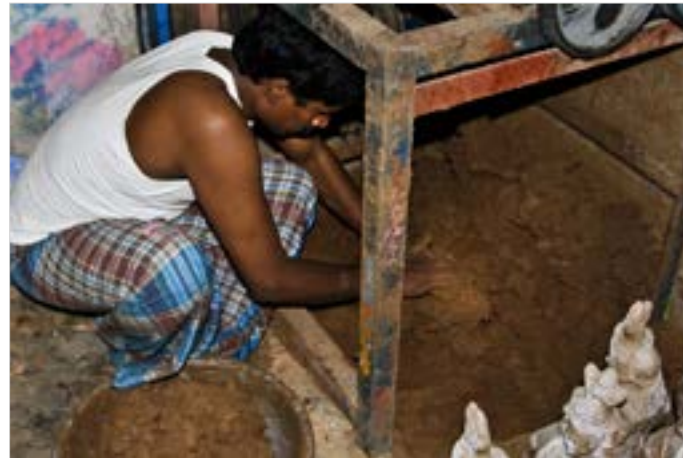
The process is continued three times to enhance the elasticity of the clay.
