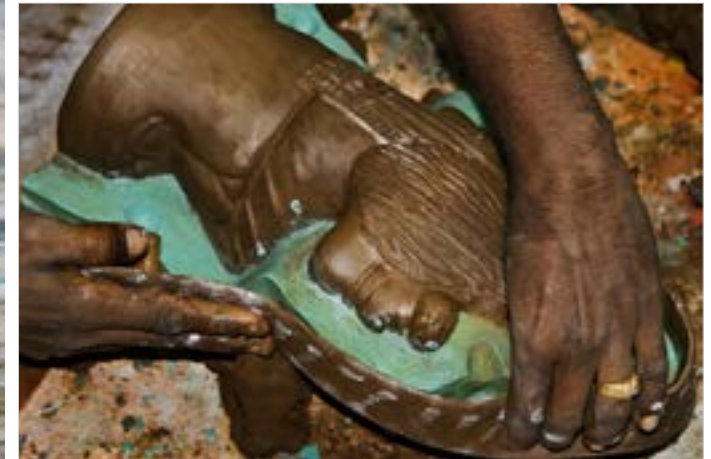
Sidewalls are made and attached to prepare the other half of the mould.
