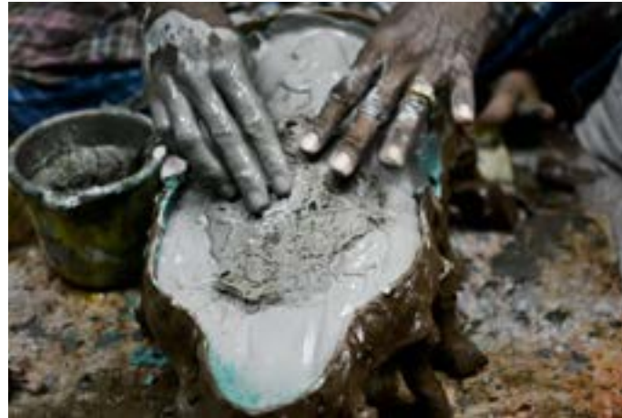
Same process of molding is repeated to prepare the other half of the mould.
