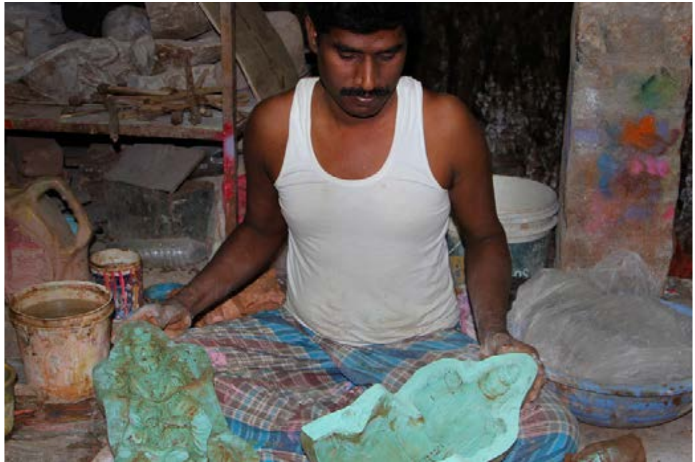
Prepared mould is kept to dry in the room temperature for a week.
