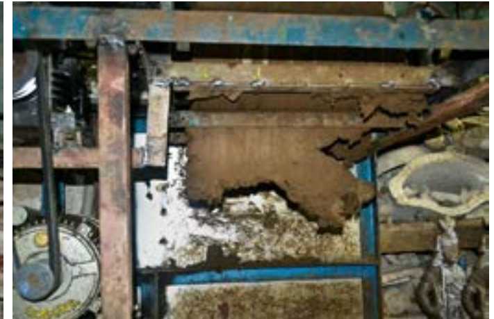
The machine smashes mixture turning it into a soft clay dough.
