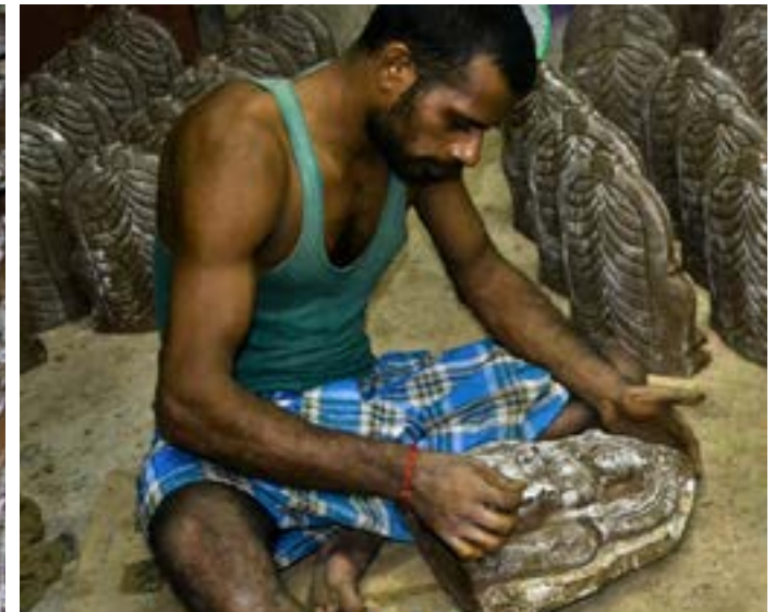
Artisan involved in removing the prepared clay idol from the mould.
